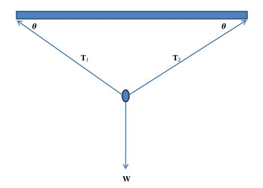
An object in **equilibrium** is suspended from a beam by two ropes, each making an angle of  $\theta$  with the horizontal. The tension forces acting on the object are  $T_1$  and  $T_2$  and W is the weight force. Which one of the following statements is true?
