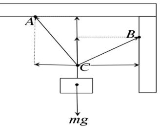
All forces acting on the block and their components in the horizontal and vertical directions are
