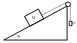
Two particles of different masses M kg and m kg are connected through a light inextensible string over an inclined surface with the friction coefficient  $\mu$ . The angle is  $\alpha$  degrees to the horizontal.
