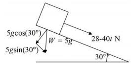
Considering the forces acting parallel to the ramp, the following equation of motion can be found.
