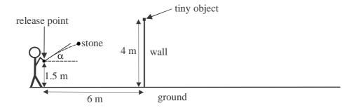
The position vector of the stone at time t seconds,  $t \ge 0$ , relative to the release point is given by  $\mathbf{r}(t) = 15t \cos(\alpha) \mathbf{i} + (15t \sin(\alpha) - 4.9t^2) \mathbf{j}$  where  $\mathbf{i}$  is a unit vector in the horizontal direction of motion and  $\mathbf{j}$  is a unit vector vertically upwards. Displacement is measured in metres.
