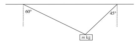
The longer string makes an angle of  $60^{\circ}$  with the vertical and has tension of  $\sqrt{6}$  newtons. The shorter string makes an angle of  $45^{\circ}$  with the vertical.
