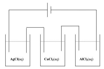
As the cells are connected in series, the same number of mole of electrons passes through each cell. The metals have different oxidation states, so the number of mole of metal obtained will differ.
