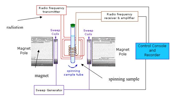
Sample is – placed in a magnetic field, where the intensity of the field is varied.
