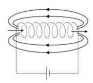
The current is up the left hand wire, so it goes down at the front of the solenoid
