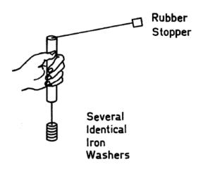
A rubber stopper of mass m is whirled in a horizontal circle of radius r. An experiment is performed to investigate the relationship between m, r, the speed of the stopper v, and the centripetal force, F, acting on the stopper.
