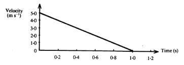
The graph above gives the velocity-time relationship for a block of mass 4.0 kg which slides across a rough, horizontal floor, coming to rest after 1.0 s.
