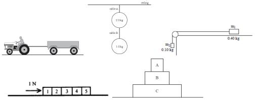
Problems involving the motion of two bodies connected by strings are solved on the following assumptions: the string is assumed light and inextensible so its weight can be neglected and there is no change in length as the tension varies. Tension forces are pulls exerted by a string on the bodies to which it is attached.
