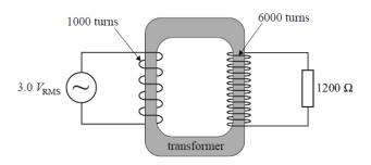
The primary coil has 1000 turns; the secondary coil has 6000 turns. There is a 1200  $\Omega$  resistor in the secondary circuit. A 3.0  $V_{\text{RMS}}$  AC power supply is connected across the primary coil.
