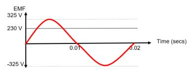
The peak to peak voltage is from +325 to – 325. The peak voltage is 325 V. The Root Mean Square (RMS) voltage is the square root of the mean of the square of the potential difference.
