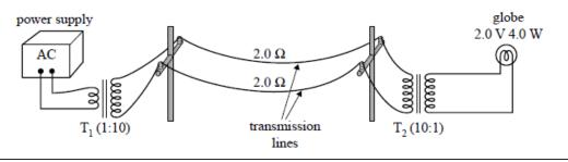
The step up transformer is always at the supply end. Stepping up the voltage, reduces the current in the transmission lines for the same power being supplied. The decrease in current leads to less power loss in the transmission lines, which leads to more power at the output. The step down transformer at the output, brings the voltage down to manageable levels.
