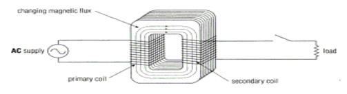
In an ideal transformer the total transfer of magnetic flux is assumed,  $\therefore$  energy (power) is conserved. Input power = Output power  $P_{in} = P_{out}$
