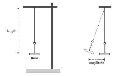
The students use a constant mass and a constant amplitude of swing, changing only the length of the pendulum and then measuring the time for five oscillations. They obtain four different time readings for four different lengths of the pendulum.
