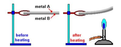
Different metals expand different amounts for the same temperature rise. A bimetallic strip is made from two different metals joined together. The effect of heating a bimetallic strip is shown in the diagram. Which pair of metals could be used in the experiment to make the strip bend downwards?
