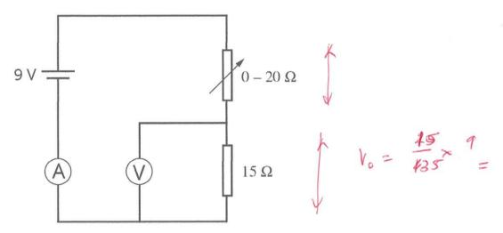
a What is the possible range of readings on the ammeter?
