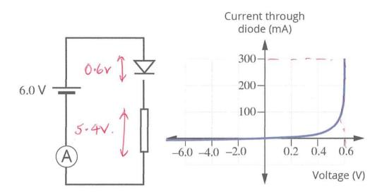
**a** If the current in the circuit is 300 mA, what is the resistance value of the fixed resistor?
