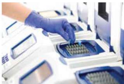
Figure 3 Photograph of a PCR cyclor machine
