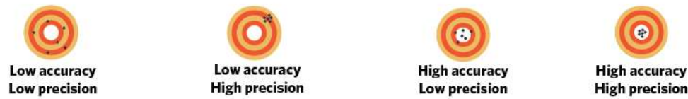
Figure 2 Accurate results are close to the true value whereas precise results have very little spread around the mean value.
