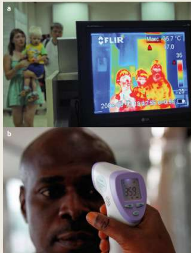
FIGURE 5.3.4 (a) Thermal scanning cameras are used to monitor the skin temperature of passengers arriving at airports. Raised skin temperature can be an indicator of fever from illnesses such as influenza and Ebola. Such cameras have been used widely to screen for carriers of various epidemic influenzas, such as bird flu and swine flu, to prevent the global spread of the viruses. (b) Teams in airports around the world were equipped with thermal guns to measure the temperatures of travellers from Liberia, Sierra Leone and Guinea in an effort to prevent an Ebola pandemic in 2014.
