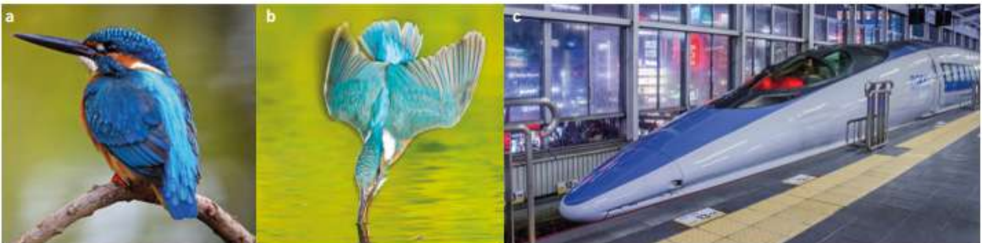
FIGURE 5.1.37 (a,b) A kingfisher's long, streamlined beak allows it to dive for fish without creating a splash. (c) The Shinkansen bullet train's nose shape is modelled on the kingfisher's beak. The streamlined shape solved the problem of sonic booms when the train travels through tunnels at high speed.
