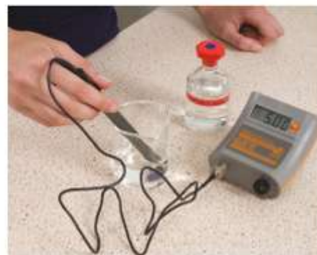
FIGURE 1.5.4 Measuring the pH level of tartaric acid with a pH meter. To ensure an accurate reading, the student would first have calibrated the meter using a solution of known pH.
