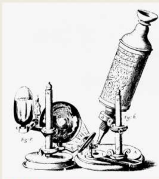
FIGURE 2.1.1 Robert Hooke's drawing of his light microscope in Micrographia , published in 1665.
