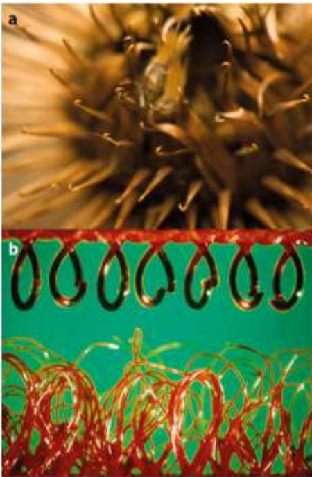
FIGURE 5.1.36 (a) A magnified view of a burdock ( Arctium lappa ) seed. (b) A magnified image of Velcro, showing the separated hooks and loops.
