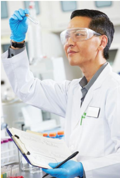
FIGURE 1.2.4 A lab coat, gloves and safety glasses are essential items of personal protective equipment in the laboratory.
