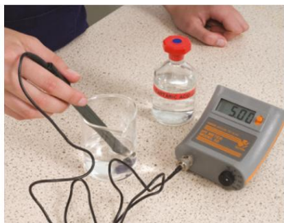
FIGURE 1.4.6 Measuring the pH level of tartaric acid with a pH meter. To ensure an accurate reading, the student would first have calibrated the meter using standard solutions of known pH.
