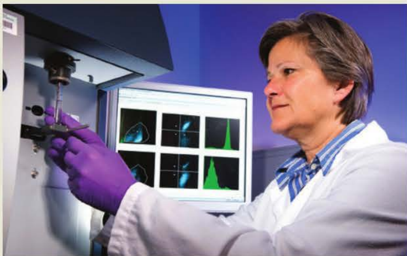
FIGURE 1.3.4 A scientist analyses cells with a flow cytometer. Cells are tagged with a fluorescent marker, sorted in the flow cytometer and visualised on a computer screen.
