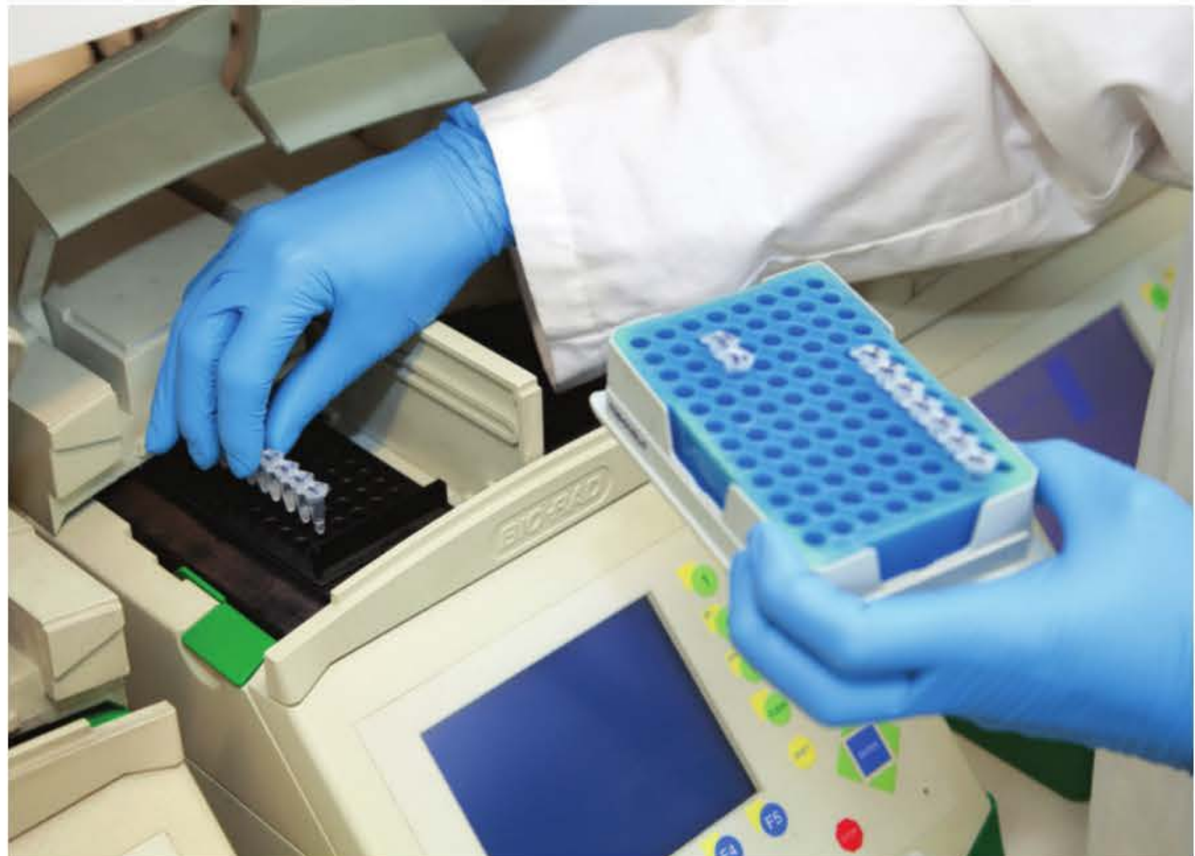
FIGURE 4.1.3 A scientist loads DNA samples into a thermocycler to be amplified by PCR.
