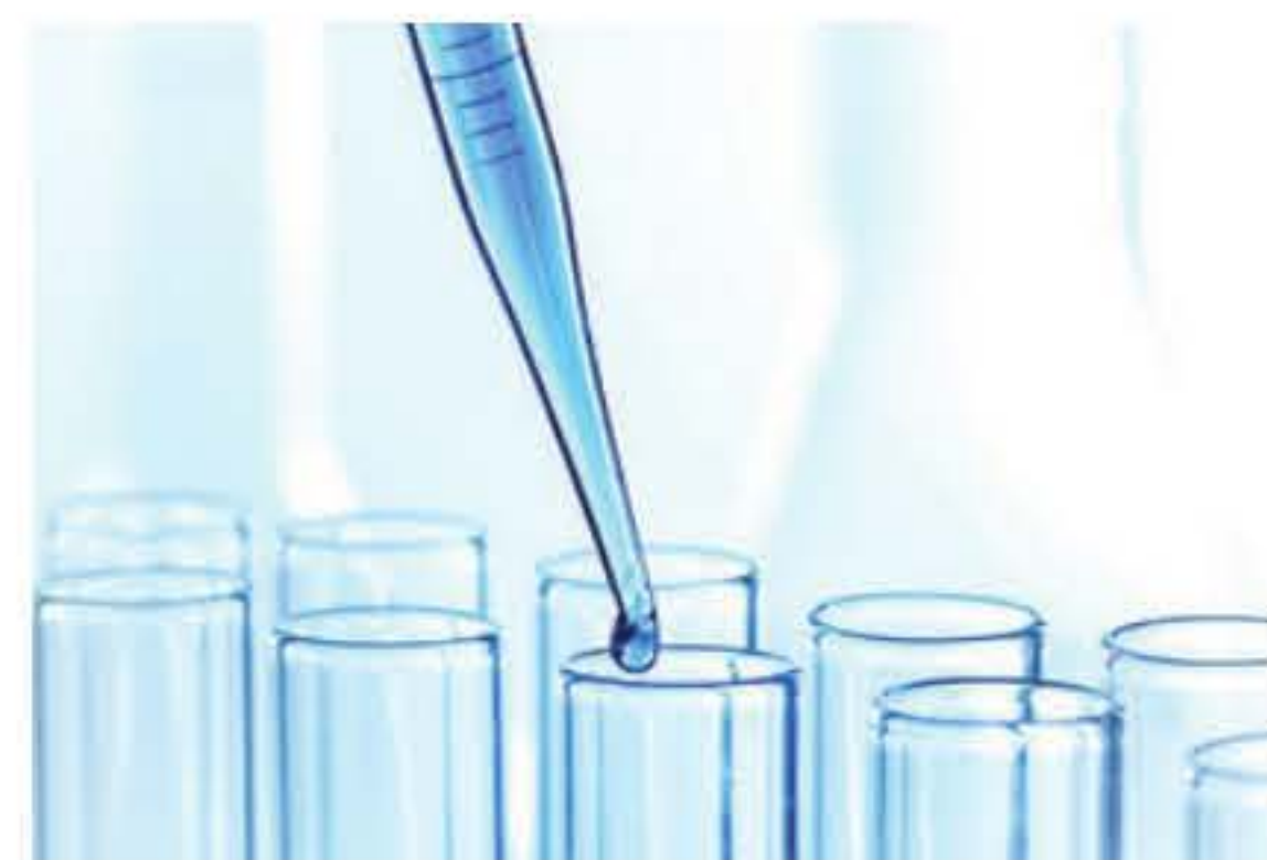
FIGURE 1.4.8 A 5 mL graduated pipette can measure volumes to an accuracy of one hundredth of a millilitre, or 5 \text{ mL} \pm 0.01 \text{ mL} . The pipette has major divisions of 1 mL and minor divisions of 0.1 mL. You can estimate to 0.01 mL and record volumes to 2 decimal places, for example 3.80 mL or 4.52 mL.
