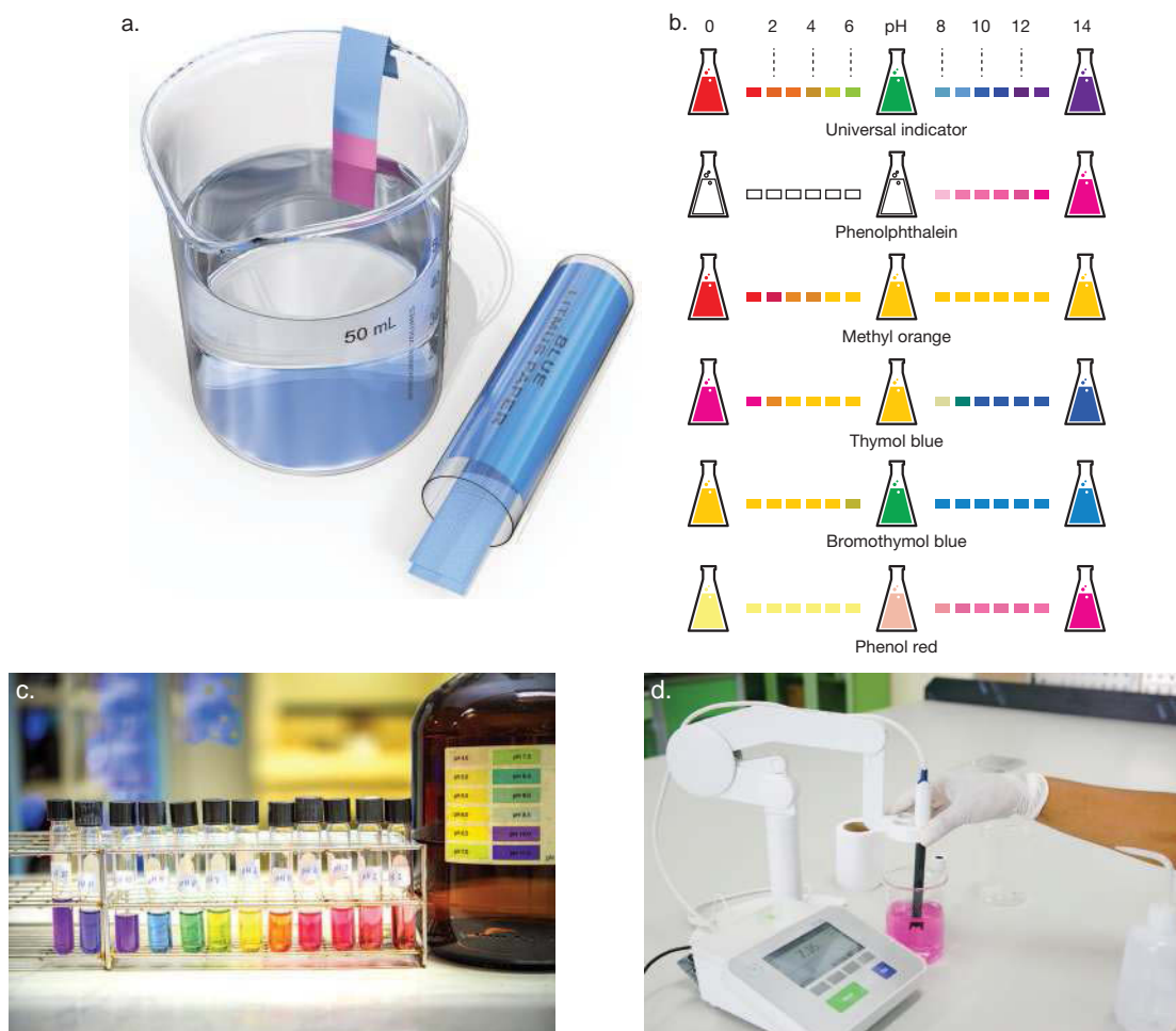
FIGURE 5.26 a. Litmus paper, changes red in acids and blue in bases b. Different indicators that can be used to determine pH c. Universal indicator d. pH meter
