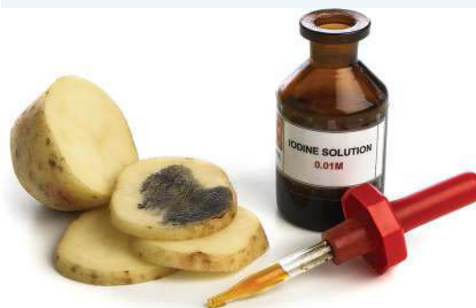
FIGURE 5.36 When iodine reacts with the starch in potato, a blue-black colour is seen. Using cubes of potato is often used to explore surface area to volume ratio.
