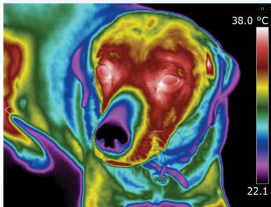
FIGURE 4.27 Heat signature of Lettie, a Labrador dog, obtained with an infra-red camera that detects surface temperatures
