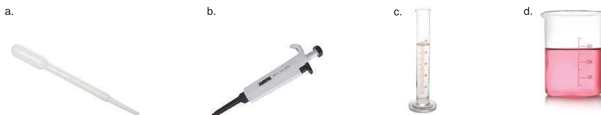
FIGURE 5.23 Equipment used to measure volumes: a. micropipette b. pipette c. measuring cylinder d. beaker
