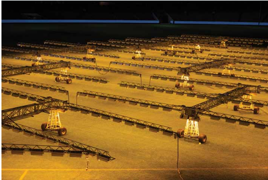
FIGURE 4.28 Artificial lighting is used to illuminate the grass surface of a soccer field at night.
