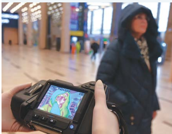
FIGURE 6.1 Airport screening for the 2020 COVID-19 coronavirus outbreak. Thermal imagery is being used to check for signs of fever.
