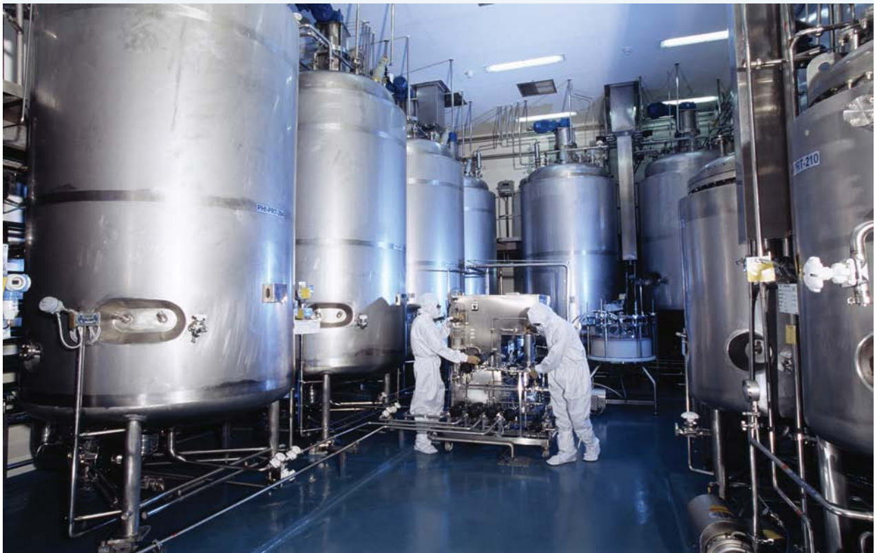
FIGURE 2.42 Stainless steel fermentation vats in which mass culturing of recombinant E. coli bacterial cells takes place and where those cells express the insulin gene
