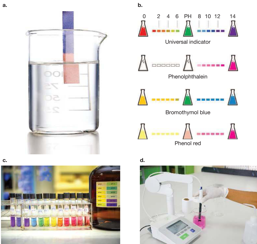
FIGURE 11.17 a. Litmus paper, changes red in acids and blue in bases b. Different indicators that can be used to determine pH c. Universal indicator d. pH meter
