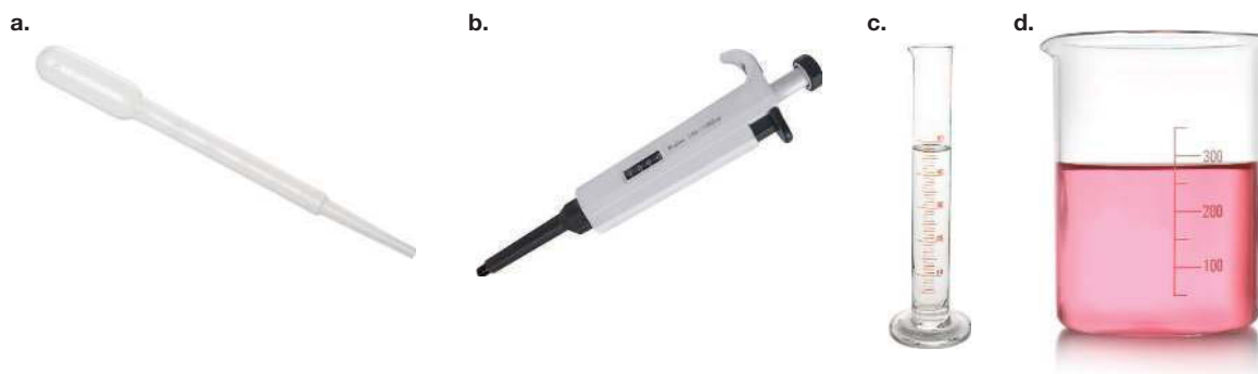
FIGURE 11.13 Various equipment used to measure volumes: a. pipette, b. micropipette, c. measuring cylinder and d. beaker
