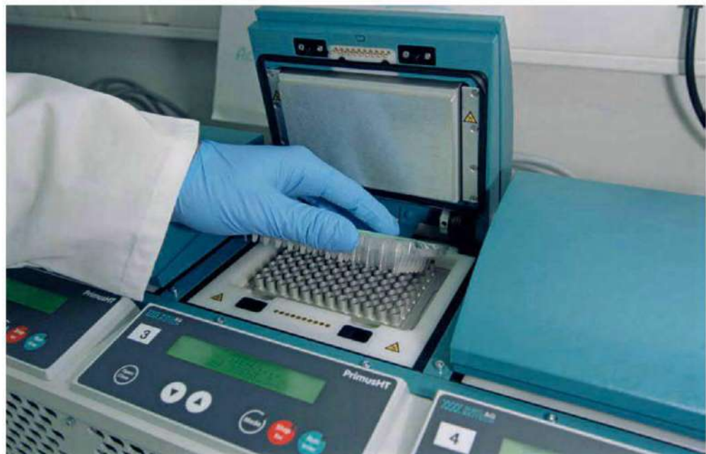
Figure 5.5 ▶ Thermal cyclers, in which the PCR is carried out as an automated process
