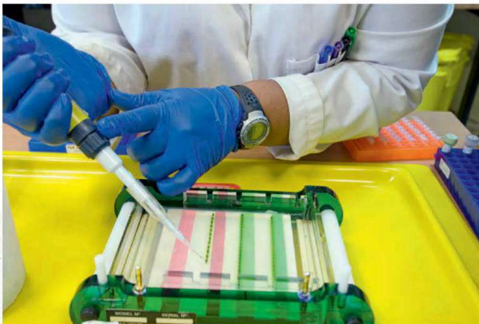
◀ Figure 5.6 A researcher injecting genetic material from coral into an agarose electrophoresis gel apparatus
