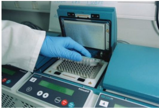
Figure 3.13 A thermal cycler, in which the PCR is carried out as a programmable automated process. The thermal cycler raises and lowers the temperature of the samples, which allows denaturation, annealing and extension to take place in a controlled way.
