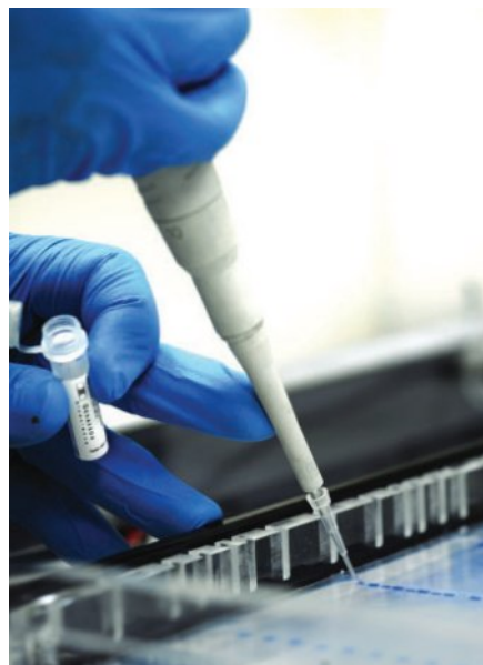
Figure 3.14 A researcher loads genetic material from coral into an agarose electrophoresis gel apparatus.
