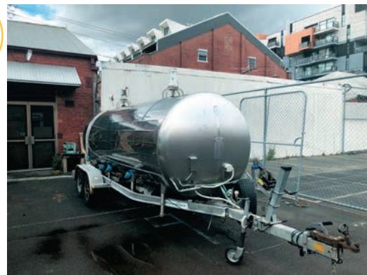
Figure 5.27 The portable bioreactor at the Ecological Justice Hub in Brunswick produces electricity from biomass waste products, supplying electricity without the use of fossil fuels.
