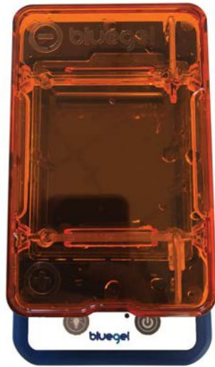
FIGURE 3 A gel electrophoresis box separates strands of DNA based on size. The negatively charged DNA travels towards the positive end of the gel.
