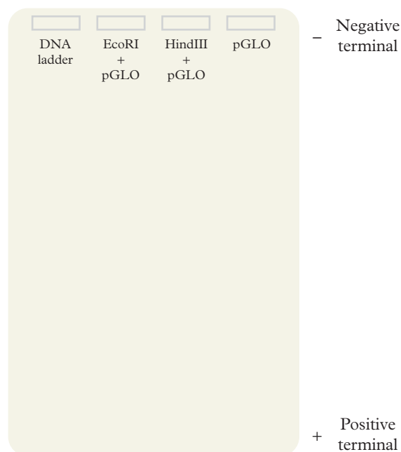
FIGURE 2 An example of an agarose gel with samples loaded in the wells at the top of the gel prior to electrophoresis. Note that the negative and positive terminals have been labelled.
