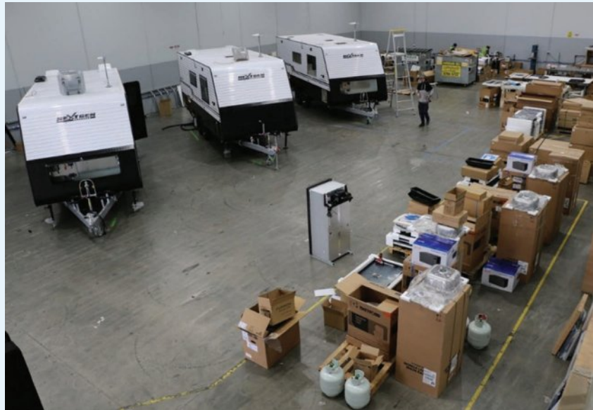
Figure 8.19 Network RV employs a cellular production method to efficiently construct caravans.
