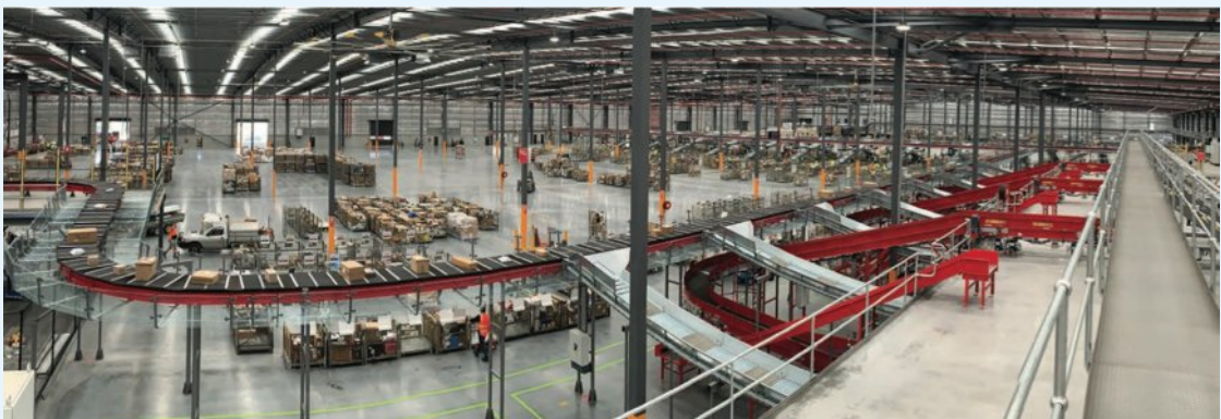
Figure 15.5 The new Victorian parcel distribution centre at Sunshine West integrates the latest in automated sorting technology and remained fully operational 24 hours a day to cope with demand during the COVID-19 pandemic.
