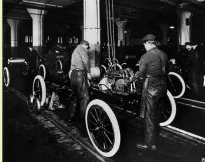
Workers constructing a Model-T car on an assembly line in a Ford Motor Company factory, circa 1914.
