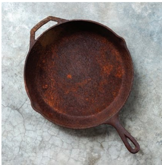
Figure 3B–6 The flaky red-brown coating on this iron frying pan is rust.
