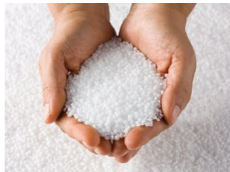
Figure 7A–5 Plastic resin made from materials from crude oil. This resin can be moulded into many of the plastic items we use daily.
