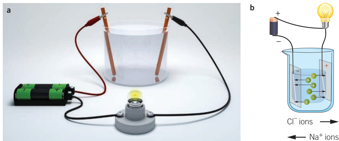
Figure 14A–6 A simple circuit showing how salt water can successfully conduct electricity; a ) The brighter the bulb, the greater the conductivity of the solution, and hence the higher the level of dissolved salt. b ) An ionic solution will conduct an electric current as positive ions move towards the negatively charged electrode and negative ions move towards the positively charged electrode.
