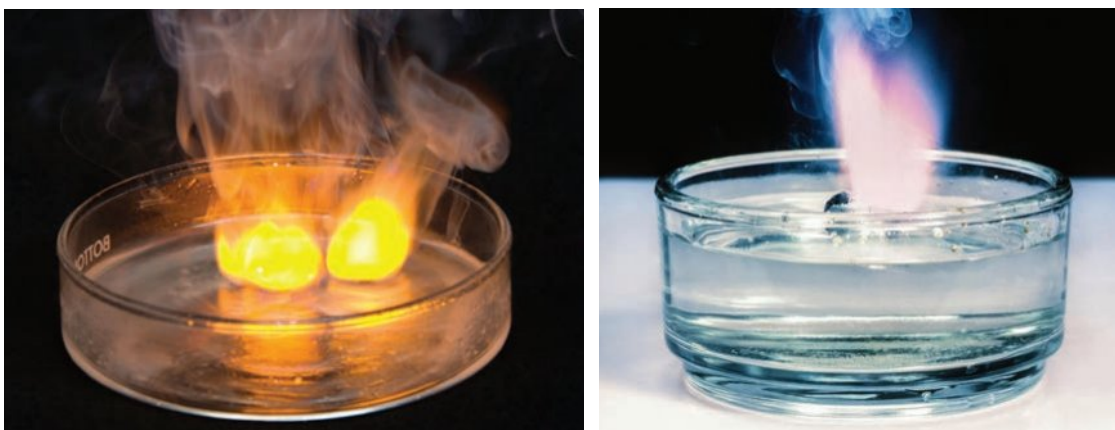
Figure 1C-8 Group 1 metals, such as sodium (left) and potassium (right), reacting with water
