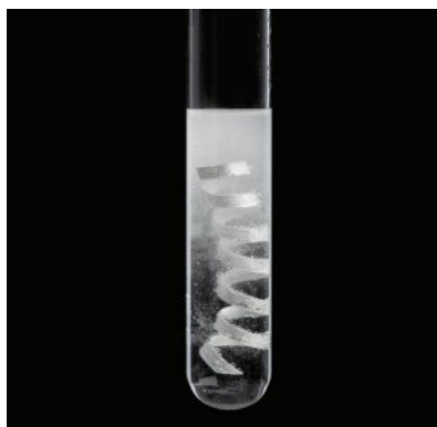
Figure 11E–3 Metals reacting with an acid. Bubbles of hydrogen gas can be seen forming on the surface of the metal.
