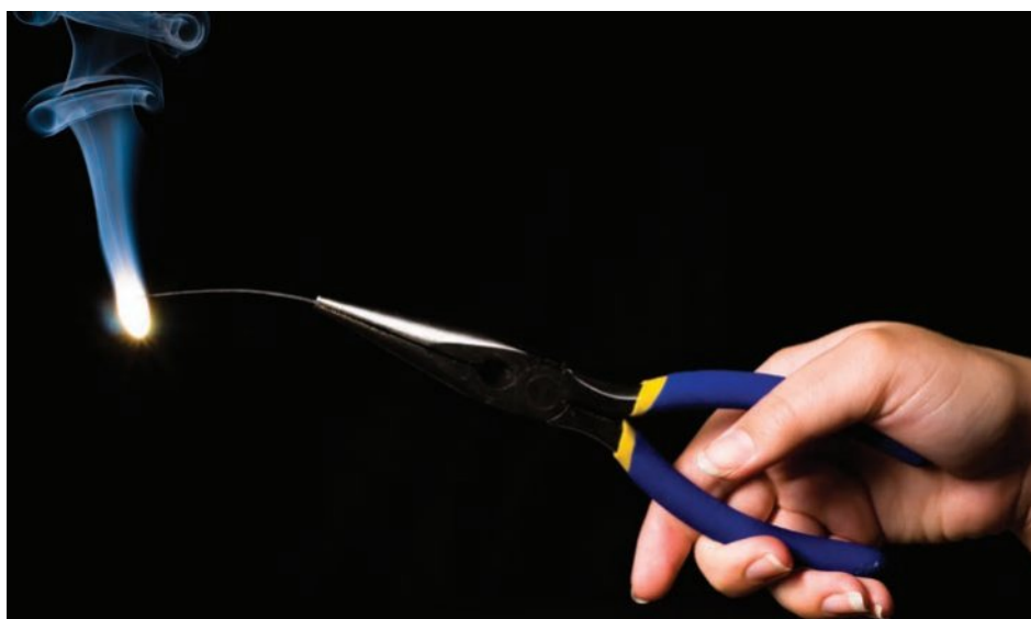
Figure 12A–2 In this redox reaction, magnesium ribbon burns in the presence of oxygen to produce a bright white flame.
