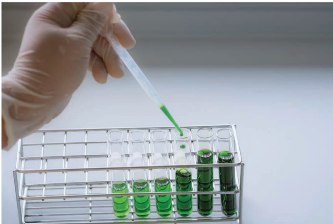
Figure 14C–2 The concentration of this green-coloured solution increases from left to right, as seen by the increase in darkness of the solution.
