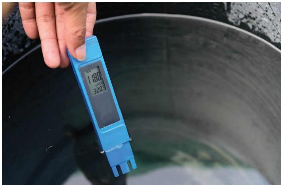
Figure 14A-8 Testing a water sample with portable digital probe. This will provide a numerical, or quantitative, reading of temperature, pH and electrical conductivity.
