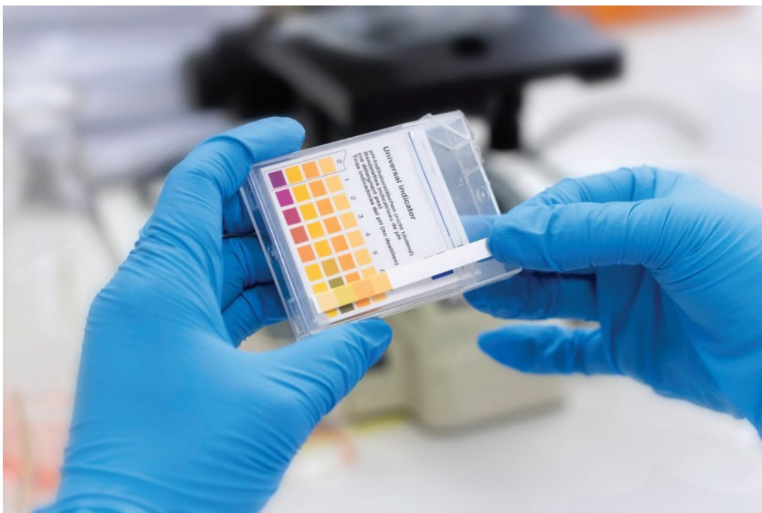
Figure 11C–4 Universal indicator paper contains a mixture of indicators: it uses a qualitative approach, changing colour in solution to indicate approximate pH. Using a scale, this can be translated into a quantitative pH number for the solution.
