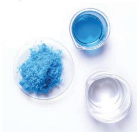
Figure 14B–3 Blue copper sulfate, \text{CuSO}_4 \cdot 5\text{H}_2\text{O} crystals, are an example of a hydrated salt.
