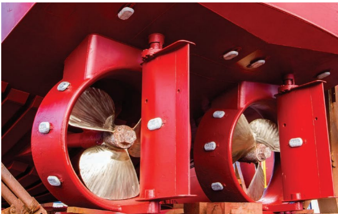
Figure 12D–3 Sacrificial anodes (the white blocks) are placed around a ship's motor to protect it against corrosion.
