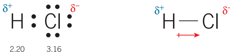
Figure 2B–4 Lewis structure and structural formula for hydrogen chloride, showing a polar bond and permanent dipoles in the molecule
