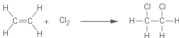
Figure 7B–10 Addition reaction between ethene and chlorine gas, resulting in the production of a haloalkane.
