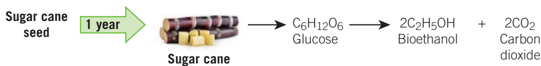
Figure 9C-4 Production of bioethanol from sugar cane, a renewable feedstock
