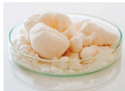
Figure 2B–4 Potassium chloride is a common staple of laboratories that conduct a lot of solution calorimetry experiments as it is a widely available, cheap and well-studied compound.
