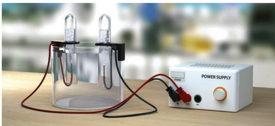
Figure 3C–5 An electrochemical cell showing a set-up with two gas electrodes
