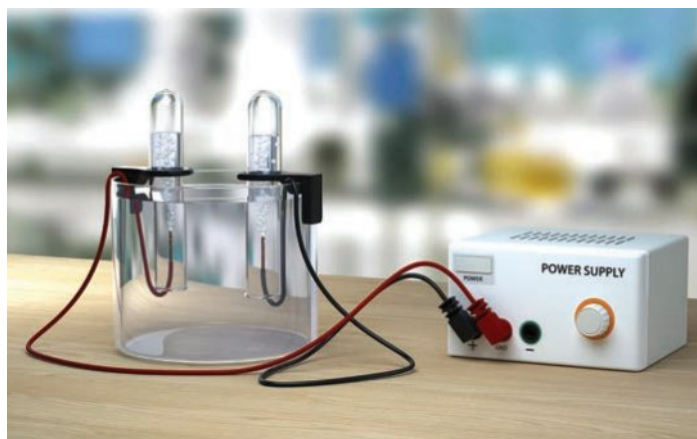
Figure 7C–5 Electrolysis of water into hydrogen and oxygen gas. In the schematic, a universal indicator has been added that turns red in the acidic environment generated around the anode and blue in the alkaline environment generated around the cathode.
