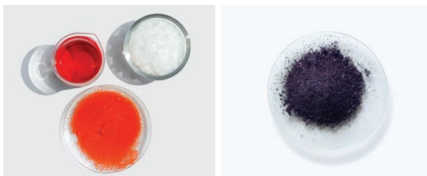
Figure 9A–20 Samples of \text{K}_2\text{Cr}_2\text{O}_7 (left) and \text{KMnO}_4 (right) are strong oxidising agents used to oxidise primary alcohols to carboxylic acids.
