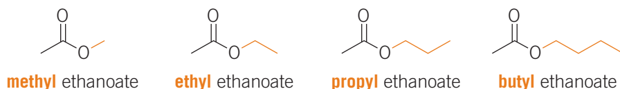
Figure 8D–16 The first word in the name of an ester describes the alcohol part of the structure.
