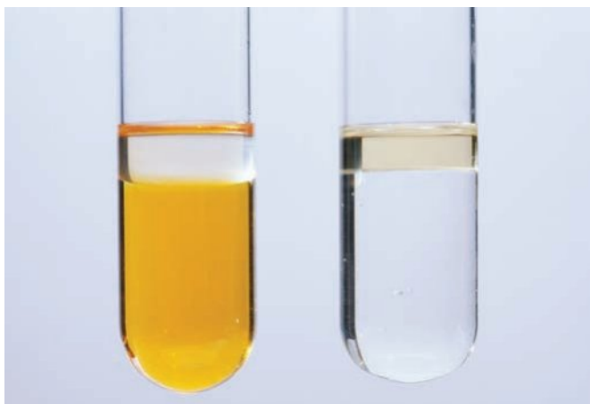
Figure 10A-4 When a reaction takes place, the bromine solution changes from a yellow-orange colour (left) to colourless (right). This forms the basis of the bromine test.
