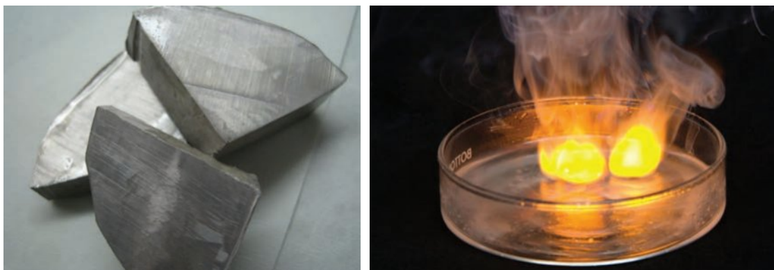
Figure 5B–4 Solid sodium (left) is safe to have in the open as the surface area that can react with the atmosphere is a small proportion of the volume of the object, and thus the reaction rate is low. Powdered sodium (right), however, is made of many small particles, all of which can react with the atmosphere. Therefore, the reaction rate is fast (and the reaction is violent!).
