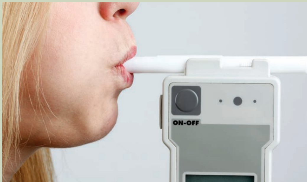
Figure 11B–1 In a breathalyser (or breath analyser), breath is blown into the sample chamber and analysed by a beam of infrared radiation to detect the concentration of alcohol in your blood.
