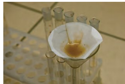
Figure 1 Simple filtration of a soil sample dissolved in water
