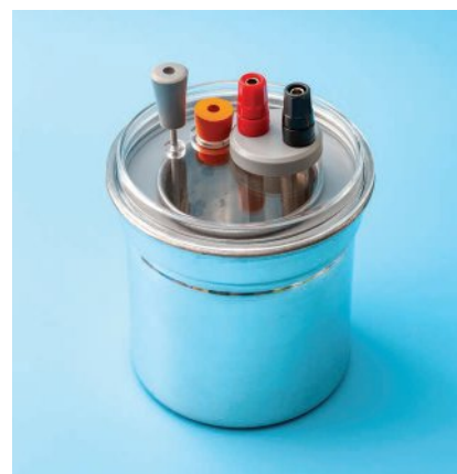
Figure 2 Calorimeter used to measure enthalpy of a combustion reaction
