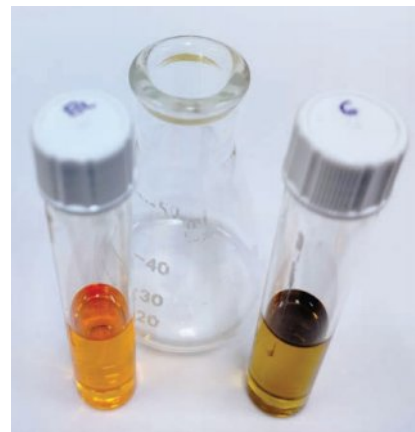
Figure 5 Using potassium dichromate a primary or secondary alcohol can be oxidised, turning from orange to green.
