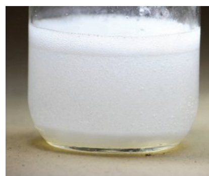
Figure 9 Carboxylic acids readily effervesce with sodium carbonate.
