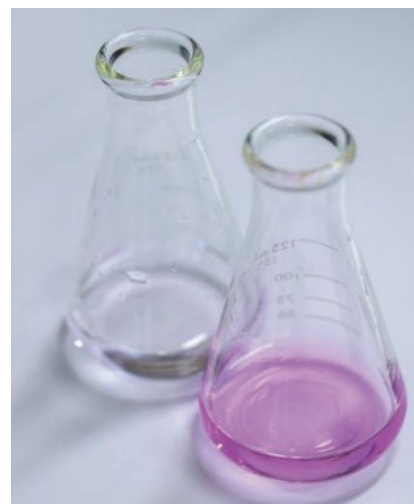
Figure 8 Phenolphthalein changes from pink to colourless when an acid is added.
