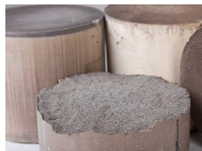
Figure 4 The honeycomb structure of a catalytic converter can have a surface area of up to 500 m 2 .
