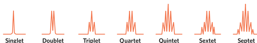
Figure 5 Splitting patterns in high resolution proton NMR spectra
