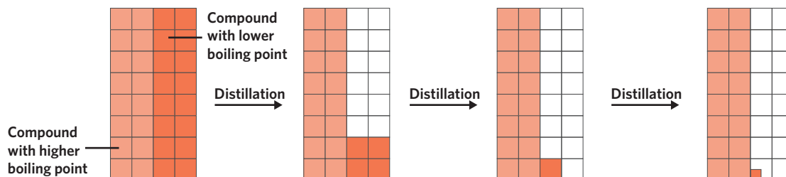
Figure 8 Representation of distillation, where three quarters of the remaining undesired compound is distilled at each stage
