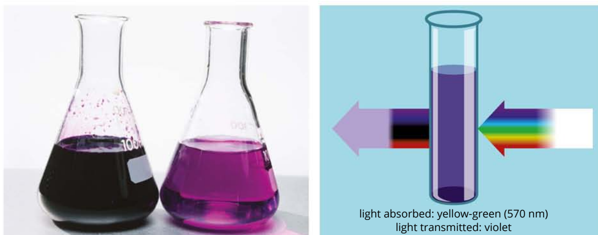
FIGURE 18.4.2 Two solutions of potassium permanganate ( \text{KMnO}_4 ) appear purple because they absorb yellow-green light. The 0.001 M solution is lighter in colour than the 0.01 M solution because it absorbs less light.
