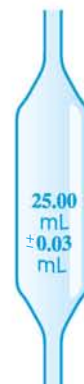
FIGURE 21.2.6 Record the uncertainty for glassware and instruments in your logbook. This pipette can dispense an aliquot of 25.00 mL \pm 0.03 mL.
