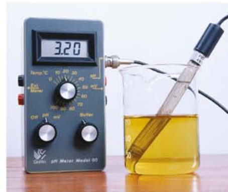
FIGURE 15.3.2 A pH meter is used to measure the acidity of a solution.
