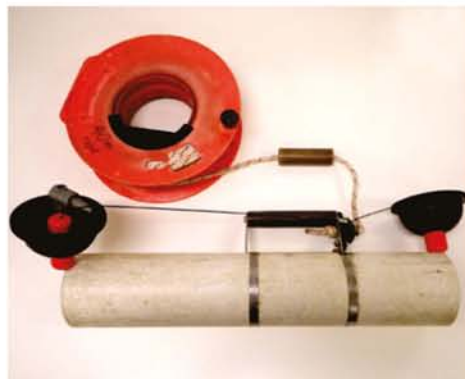
FIGURE 17.2.5 A Van Dorn sampler consists of a polymer tube with caps at each end.
