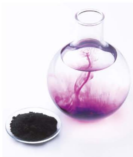
FIGURE 13.1.1 When solid potassium permanganate is added to water, it dissolves. The particles disperse into the solution and move around freely.
