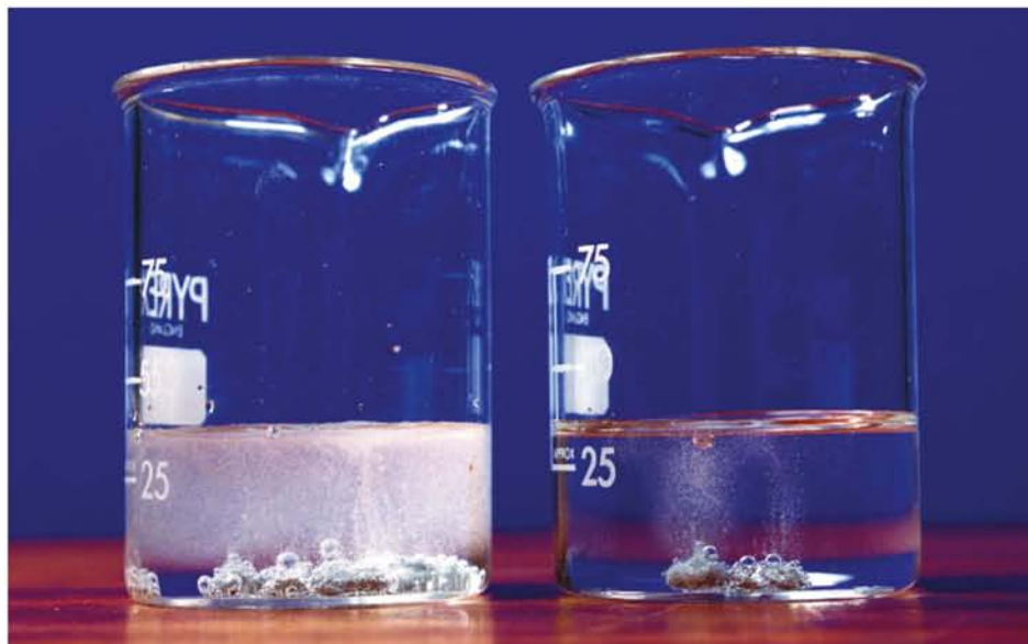
FIGURE 15.2.1 Zinc reacts more vigorously with a strong acid (left) than with a weak acid (right). The acid solutions are of equal concentration and volume.
