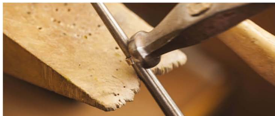
FIGURE 3.5.6 The crystal structure of metals like this gold ring can be altered by work hardening. Care is needed as the gold becomes more brittle through this process.
