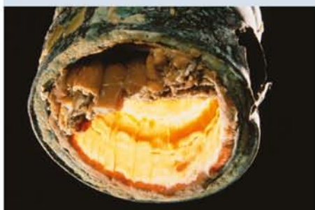
FIGURE 13.4.6 Accumulation of limescale in pipes is a result of precipitation of \text{CaCO}_3 .
