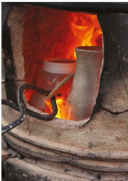
FIGURE 4.2.1 Bricks made from the ionic compound magnesium oxide are used to line furnaces and kilns.
