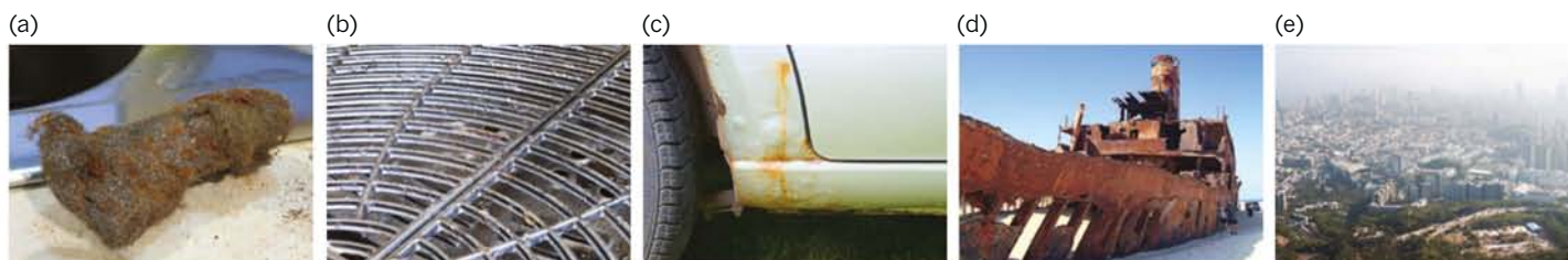
FIGURE 16.3.3 Wet corrosion. (a) A piece of steel wool (iron) does not corrode on supermarket shelves. However, once it becomes wet through use, it corrodes quickly. (b) An iron barbecue grill that has been coated with grease shows little sign of corrosion, even after being exposed to the rain for some time. (c) Rust in a car generally starts inside door frames, under mudguards, or in places where the paint has been chipped. (d) Shipwrecks corrode rapidly and will eventually disintegrate. (e) Corrosion occurs more rapidly in cities with a pollution problem, particularly where the pollutants include acidic oxides such as nitrogen dioxide and sulfur dioxide.
