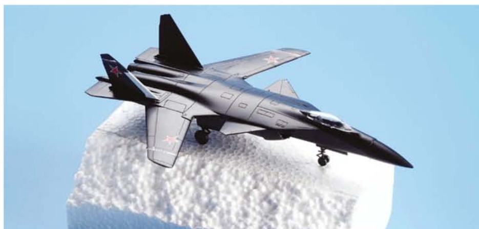
FIGURE 10.2.21 A model plane made of rigid polystyrene sitting on a block of foamed polystyrene.
