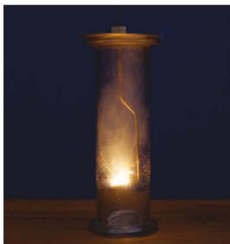
FIGURE 3.3.4 Sodium burning in pure oxygen.
