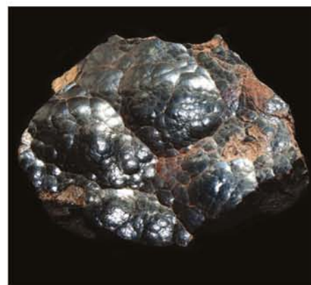
FIGURE 3.4.2 The mineral haematite ( \text{Fe}_2\text{O}_3 ) is mined as the main source of iron. This sample has been partially polished, removing most of the red oxide coating that forms upon exposure to air.
