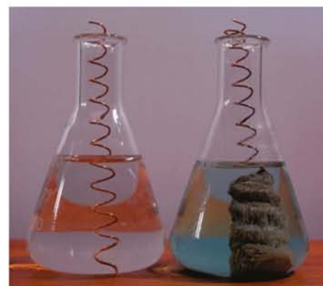
FIGURE 16.2.5 When a strip of copper wire is suspended in a solution of silver nitrate in the flask on the left, long crystals of silver metal start to form. In the flask on the right, the copper has displaced the silver from the solution.
