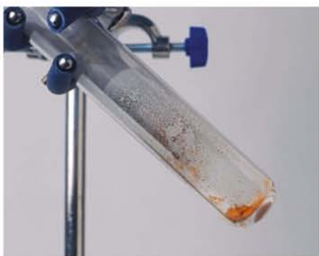
FIGURE 1.2.5 The red powder in this test-tube is mercury(II) oxide ( \text{HgO} ). If you look closely at the test-tube, you will see beads of liquid mercury forming from the decomposition of the compound.
