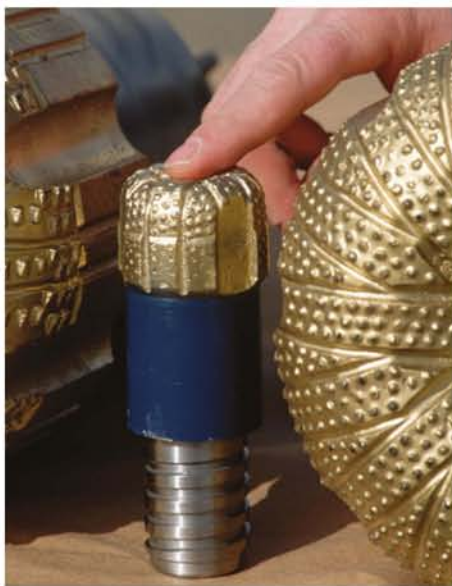
FIGURE 8.1.5 Diamond-tipped drills used to drill through rock in the fracking industry.
