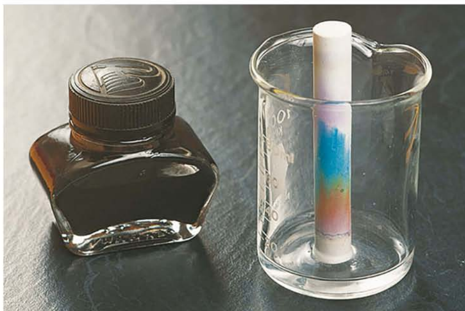
FIGURE 19.2.1 The pattern of bands produced when this stick of chalk is dipped in black ink and then placed in water is called a chromatogram.
