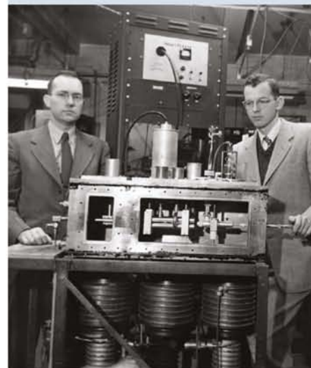
FIGURE 7.1.5 Charles Hard Townes and James Power Gordon invented the first maser using ammonia gas.
