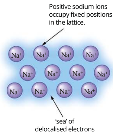
FIGURE 3.2.2 A representation of a sodium metal lattice. Each sodium atom loses its one valence electron. This electron is shared with all atoms in the lattice to form a sea of delocalised electrons.
