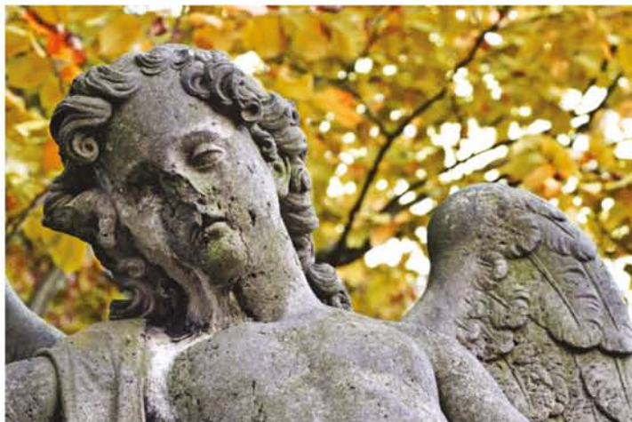
FIGURE 15.5.4 This statue has been heavily eroded by acid rain, which reacts with carbonate salts in limestone. Acid rain is formed when gases, such as sulfur dioxide and nitrogen oxides, dissolve in water to form acidic solutions.
