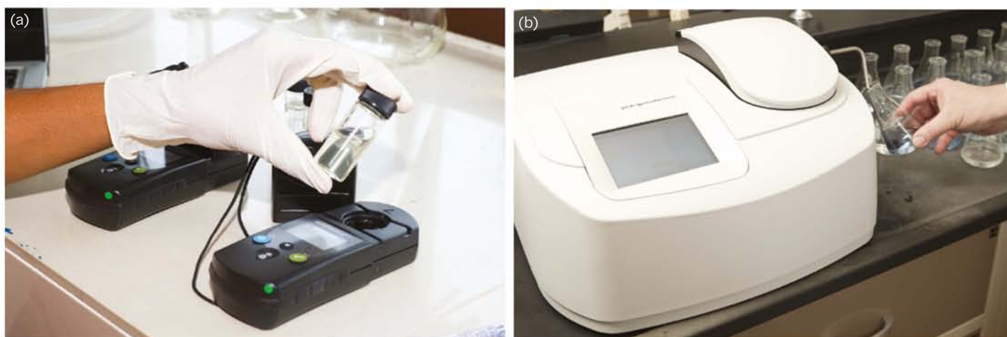
FIGURE 18.4.9 (a) A portable colorimeter. A solution sample is inserted into this unit in a small plastic cell. (b) A laboratory UV–visible spectrophotometer.
