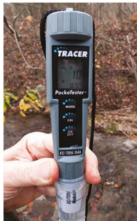
FIGURE 18.1.14 Portable digital salinity meters such as this one usually self-adjust for temperatures other than 25^\circ\text{C} .
