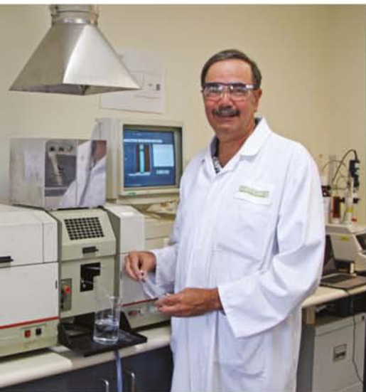
FIGURE 18.5.13 An analytical chemist uses AAS to determine the concentration of metals in food samples.
