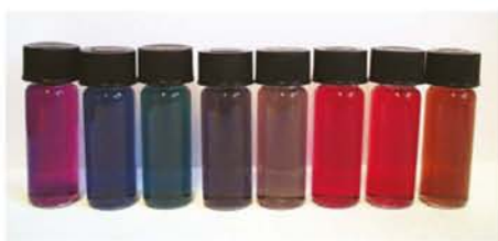
FIGURE 1.1.10 These vials contain gold particles of various sizes. The different-sized particles are different colours because they interact with light differently.
