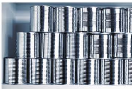
FIGURE 3.5.9 'Tin' cans constructed from steel with a thin coating of tin make the can resistant to rusting.
