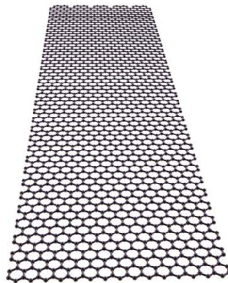
FIGURE 8.2.5 Graphene is a single layer sheet with the same arrangement as those stacked in graphite.
