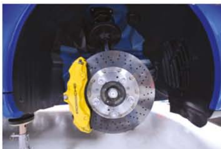
FIGURE 4.2.2 Ceramic brake discs work more effectively than steel ones at high temperatures. A ceramic brake disc contains ionic compounds that have very high melting temperatures and withstand the heat produced by braking better than metals.
