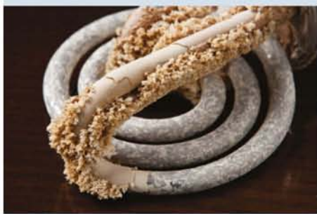
FIGURE 13.4.5 The accumulation of limescale on domestic kettles is the result of precipitation of calcium carbonate as water is repeatedly boiled.
