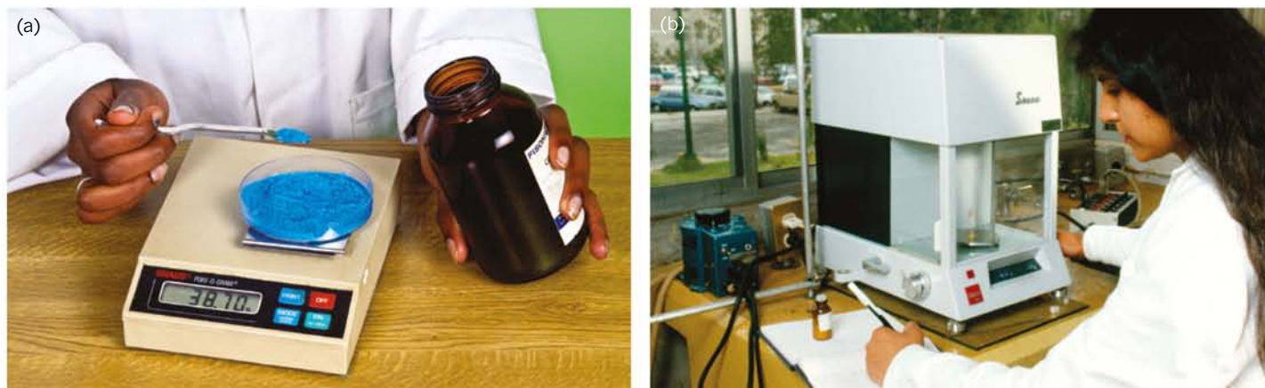
FIGURE 20.2.2 (a) A top-loading balance and (b) an analytical balance can be used to accurately weigh substances used in chemical analysis.
