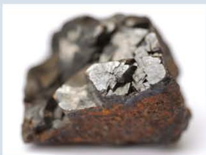
FIGURE 5.4.3 Elemental analysis of the mineral magnetite has allowed chemists to determine the percentage composition to be 72.4% iron and 27.6% oxygen.
