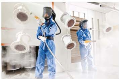
FIGURE 3.5.10 Powder coating uses fine particles of pigment and resin to protect the metal underneath.
