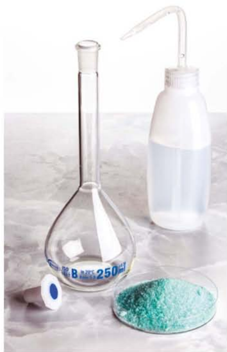
FIGURE 20.2.1 Apparatus and materials needed to prepare a standard solution. The measured mass of solid will be dissolved in water in a volumetric flask to make an accurate volume of solution.
