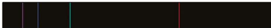
FIGURE 1.5.8 The emission spectrum of the hydrogen atom has four lines in the visible range—violet, blue, green and red.
