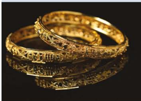
FIGURE 3.5.4 Gold jewellery is typically made from alloys. Pure gold (24-carat purity) is not often used for jewellery because it is too soft.
