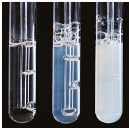
FIGURE 15.5.7 Limewater test. Carbon dioxide is bubbled through limewater, turning the limewater cloudy.
