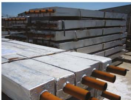
FIGURE 16.3.8 These aluminium sacrificial anodes are attached to the underwater steel structures of offshore gas platforms to protect them against corrosion.
