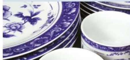
FIGURE 4.2.6 Porcelain cups and plates are made from clay, which contains ionic compounds. Therefore, porcelain is hard and brittle.
