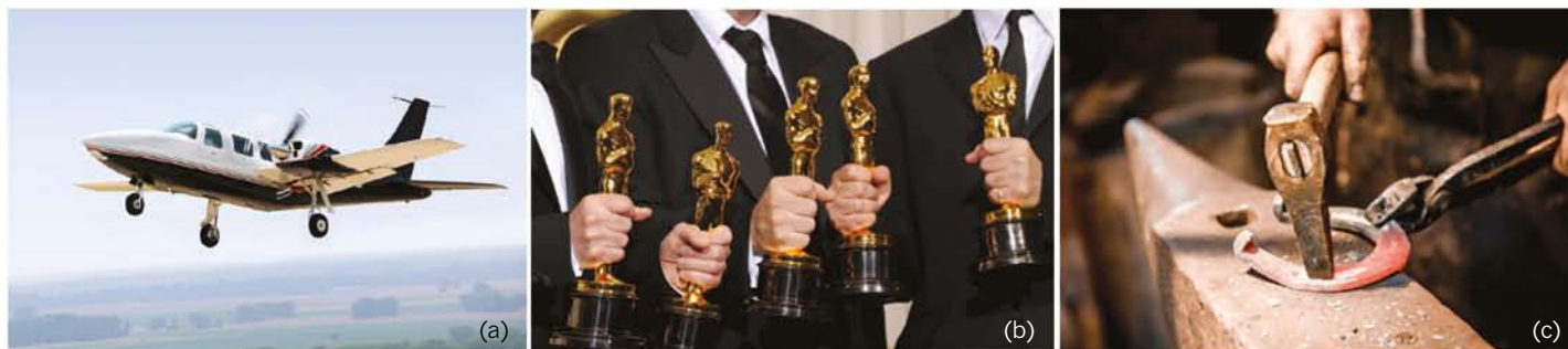
FIGURE 3.5.1 (a) Modified metals are used in aeroplanes, which need to be made from materials that are strong, durable and light. (b) The Oscar statuettes are made of britannium (a mixture of tin, copper and antimony) and then coated successively in layers of copper, nickel, silver and gold. (c) Blacksmiths use heat and hammering tools to modify the properties of the metal used for horseshoes.
