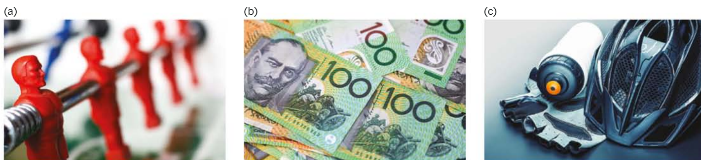
FIGURE 10.1.1 (a) The polymer used to make the toy soccer players in this game was selected for its strength and how easy it is to mould. (b) The polymer bank notes used in Australia are strong and flexible. (c) The polymers in the helmet, gloves and bottle are similar, but differences in processing have given them very different properties.
