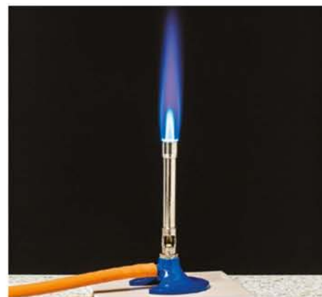
FIGURE 9.1.4 Methane undergoes complete combustion in a Bunsen burner when the air holes are open.
