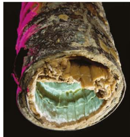
FIGURE 18.1.8 Accumulation of limescale in pipes is a result of the precipitation of soap scum due to the calcium and magnesium ions present in hard water. Eventually, the crystalline deposits can become so severe they block the flow of water.
