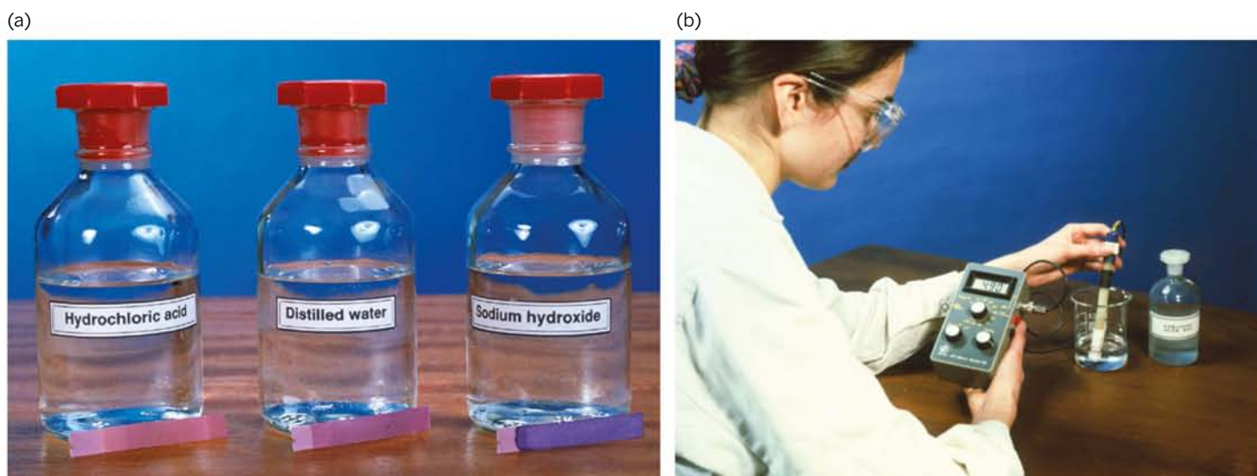
FIGURE 21.1.2 Determining whether a solution is acidic or basic can be qualitative or quantitative. (a) Litmus paper gives a qualitative observation indicating the nature of the solution. (If the paper turns purple, the solution is basic; if the paper turns pink, the solution is acidic.) (b) A calibrated pH meter gives a quantitative measurement indicating the nature of the solution ( \text{pH} < 7 , the solution is acidic; \text{pH} > 7 , the solution is basic.)
