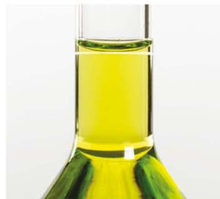
FIGURE 20.2.4 This close-up view of the neck of a standard flask shows the bottom of the meniscus level with the graduation line.
