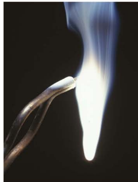
FIGURE 16.1.4 Magnesium ribbon burns brightly when heated in air to form a white powder, magnesium oxide.
