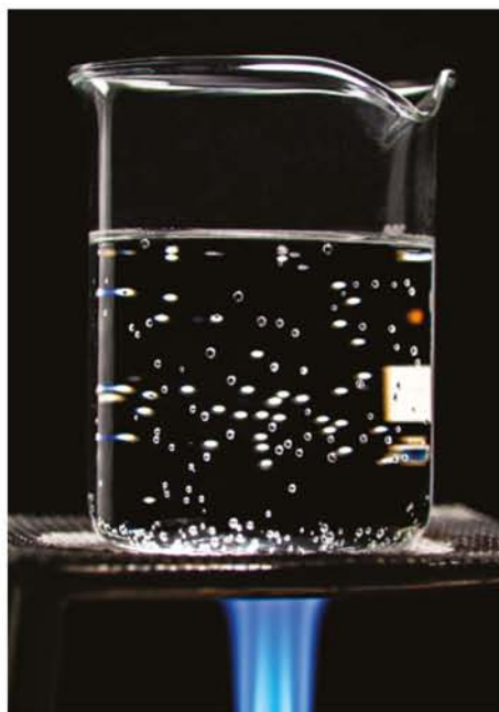
FIGURE 14.2.9 Bubbles of air appear as water is heated. This is because solubility of gases decreases at higher temperatures.
