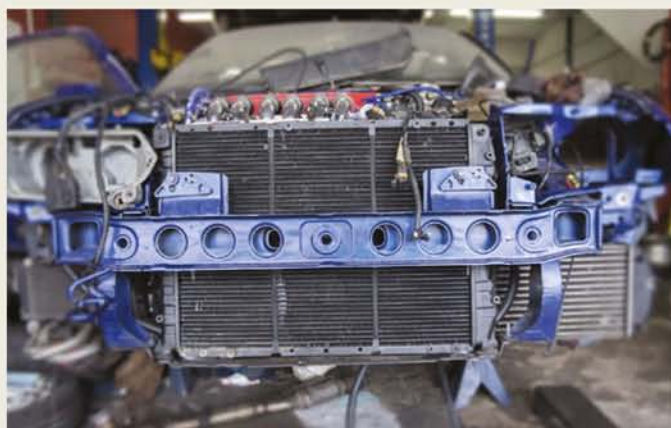
FIGURE 12.3.5 Car radiators make use of the high specific heat capacity of water to discharge excess heat from the engine and maintain performance.
