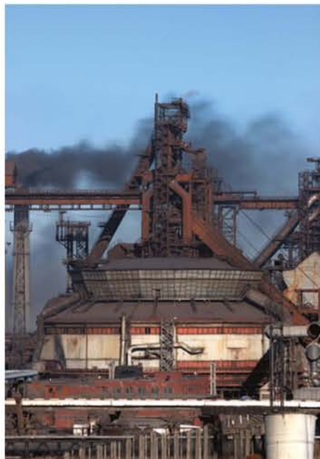
FIGURE 3.4.5 A blast furnace used to extract iron from iron ore. Iron ore is added continuously to the top of the furnace by the conveyor belts on the left-hand side.
