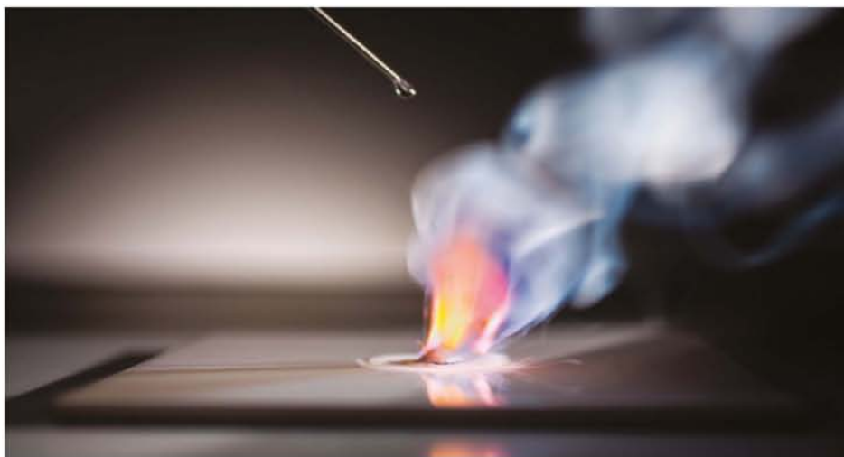
FIGURE 3.3.1 When water is dropped onto metallic potassium, hydrogen gas is produced.
