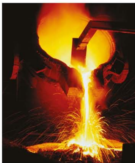
FIGURE 16.1.2 Molten iron from a blast furnace being poured into a bucket.
