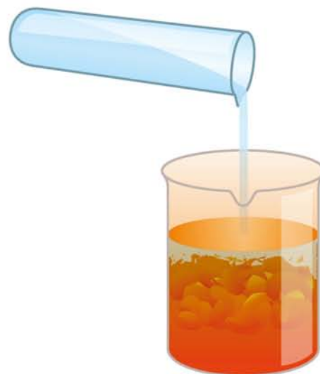
FIGURE 18.2.1 When colourless aqueous solutions of mercury(II) ethanoate and sodium iodide are mixed, they produce a red precipitate, mercury(II) iodide. The mass of the precipitate from this reaction can be used to determine the amount of mercury present in the original sample.
