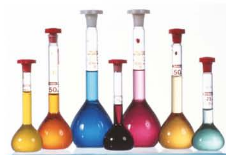
FIGURE 20.2.3 Volumetric flasks of various sizes are used to prepare standard solutions.
