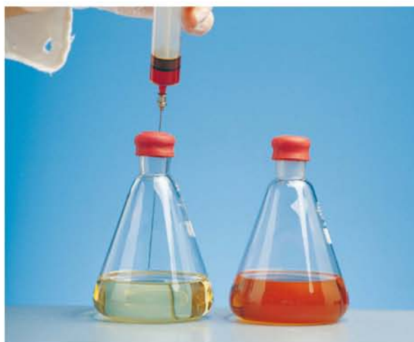
FIGURE 9.2.3 Test for unsaturation. Adding a few drops of orange-coloured bromine solution to hexane (right) produces no reaction. In sunflower oil (left), the colour of the bromine solution disappears almost immediately because molecules in the sunflower oil contain carbon–carbon double bonds, which undergo addition reactions with bromine ( \text{Br}_2 ).
