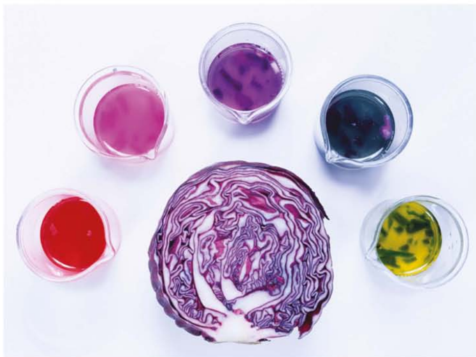
FIGURE 15.1.4 Natural acid–base indicators are found in plants such as red cabbage. Red cabbage extract turns a different colour in (from left to right) strong acid, weak acid, neutral solution, weak base and strong base.
