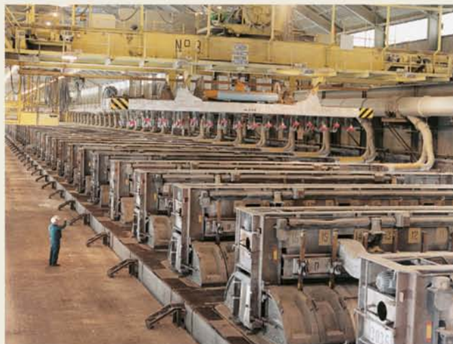
FIGURE 16.2.3 A row of electrolytic cells used for the modern production of aluminium.
