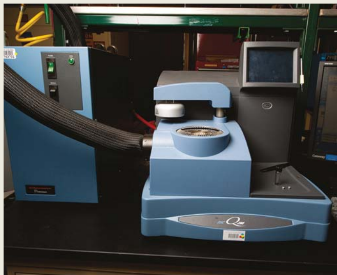
FIGURE 17.2.7 A differential scanning calorimeter is used to measure the effects of temperature on substances.
