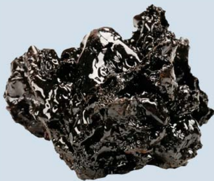
FIGURE 11.2.4 A sample of pitch at room temperature appears solid and shatters when hit with a hammer.
