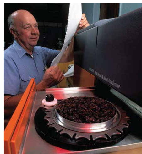
FIGURE 12.1.3 A food chemist uses an infrared spectrometer to evaluate the quality of raisins.
