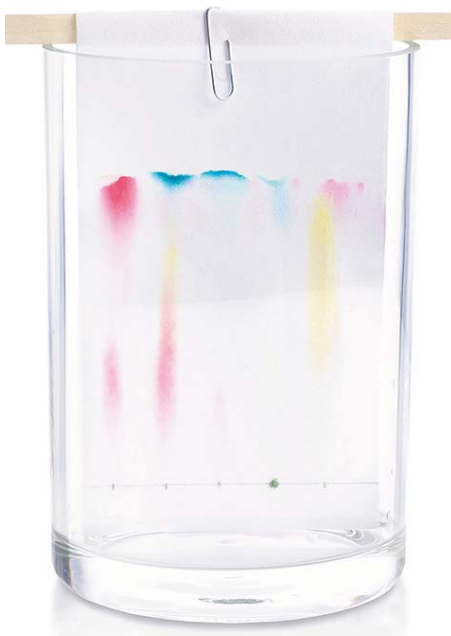
FIGURE 13.1.2 Paper chromatography can be used to separate mixtures of inks into their separate components.
