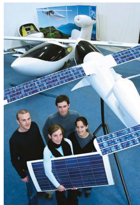
FIGURE 6.1.8 Technicians with a prototype aircraft powered by a combination of solar cells, which power the on-board electronics, and a hydrogen fuel cell, which powers the electric engine.
