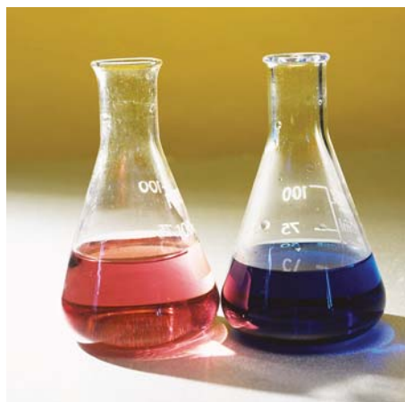
FIGURE 8.5.1 The effect of changes on the equilibrium: \text{Co}(\text{H}_2\text{O})_6^{2+}(\text{aq}) + 4\text{Cl}^-(\text{aq}) \rightleftharpoons \text{CoCl}_4^{2-}(\text{aq}) + 6\text{H}_2\text{O}(\text{l}) The addition of excess \text{Cl}^- ions causes a net forward reaction and the solution turns blue as more \text{CoCl}_4^{2-} is formed. The addition of excess water causes a net reverse reaction and the solution returns to the original pink colour as more [\text{Co}(\text{H}_2\text{O})_6]^{2+} is formed.
