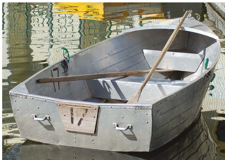
FIGURE 9.2.4 Boats made from aluminium are light, strong and resistant to corrosion.
