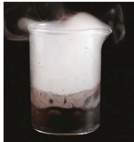
FIGURE 7.2.1 The decomposition of hydrogen peroxide is usually very slow, but the addition of crystals of potassium permanganate results in the rapid evolution of oxygen gas and water vapour.
