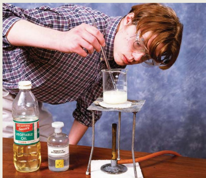
FIGURE 11.4.16 Making soap from vegetable oil and sodium hydroxide solution is a relatively easy reaction to perform in the school laboratory.
