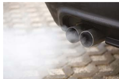
FIGURE 8.5.7 Carbon monoxide gas is formed when hydrocarbon fuels, such as petrol, are burnt in limited supplies of oxygen.
