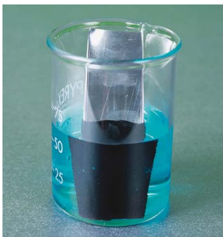
FIGURE 5.1.6 \text{Cu}^{2+}(\text{aq}) ions in blue-coloured copper(II) sulfate solution reacting directly with a strip of zinc metal.
