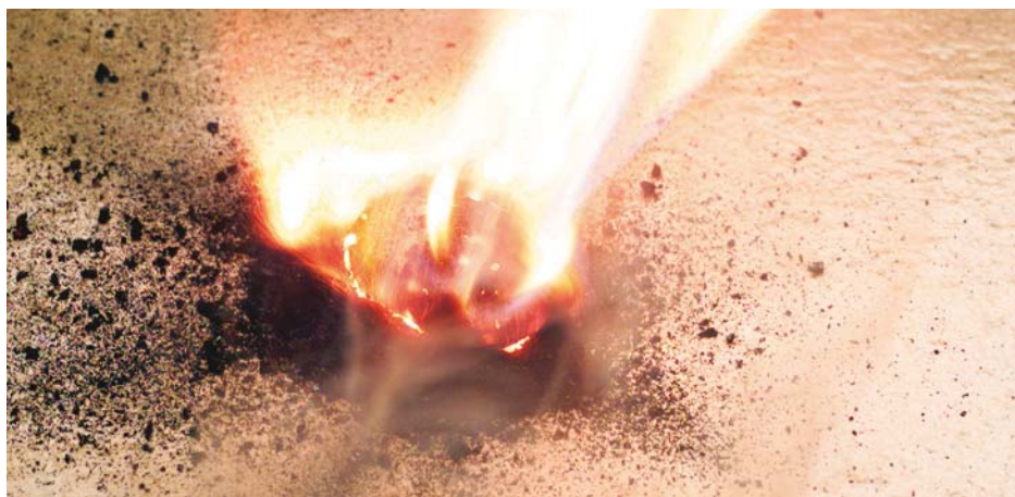
FIGURE 4.1.1 When glycerol is added to potassium permanganate, a vigorous reaction occurs in which the glycerol is oxidised by the potassium permanganate.
