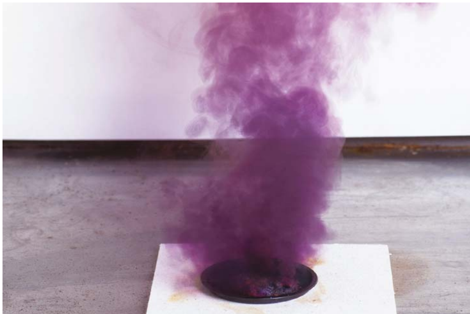
FIGURE 4.1.3 In a vigorously exothermic reaction, aluminium is oxidised by iodine upon the addition of a few drops of water, to form aluminium iodide. The heat that is released during the reaction causes iodine to sublime from a solid to a purple gas.
