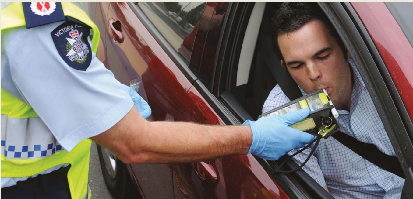
FIGURE 4.3.6 Breathalysers are used to analyse the blood alcohol content of motorists. The sensor detects the change in colour as the ethanol is oxidised to ethanoic acid in the presence of acidified potassium dichromate.
