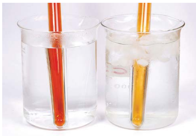
FIGURE 8.6.7 Equilibrium mixtures of NO_2 and N_2O_4 in hot water and ice. Heating the mixture favours the formation of brown NO_2 gas.
