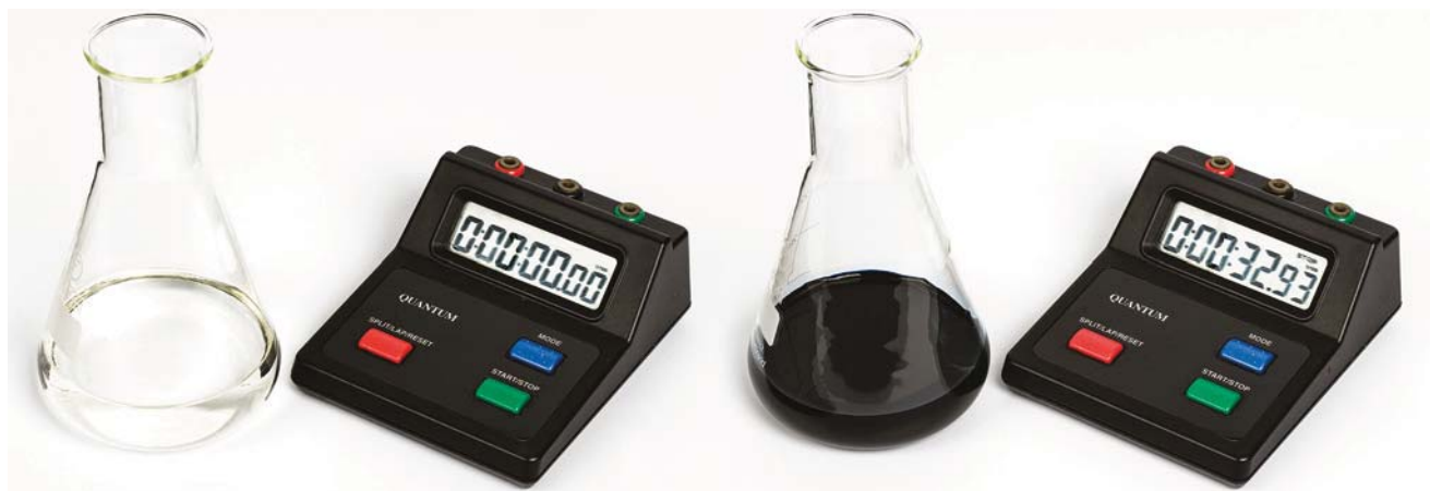
FIGURE 4.3.1 This redox reaction involving colour changes is known as a clock reaction. The black compound is a starch–iodine complex.
