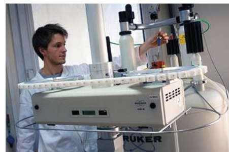
FIGURE 12.2.1 A research chemist places a sample tube into an NMR spectrometer.
