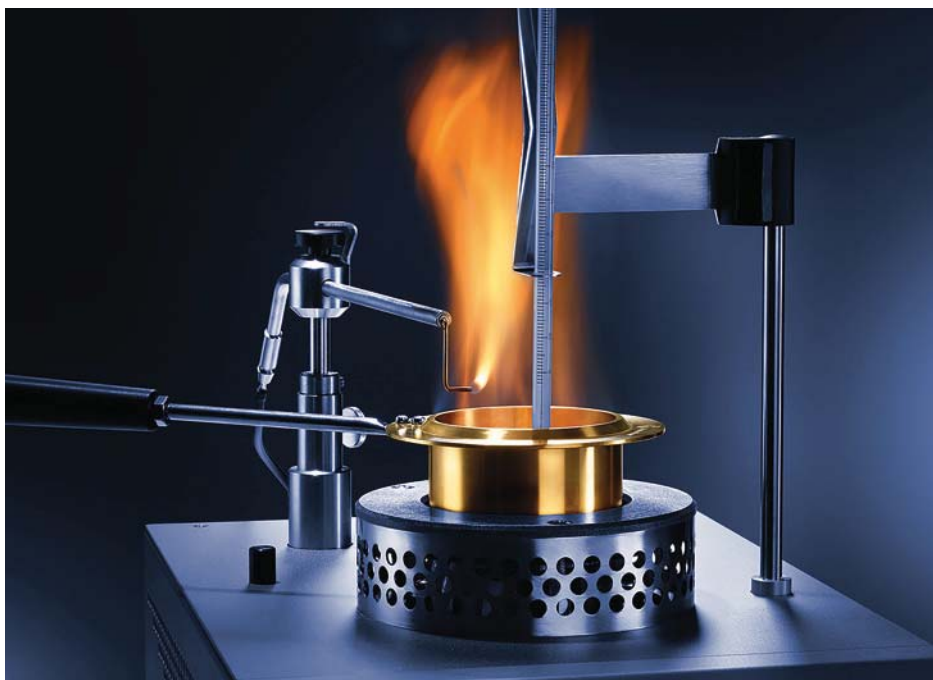
FIGURE 11.2.7 This apparatus measures the flashpoint of fuels. The fuel is heated steadily in a metal cup and, at intervals, a flame is brought above the liquid in the cup. The flashpoint is the lowest temperature at which the fuel will ignite when the flame is brought above it.
