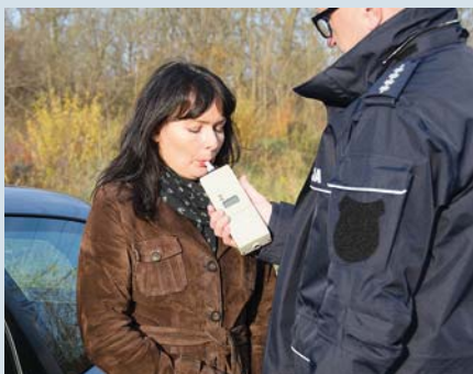
FIGURE 12.1.12 A driver's blood alcohol level is tested in a roadside breath test.
