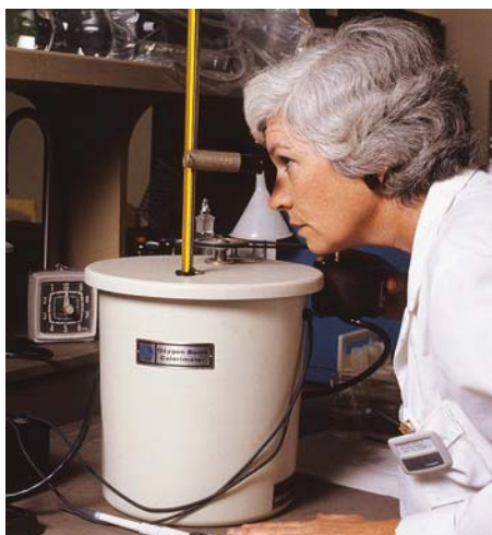
FIGURE 17.3.1 Bomb calorimeter temperature changes being observed by a laboratory technician. Bomb calorimeters are used to measure the heat released by combustion reactions. The rise in temperature is used to calculate the energy released.
