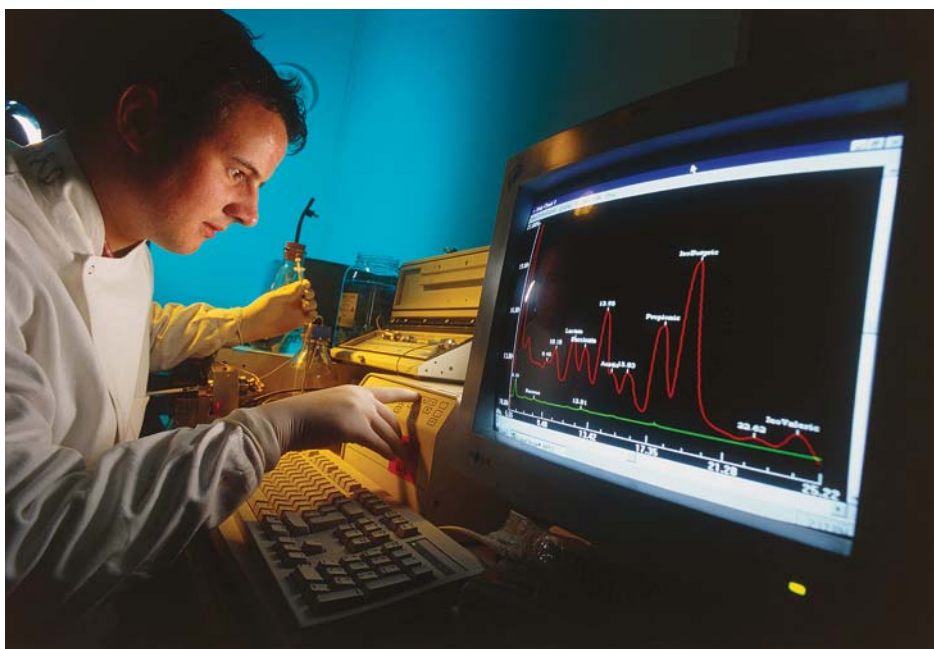
FIGURE 13.2.3 A research chemist uses HPLC to analyse the components in a mixture for medical research.
