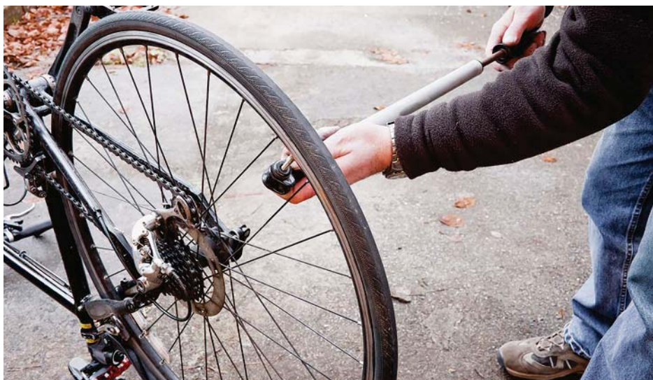
FIGURE 3.1.4 Pumping more air into a tyre increases the pressure in the tyre because more particles are being pumped into a nearly fixed volume.
