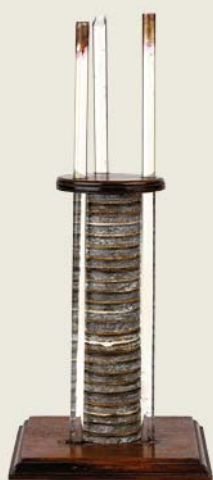
FIGURE 5.1.2 An original voltaic pile. The pile is 15 cm high and contains alternating copper and zinc discs separated by cardboard.
