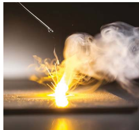
FIGURE 5.2.1 Water dropped onto sodium metal. Sodium is highly reactive; the products are sodium hydroxide and hydrogen gas.
