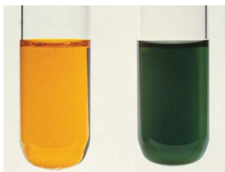
FIGURE 4.3.4 The oxidation of ethanol, described in Worked Example 4.3.2, was the basis of an older form of the breathalyser. The presence of alcohol in a motorist's breath was identified by a colour change in the oxidising agent, potassium dichromate. During the reaction, the yellow-orange colour of dichromate ions changed to the green colour of chromium(III) ions as the alcohol was oxidised.
