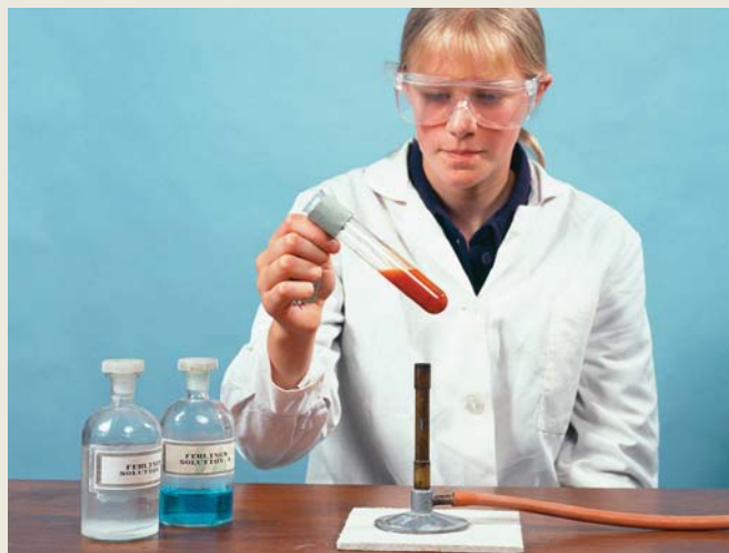
FIGURE 16.3.2 A student conducts the Fehling's test on a solution containing glucose. On heating the reaction mixture it produces a reddish-brown colour. The amount of reddish-brown precipitate formed is proportional to the amount of glucose in the solution.
