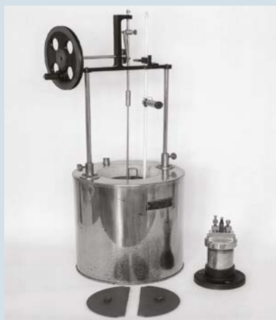
FIGURE 17.3.2 Berthelot's bomb calorimeter. The reaction vessel was lined with platinum to avoid corrosion from acidic vapours and solutions.
