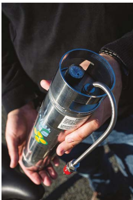
FIGURE 6.1.1 A hydrogen fuel cell for an electric bicycle. The hydrogen bicycle operates like a standard electric bicycle, but the battery lasts three times longer.
