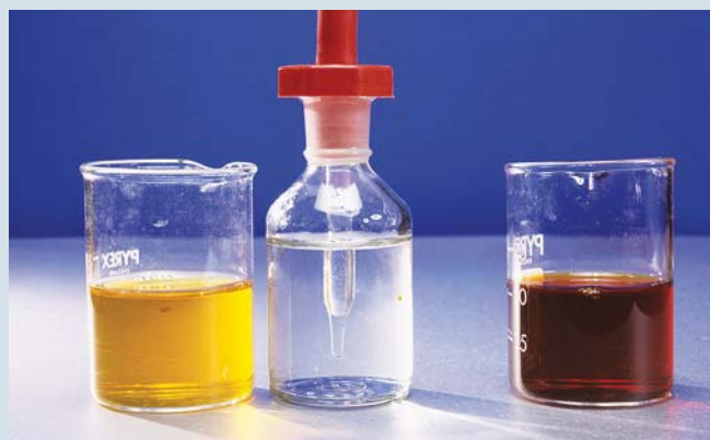
FIGURE 8.2.2 Chemicals needed to make fake blood. From left to right: a solution containing \text{Fe}^{3+} , a solution containing \text{SCN}^- , and an equilibrium mixture of \text{Fe}^{3+} , \text{SCN}^- and \text{FeSCN}^{2+} .
