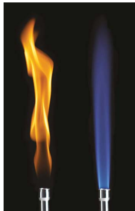
FIGURE 2.3.2 The yellow flame of a Bunsen burner is due to incomplete combustion and produces carbon as a product. The blue flame is a hotter flame that occurs when the collar hole is open and more oxygen is allowed into the reaction. Complete combustion can then occur.
