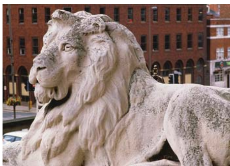
FIGURE 7.1.4 This limestone statue has become pitted in recent years. Limestone (calcium carbonate) reacts more rapidly with the increased concentration of hydrogen ions in rainwater.
