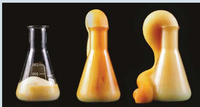
FIGURE 4.3.7 The 'elephant's toothpaste' demonstration involves a redox reaction in which hydrogen peroxide reacts with itself to form water and oxygen gas. In this reaction, the hydrogen peroxide is both the reducing agent and the oxidising agent. In this image, solid potassium iodide catalyst is added to hydrogen peroxide solution. Red colouring has also been added for effect.
