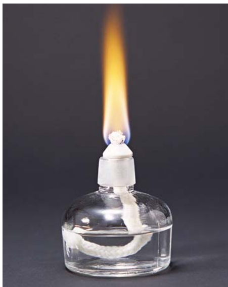
FIGURE 2.3.4 Ethanol burning in a spirit burner. Combustion of 1 gram of ethanol releases almost 30 kJ of energy.
