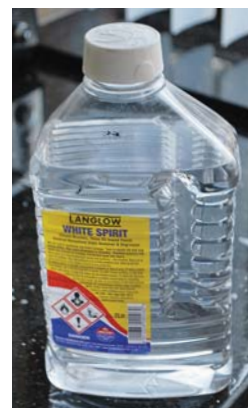
FIGURE 11.1.7 White spirit contains a mixture of alkanes. It is a useful solvent for other non-polar liquids.
