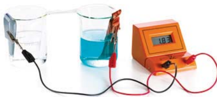
FIGURE 5.1.3 Construction of a galvanic cell from simple laboratory equipment.
