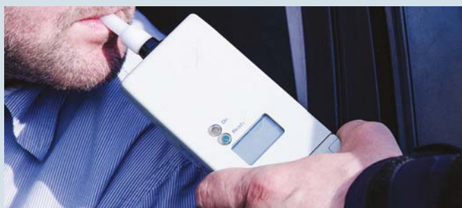
FIGURE 6.1.4 Hand-held breathalysers are a type of fuel cell.
