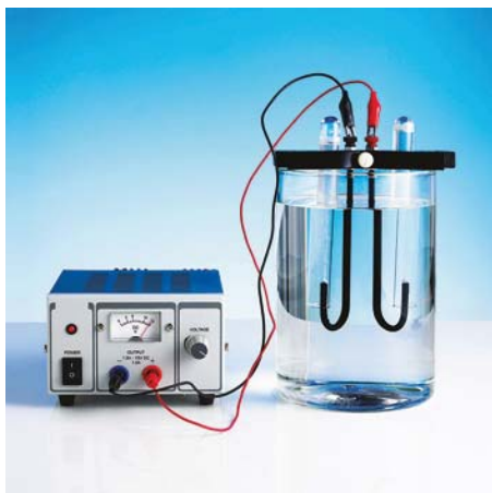
FIGURE 9.1.1 During electrolysis, electrical energy is used to make redox reactions occur. In this experiment, electricity passing through dilute sodium chloride solution creates bubbles of hydrogen gas at the left-hand electrode and bubbles of oxygen gas at the right-hand electrode. The gases are being collected in the test tubes.
