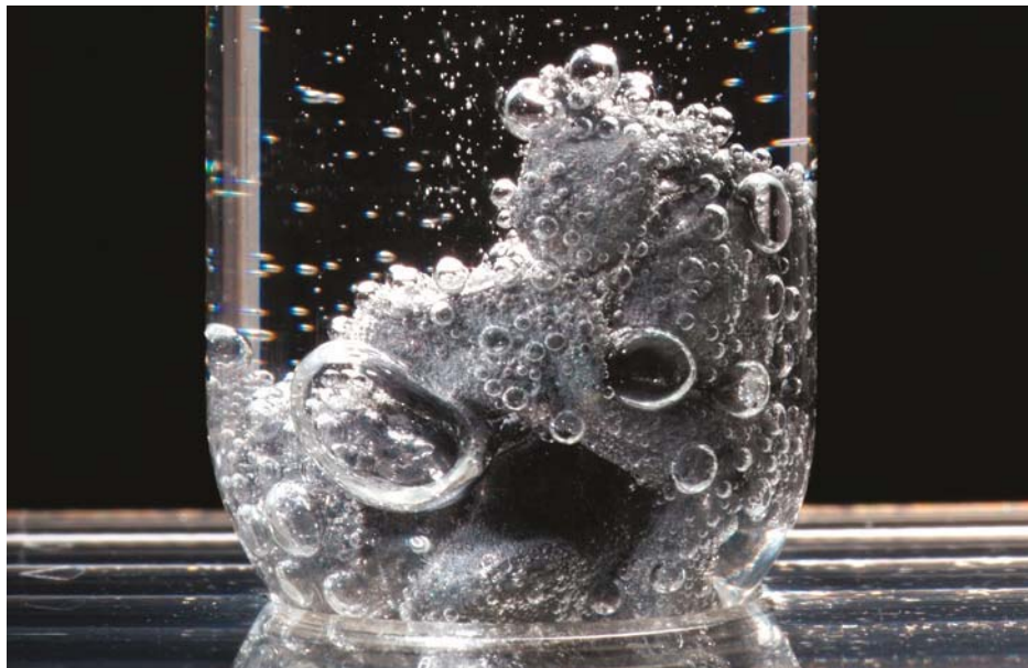
FIGURE 2.2.4 When zinc comes into contact with hydrochloric acid, it reacts almost immediately. The reactants have sufficient energy to ‘overcome’ the activation energy barrier.
