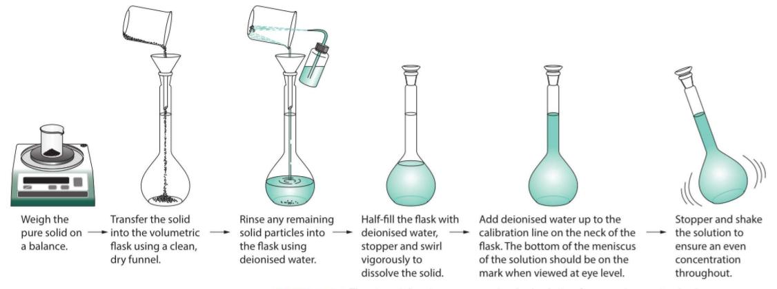
FIGURE 14.1.4 The steps taken to prepare a standard solution from a primary standard
