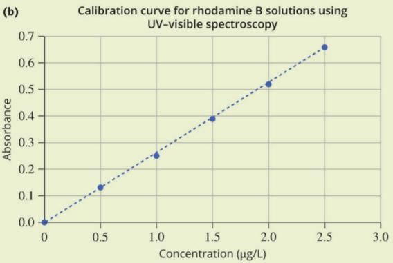
FIGURE 1.4.10 (a) Rhodamine B is a fluorescent pink dye which dissolves readily in water and also in a number of organic solvents. (b) A calibration curve for a solution of rhodamine B, determined using UV–visible spectroscopy.
