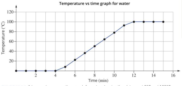
FIGURE 10.3.2 A temperature versus time graph for water, showing the plateaus at 0°C and 100°C
