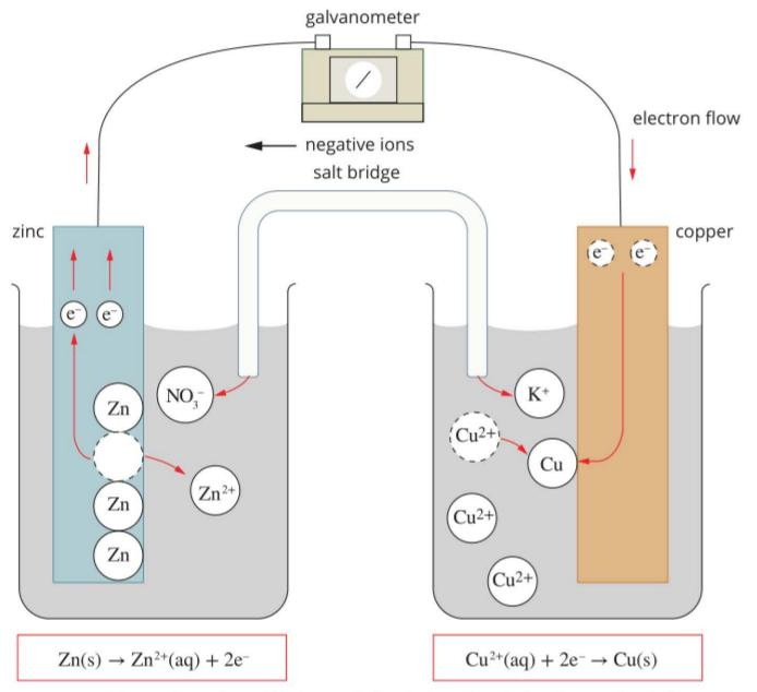
FIGURE 12.3.1 The equipment used to demonstrate electron flow during the reaction between zinc and copper(II) sulfate
