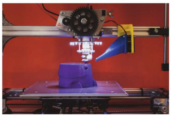
FIGURE 9.3.8 This 3D printer uses an ABS copolymer filament to make an object.
