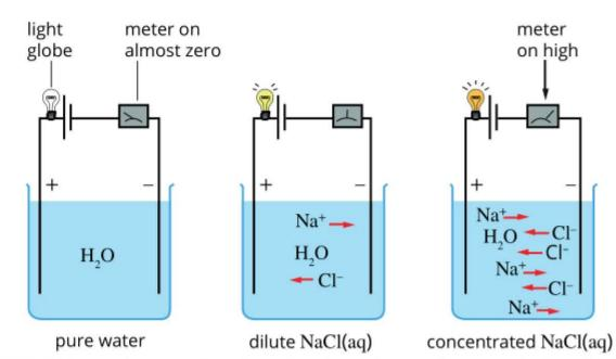
FIGURE 16.1.10 The conductivity of a salt solution depends upon the concentration of salt in the solution. The flow of current increases as the concentration of ions increases.
