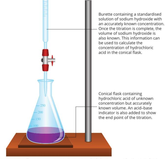
FIGURE 14.1.6 The equipment used in the titration of HCI (in the conical flask) with NaOH (in the burette)
