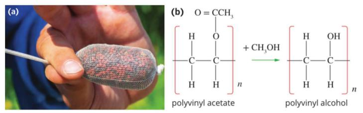
FIGURE 9.5.1 (a) Polyvinyl alcohol (PVA) bags that dissolve in water. (b) The formation of PVA from polyvinyl acetate. PVA is water-soluble because it can form hydrogen bonds with water.
