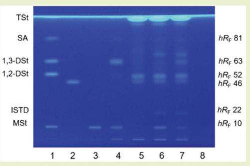
FIGURE 6.2.5 A photo of a chromatogram taken under UV light, showing mixtures of standards (1–4) and those of aerosol whipped cream samples (5–8).
