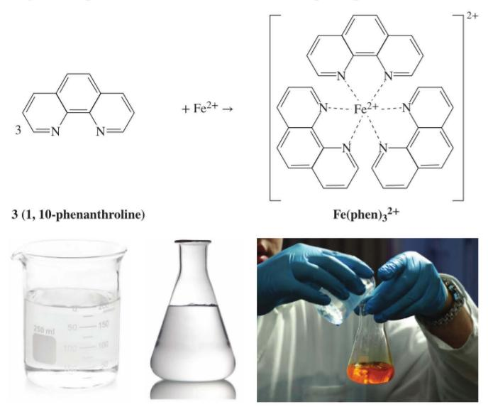
FIGURE 16.3.8 A colourless solution of Fe<sup>2+</sup> reacts with a colourless solution of 1,10-phenanthroline, forming a bright orange metal complex, that can be analysed by colorimetry or UV–visible spectroscopy.
