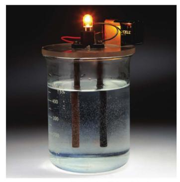
FIGURE 16.1.9 A simple circuit for detecting salinity. The brighter the light emitted from the globe, the greater the conductivity of the solution.
