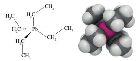
FIGURE 16.1.6 Two different structural representations of tetraethyl lead. This compound has four ethyl groups (-CH<sub>2</sub>CH<sub>3</sub>) bonded to a lead atom in the centre of the molecule.
