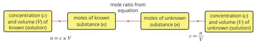
FIGURE 14.2.1 Flow chart for solution volume-volume stoichiometry calculations
