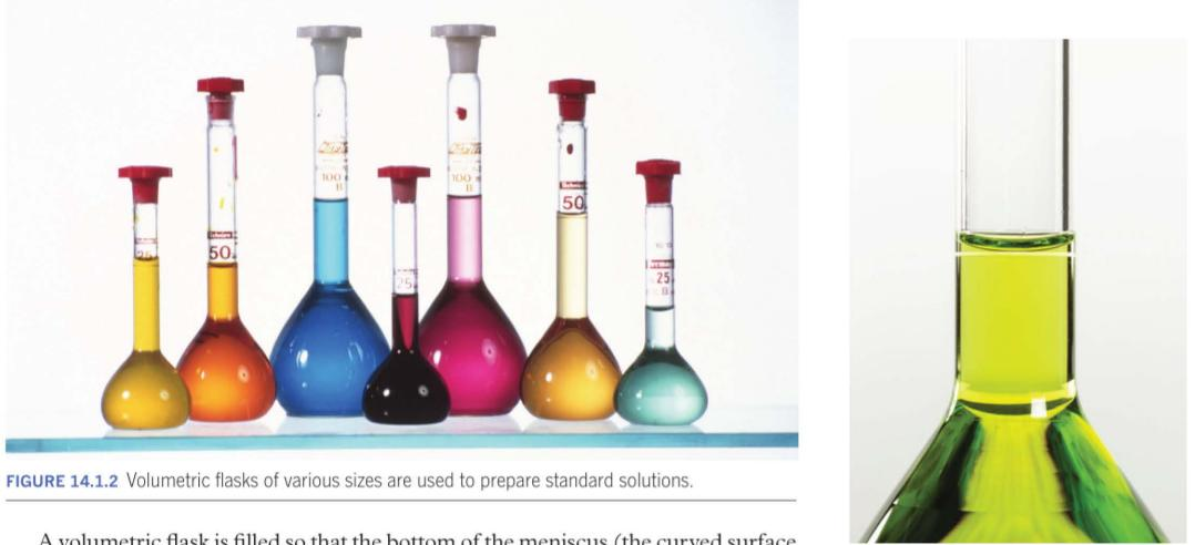
A volumetric flask is filled so that the bottom of the meniscus (the curved surface of the solution) is level with the graduation line on the neck of the flask (Figure 14.1.3). Your eye should be level with the line to avoid **parallax errors** (errors caused by the shift in the apparent position of an object due to the viewing angle).
