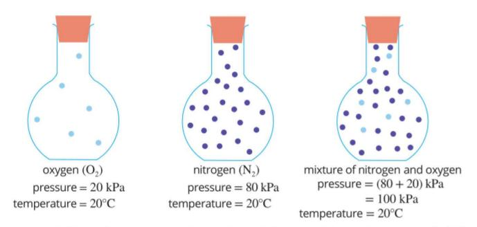
FIGURE 15.2.5 The total pressure of a mixture of gases is the sum of the partial pressures (individual pressures) of each of the gases in the mixture.
