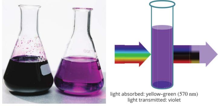
FIGURE 16.3.2 Two solutions of potassium permanganate (KMnO<sub>4</sub>) appear purple because they absorb yellow-green light. The 0.001 M solution on the right is lighter in colour than the 0.01 M solution because it absorbs less light.
