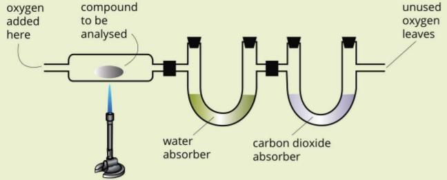
FIGURE 7.4.3 Experimental set-up for the elemental analysis of an organic compound
