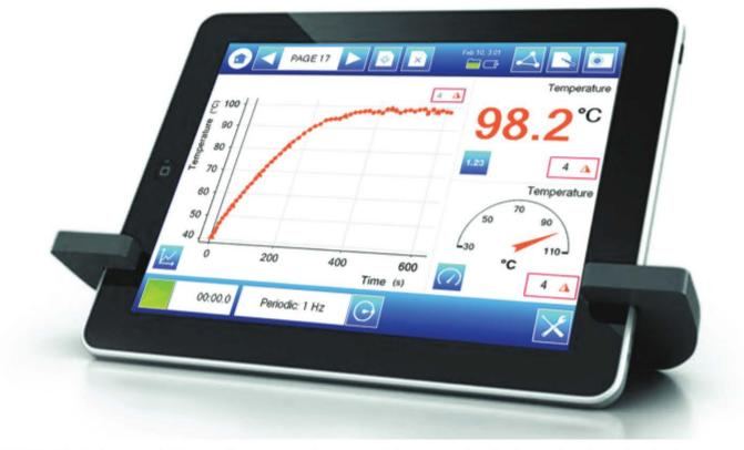
FIGURE 1.3.7 Data acquisition software produces real-time graphs that can be downloaded or printed.
