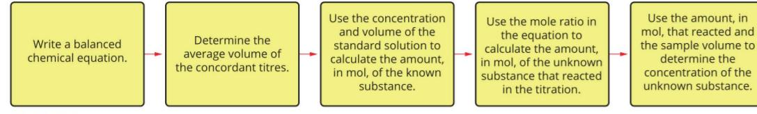
FIGURE 14.2.2 Flow chart summarising the steps in the calculation of the concentration of an unknown substance using data from a titration
