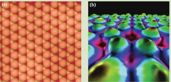
(a) Coloured image of copper atoms produced by a scanning tunnelling microscope (STM). (b) Silicon atoms on a silicon chip imaged with a scanning tunnelling microscope
