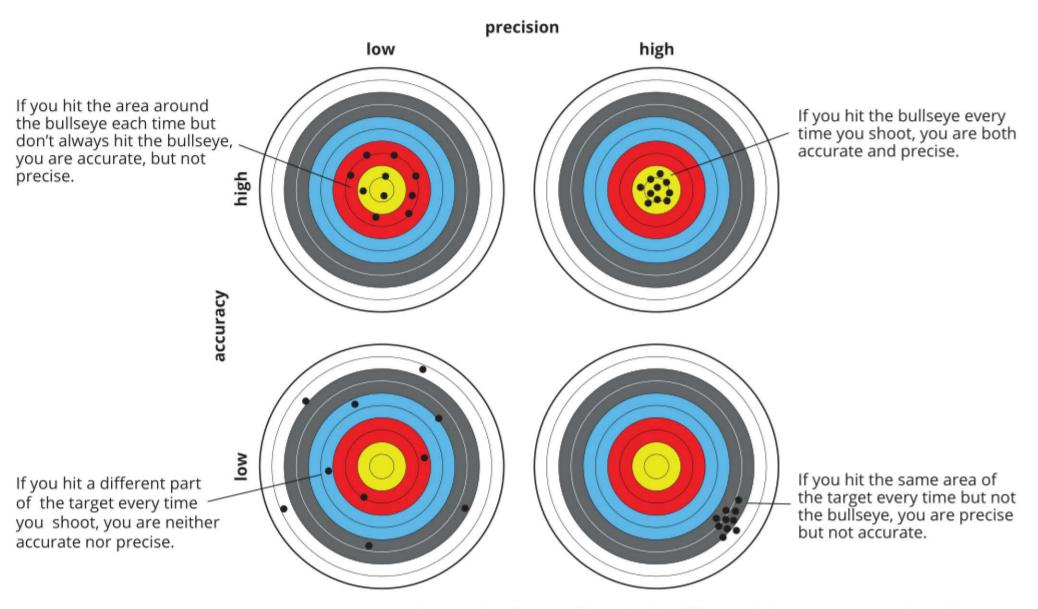
FIGURE 1.3.5 An example of a target illustrates the difference between accuracy and precision.
