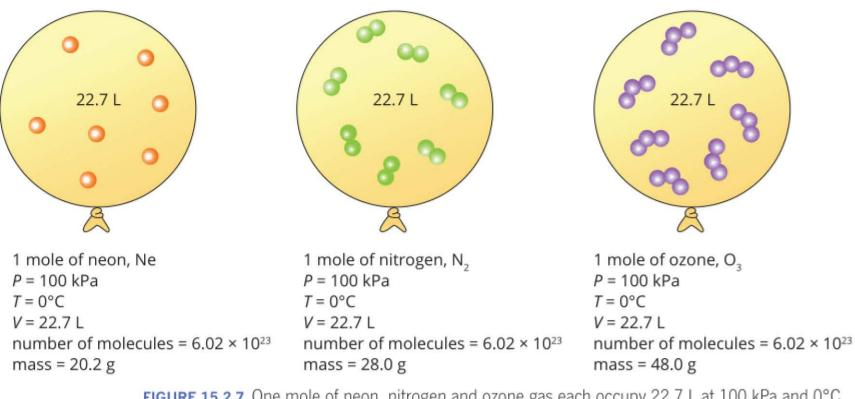
FIGURE 15.2.7 One mole of neon, nitrogen and ozone gas each occupy 22.7 L at 100 kPa and 0°C (273 K).
