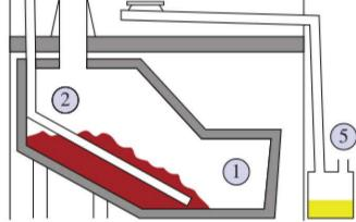
**FIGURE 2.4.12** A diagram of a composting toilet with urine diversion and dehydration: 1. solid waste compartment; 2. ventilation pipe; 3. toilet; 4. urinal; 5. urine collection and dehydration
