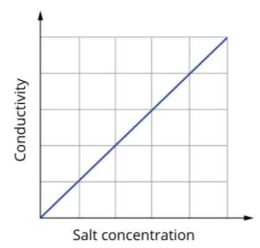
FIGURE 16.1.11 The conductivity of a salt solution increases with concentration. At low concentrations, the relationship is considered to be a linear one.
