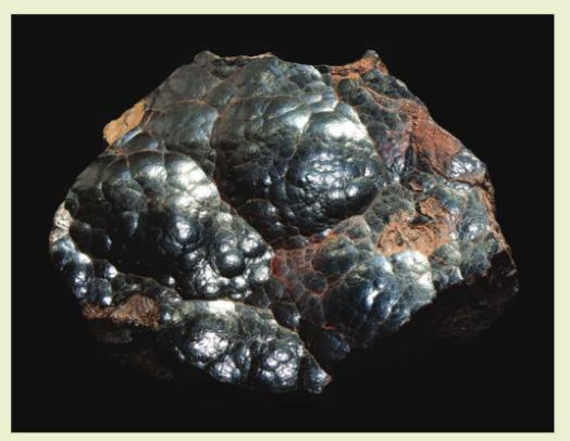
**FIGURE 4.3.2** The mineral haematite ( $Fe_2O_3$ ) is mined as the main source of iron. This sample has been partially polished, removing most of the red oxide coating that forms upon exposure to air.
