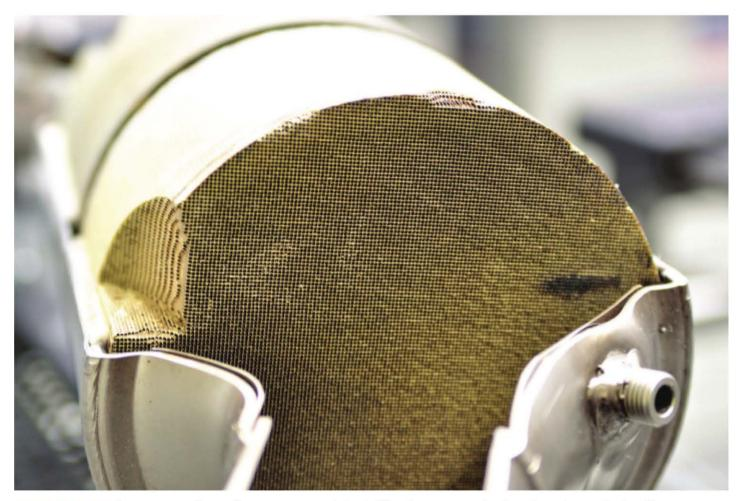
**FIGURE 4.3.8** A cross-section of a new car catalyst. The honeycomb structure is coated with a catalyst made from an alloy of platinum and iridium.
