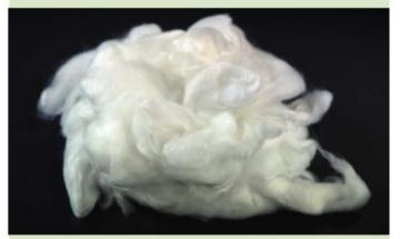
FIGURE 9.5.9 This nanollose fibre was manufactured from coconut waste using bacteria.
