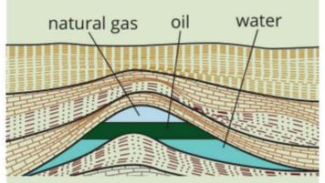
Typical structure of the impervious rock that traps oil and natural gas underground and creates an oil field
