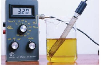
FIGURE 11.5.7 A pH meter can be used to measure the acidity of a solution.
