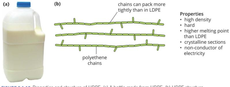
FIGURE 9.1.10 Properties and structure of HDPE. (a) A bottle made from HDPE. (b) HDPE structure.
