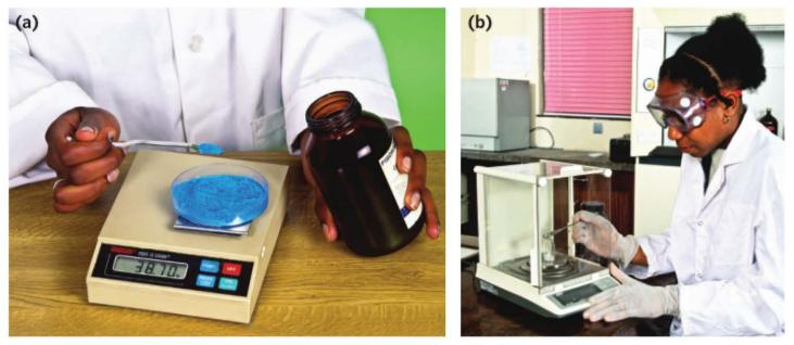
FIGURE 14.1.1 (a) A top-loading balance and (b) an analytical balance can be used to accurately weigh substances used in chemical analysis.
