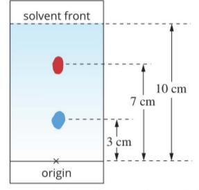
**FIGURE 6.2.3** A chromatogram of a sample that consists of two components. The distances from the origin enable  $R_i$  calculations.
