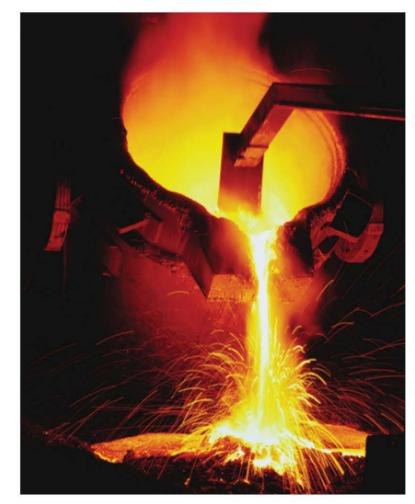
FIGURE 12.1.2 Molten iron from a blast furnace being poured into a bucket
