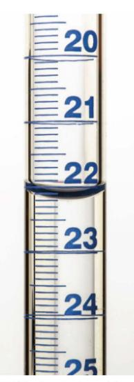
FIGURE 14.1.9 The burette is read from the bottom of the meniscus and the volume is estimated to the second decimal place. The volume measurement in this case is 22.18 mL.
