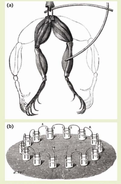
FIGURE 12.3.5 (a) In 1791 Luigi Galvani observed that a frog's legs twitched due to the flow of electricity between copper and iron. (b) A 'crown of cups' battery constructed by Alessandro Volta in 1800. This is a series of containers (half-cells) holding saltwater and electrodes, consisting of plates of zinc (Z) and copper (C). Metal hoops (A) connect the cells in series.
