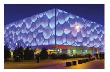
FIGURE 9.3.7 The outer shell of the Water Cube Stadium in Beijing, China, is made of ETFE, a new copolymer building material.
