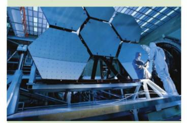
Some of the 18 mirror segments of the James Webb Space Telescope. The mirrors are supported by beryllium ribs that maintain the mirror's shape under extreme conditions.
