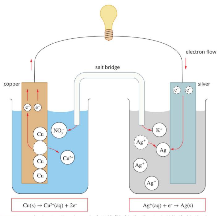
FIGURE 12.3.3 A galvanic cell made up of a Cu(s)/Cu<sup>2+</sup>(aq) half-cell and a Ag(s)/Ag<sup>+</sup>(aq) half-cell
