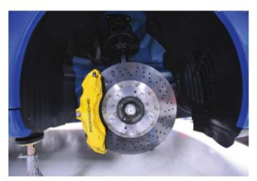
FIGURE 5.1.4 Ceramic brake discs work more effectively than steel ones at high temperatures.
