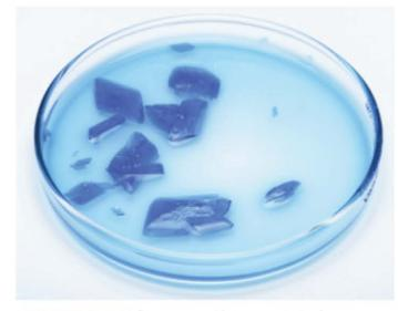
FIGURE 13.1.5 Copper sulfate crystals form when a solution cools to below a temperature where the solution becomes saturated.
