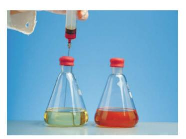
FIGURE 8.2.9 Test for unsaturation. Adding a few drops of orange-coloured bromine solution to hexane (right) produces no reaction. In sunflower oil (left), the colour of the bromine solution disappears almost immediately because molecules in the sunflower oil contain carbon–carbon double bonds, which undergo addition reactions with bromine (Br<sub>2</sub>).
