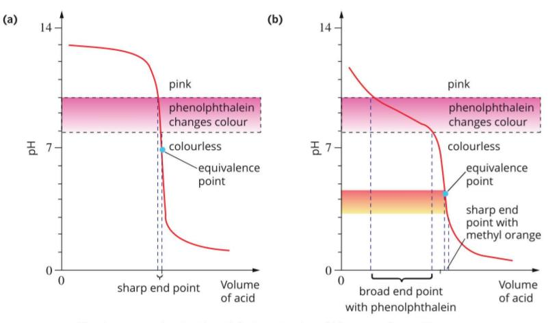
FIGURE 14.1.12 Titration curves showing the pH during a titration of (a) a strong base with a strong acid, and (b) a weak base with a strong acid. Phenolphthalein, which changes colour in the pH range 8.3–10.0, gives a sharp end point in (a) but a broad end point in (b). Methyl orange, which changes colour between pH 3.1 and 4.4, would be a more suitable indicator for the second titration.
