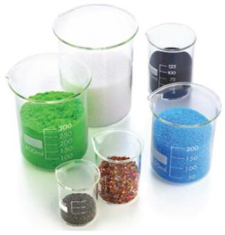
FIGURE 7.3.2 A collection of beakers, each containing one mole of a substance. Each has a different weight and volume. Clockwise from top left the substances are: sucrose, potassium permanganate, copper(II) sulfate, copper turnings, iron filings and nickel(II) chloride.
