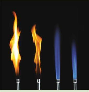
The yellow flame of a Bunsen burner is due to incomplete combustion and produces carbon. The blue flame is the hotter flame that occurs when complete combustion is occurring.
