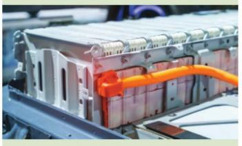
A lithium-ion battery pack and power connections in an electric car
