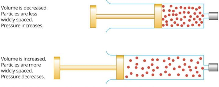
FIGURE 15.2.8 The pressure of the gas in the syringe is affected by a change in volume.
