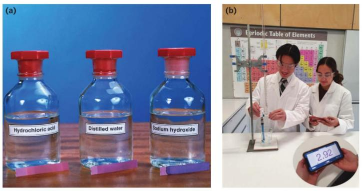
**FIGURE 1.3.2** (a) Litmus paper can be used to indicate the acidity of a solution. If the paper turns blue, the solution is basic; if the paper turns pink, the solution is acidic. (b) A pH probe measures pH quantitatively. If the pH < 7 at 25°C, the solution is acidic; if the pH > 7 at 25°C, the solution is basic.
