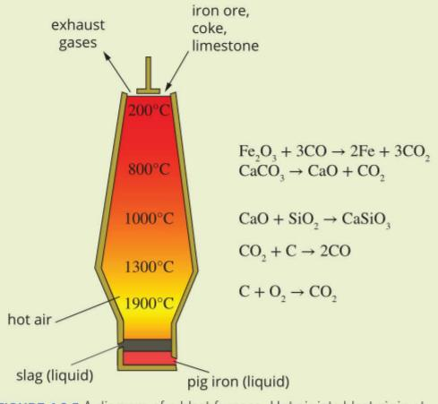
FIGURE 4.3.5 A diagram of a blast furnace. Hot air jets blast air in at the bottom. Iron ore, coke and limestone are added at the top.
