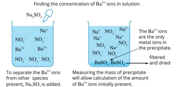
**FIGURE 16.2.3** The principle of gravimetric analysis: Ba<sup>2+</sup> ions in a solution are separated from Na<sup>+</sup> ions and NO<sub>3</sub><sup>-</sup> ions by precipitation. The precipitate is then collected and dried, so that the initial mass of Ba<sup>2+</sup> can be determined using stoichiometry.
