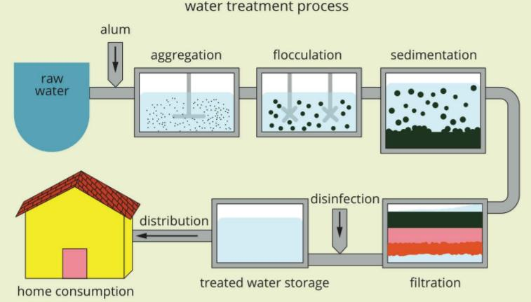
FIGURE 13.1.7 Stages in the purification of drinking water at the Winneke treatment plant, Sugarloaf Reservoir
