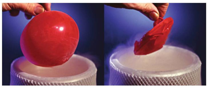
**FIGURE 15.2.2** A balloon filled with air at room temperature is dipped into liquid nitrogen at -196°C. The drop in temperature causes the volume of the air inside the balloon to decrease dramatically.
