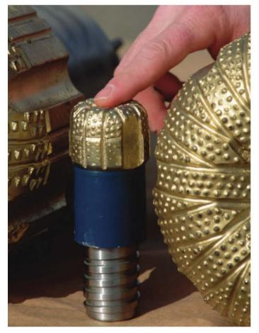
FIGURE 3.5.5 Diamond-tipped drills used to drill through rock in the oil mining industry
