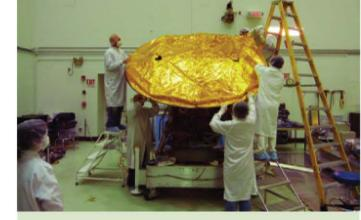
A gold-coated radiation shield is installed on a section of a satellite.
