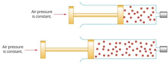
FIGURE 15.2.10 When the amount of gas in the syringe is doubled, the volume doubles, provided the pressure on the plunger and the temperature of the gas remain constant.
