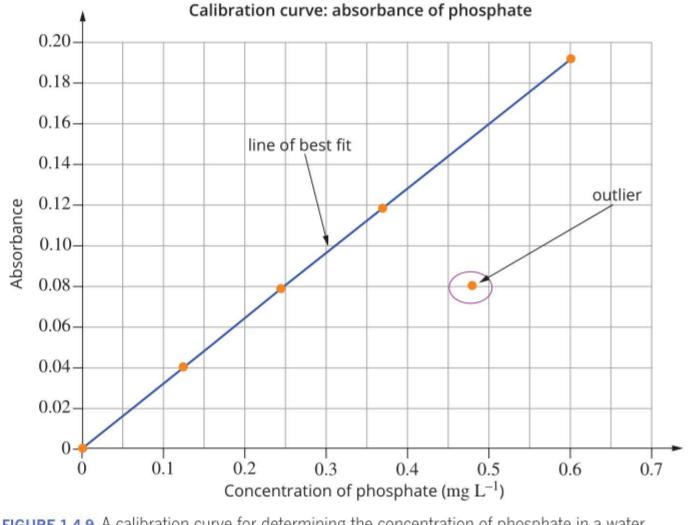
FIGURE 1.4.9 A calibration curve for determining the concentration of phosphate in a water sample
