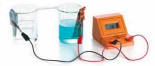
FIGURE 5.1.3 Construction of a galvanic cell from simple laboratory equipment
