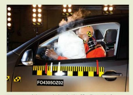
FIGURE 6.1.6 Airbags are deployed within 30 milliseconds of an impact.
