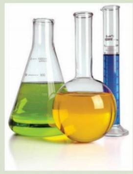
Glassware that is used in the laboratory is made of borosilicate glass.
