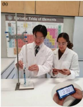
FIGURE 1.3.3 (a) Litmus paper can be used to indicate the acidity of a solution qualitatively. (b) A pH probe measures pH quantitatively.
