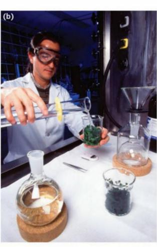
FIGURE 15.1.7 (a) Solvent extraction is used to extract components from plants. (b) A chemist adding solvent to shredded leaves.
