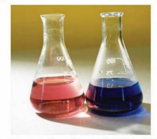
**FIGURE 7.4.1** The effect of changes on the equilibrium  $Co(H_2O)_6^{2+}(aq) + 4CI^{-}(aq) \rightleftharpoons CoCI_4^{2-}(aq) + 6H_2O(I)$ . The addition of excess CI<sup>-</sup> ions causes a net forward reaction, and the solution turns blue as more  $CoCI_4^{2-}$  is formed. The addition of excess water causes a net reverse reaction, and the solution returns to the original pink colour as more  $[Co(H_2O)_6]^{2+}$  is formed.
