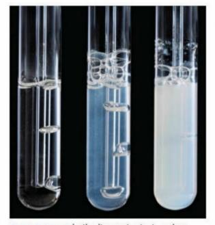
FIGURE 13.1.8 In the limewater test, carbon dioxide is bubbled through limewater, turning the limewater milky.
