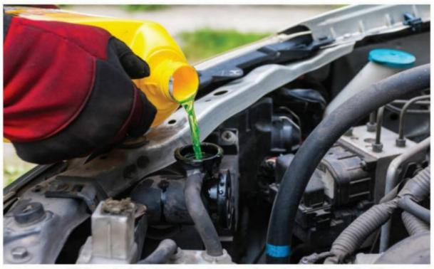
FIGURE 10.6.2 Ethylene glycol mixed with water is commonly used as a coolant and anti-freeze agent in car engines.
