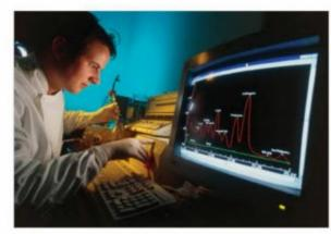
FIGURE 14.4.4 A research chemist uses HPLC to analyse the components in a mixture for medical research.
