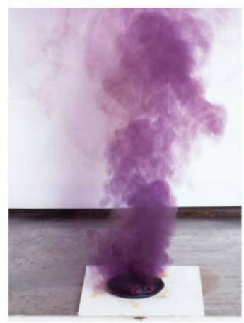
FIGURE 4.1.3 In a vigorously exothermic reaction, aluminium is oxidised by iodine upon the addition of a few drops of water, to form aluminium iodide. The heat that is released during the reaction causes iodine to sublime from a solid to a purple gas.
