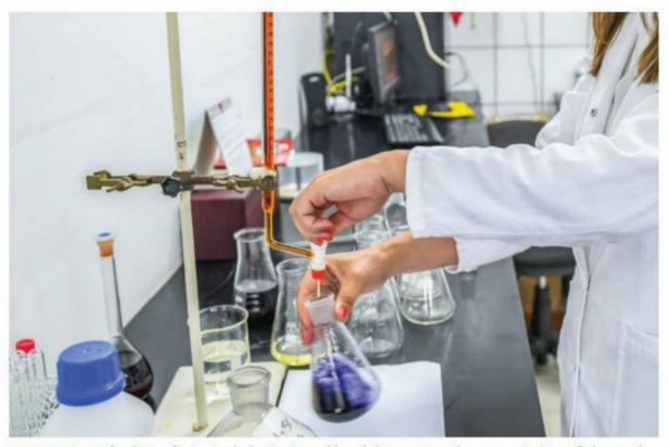
FIGURE 13.2.7 Analysis of wine includes testing pH and determining the concentration of chemicals such as ethanol, sulfur dioxide and malic acid.
