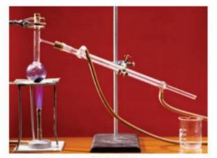
FIGURE 13.1.1 Simple distillation apparatus used to separate two or more liquids
