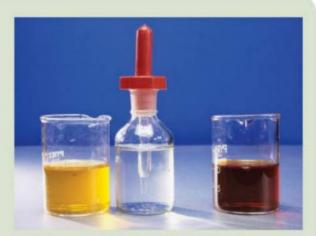
Chemicals needed to make fake blood, from left to right: a solution containing  $Fe^{3+}$ , a solution containing SCN<sup>-</sup>, and an equilibrium mixture of  $Fe^{3+}$ , SCN<sup>-</sup> and  $FeSCN^{2+}$
