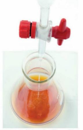
FIGURE 13.2.4 Equipment used to complete a typical redox titration
