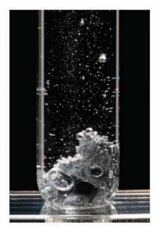
FIGURE 2.1.3 When zinc comes into contact with hydrochloric acid, it reacts almost immediately. The reactants have sufficient energy to 'overcome' the activation energy barrier.
