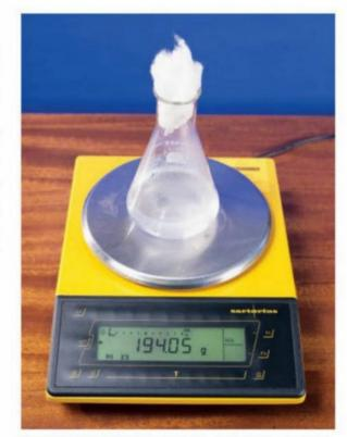
FIGURE 6.1.4 Apparatus to monitor the mass of carbon dioxide gas released during a reaction between marble chips and an acid
