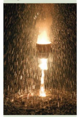
The thermite reaction between iron(III) oxide and aluminium produces a huge quantity of heat and molten iron which flows down from the reaction vessel.
