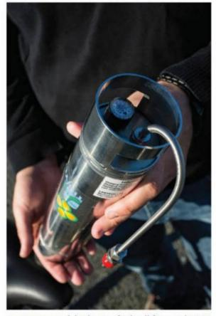
FIGURE 5.3.1 A hydrogen fuel cell for an electric bicycle. The hydrogen bicycle operates like a standard electric bicycle, but the battery lasts longer.
