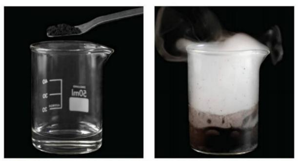
FIGURE 6.1.2 The decomposition of hydrogen peroxide is usually very slow, but the addition of solid manganese dioxide, MnO<sub>2</sub>, results in the rapid production of oxygen gas and water vapour.
