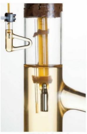
FIGURE 13.1.3 A Thiele tube is set up to determine the melting point of a yellow solid.
