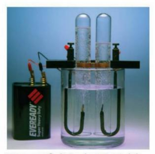
**FIGURE 1.3.4** Qualitative observations include the production of a gas at an anode or cathode during electrolysis.
