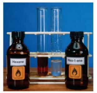
**FIGURE 13.1.5** When hex-1-ene is added to aqueous bromine, the solution decolourises. When hexane is added to aqueous bromine, the red-orange bromine colour remains.
