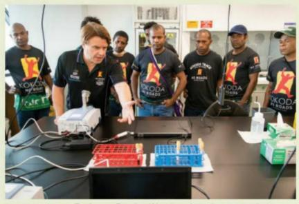
FIGURE 14.2.11 Professor Bayden Wood explains how to analyse blood samples for malaria diagnosis to the Papua New Guinean No Roads to Health team using a portable infrared spectrometer
