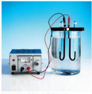
FIGURE 8.1.1 In this electrolysis set-up, electricity passing through a dilute sodium nitrate solution decomposes the water to form hydrogen gas at the left-hand electrode and oxygen gas at the right-hand electrode. The gases are collected in test tubes.
