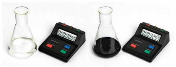
FIGURE 4.3.1 This redox reaction involving colour changes is known as a clock reaction. The black compound is a starch–iodine complex.
