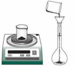
Weigh the pure solid on an electronic balance.
