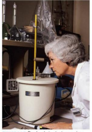
FIGURE 3.3.7 Bomb calorimeter temperature changes being observed by a laboratory technician
