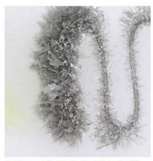
FIGURE 1.1.1 During the electrolysis of tin(II) chloride, distinct metallic crystals are formed at the negative electrode. These can be shown to be tin crystals.
