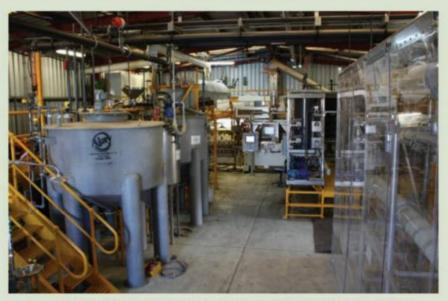
FIGURE 2.4.8 Ethtec trial plant, showing biomass fermentation tanks on the left
