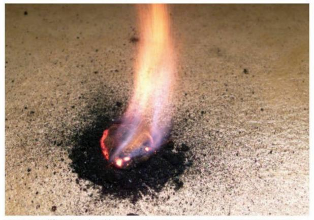
FIGURE 4.1.1 When glycerol is added to potassium permanganate, a vigorous reaction occurs in which the glycerol is oxidised by the potassium permanganate.
