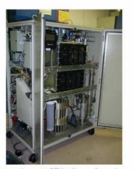
**FIGURE 9.3.4** (a) The conducting polymers in PEM cells are often polymers containing sulfur: polysulfones. (b) A stack of commercial PEM electrolysers.
