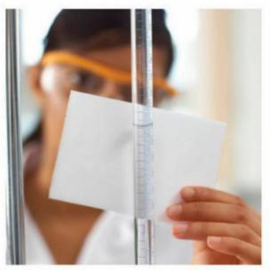
FIGURE 1.3.7 It is important to read the bottom of the meniscus of a solution in a burette at eye level to avoid parallax error.
