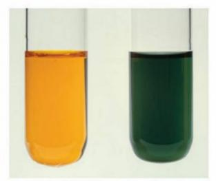
**FIGURE 4.3.3** The yellow-orange colour of dichromate  $(Cr_2O_7^{2-})$  ions changes to the green colour of chromium(III)  $(Cr^{3+})$  ions when it is used to oxidise a colourless reactant, such as ethanol.
