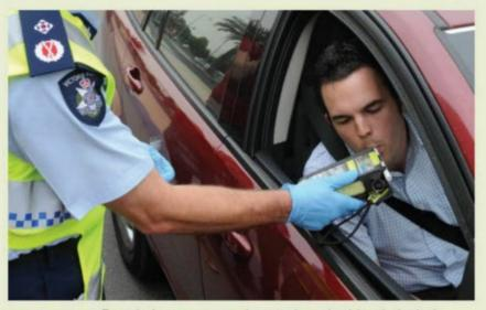
FIGURE 4.3.5 Breathalysers are used to analyse the blood alcohol content of motorists.
