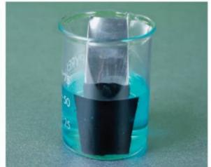
FIGURE 5.1.6 Cu<sup>2+</sup>(aq) ions in copper(II) sulfate solution reacting directly with a strip of zinc metal
