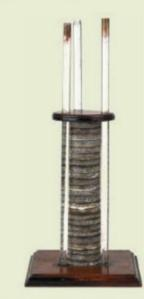
**FIGURE 5.1.2** An original voltaic pile. The pile is 15 cm high and contains alternating copper and zinc discs separated by cardboard.
