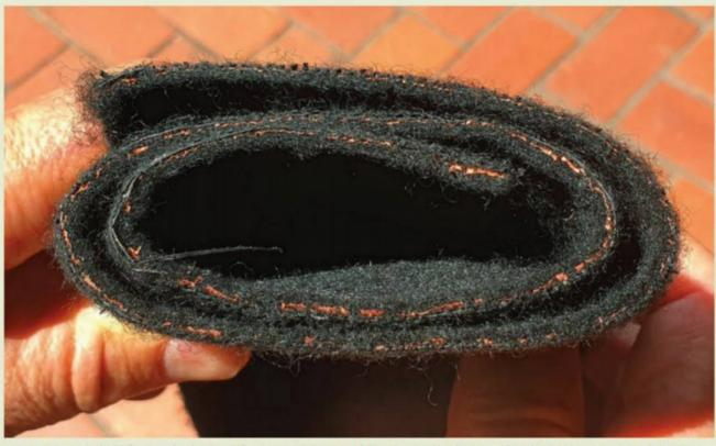
FIGURE 4.1.5 An 18 mm thickness of copper is pressed between two layers of polypropene material in this geocomposite fabric.
