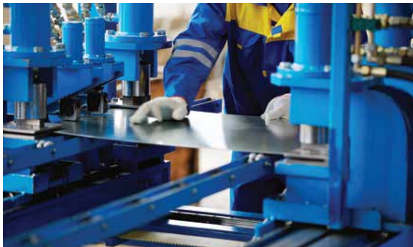
A worker pressing galvanised sheet steel at a steelworks. The zinc prevents the steel from rusting even if the surface is scratched or broken. This is because the more reactive zinc loses electrons, rather than the iron in the steel.
