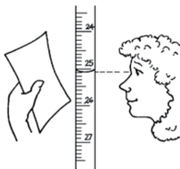
Reading a burette scale
