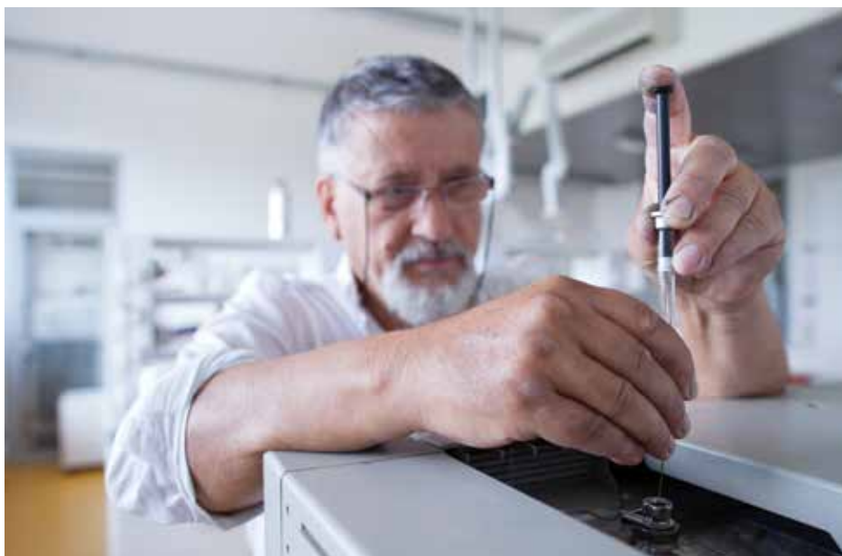
A technician injects a sample into a gas chromatograph. This sensitive instrument can analyse samples as small as one microlitre ( 10^{-6} L).
