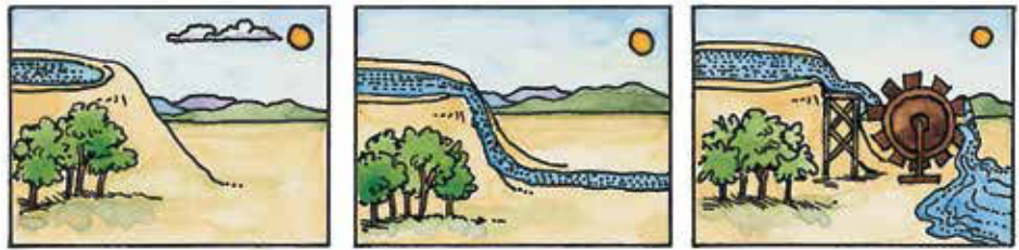
(a) Water stored in a dam has potential energy. (b) Water flows downhill and is converted to kinetic energy. (c) The falling water turns the blades of a waterwheel so that kinetic energy is converted to mechanical energy.
