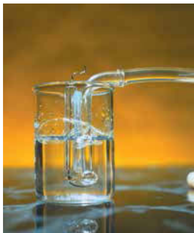
A hydrogen half-cell
