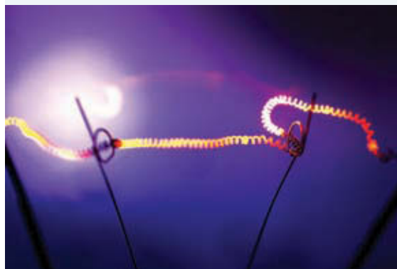
FIGURE 3.9 Tungsten metal filaments used in specialist light bulbs. If hot tungsten is exposed to air, it oxidises to form tungsten oxide. To prevent this, inert argon gas is used to fill the inside of light globes.
