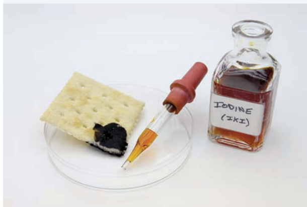
FIGURE 11.24 Iodine can be used as a test for starch. The brown colour of iodine becomes blue/black in the presence of starch.
