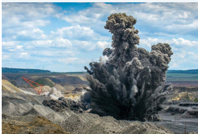
FIGURE 5.1 The explosions used in mining are chemical reactions designed to happen almost instantaneously. They release huge volumes of gases and vast amounts of energy.
