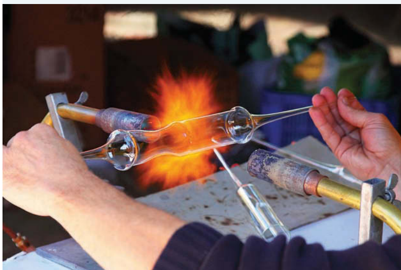
FIGURE 1.38 Making pyrex test tubes requires a very hot flame because glass has a low specific heat capacity of around 0.7 \text{ J g}^{-1} \text{ K}^{-1} .
