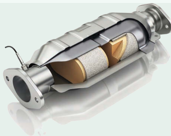
FIGURE 5.12 A typical catalytic converter from the exhaust system of a modern car.
