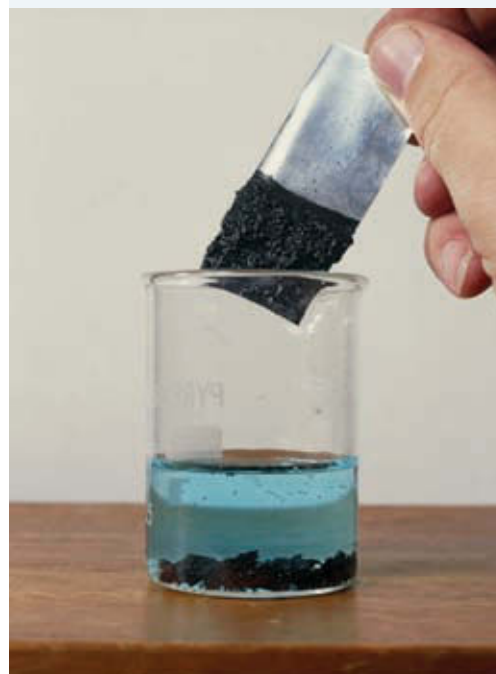
FIGURE 3.14 As Zn reacts with \text{Cu}^{2+} ions, it goes into solution as \text{Zn}^{2+} ions. \text{Cu(s)} is deposited on the surface of the zinc.
