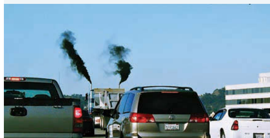
FIGURE 2.11 Black soot exhaust is less common because modern engines and fuels reduce undesired emissions.
