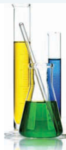
FIGURE 3.8 Different oxidation states of chromium compounds. Left to right: \text{K}_2\text{CrO}_4 , \text{CrCl}_3 , \text{CrCl}_2
