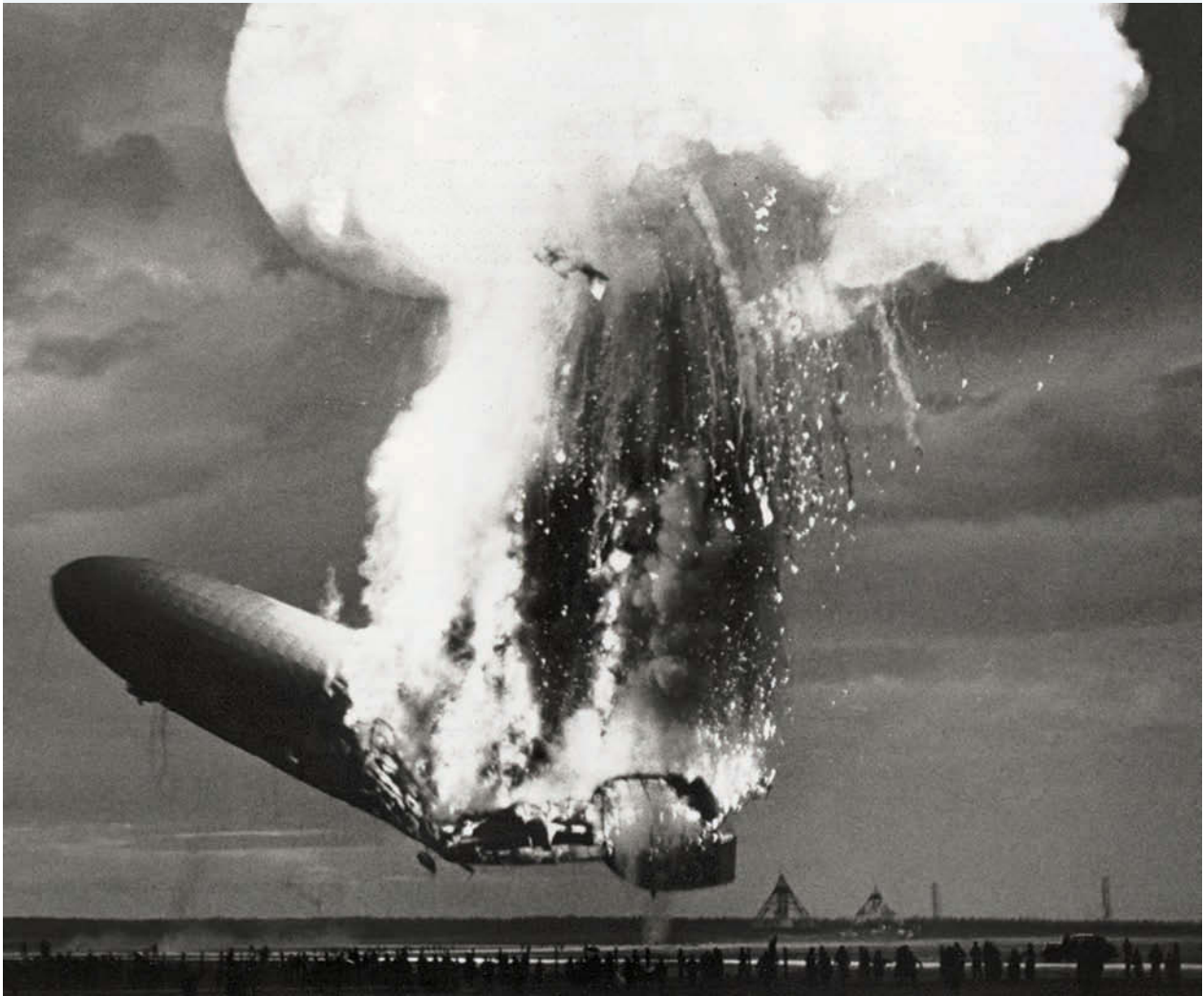
FIGURE 4.10 The Hindenburg airship disaster was caused by leaking hydrogen gas that was ignited by electrostatic discharge.
