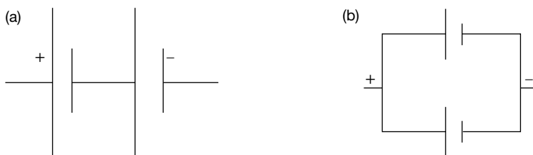
FIGURE 3.23 Arrangement of cells in circuits: (a) Two 1.5 V cells connected in series make a 3.0 V battery and (b) Two 1.5 V cells connected in parallel allow a higher current at 1.5 V.
