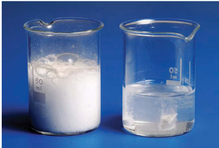
FIGURE 5.8 The higher surface area of the powder (left) results in a higher reaction rate than the solid on the right.
