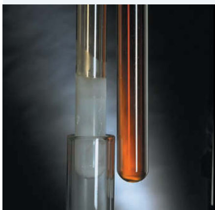
FIGURE 6.12 The equilibrium reaction between brown \text{NO}_2 and colourless \text{N}_2\text{O}_4 is affected by temperature. These tubes initially contained equal amounts of gas; the tube on the left is being cooled.
