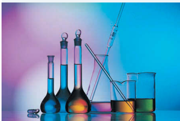
FIGURE 10.22 Volumetric flasks, conical flasks, pipettes, burettes and various beakers are used in volumetric analysis.
