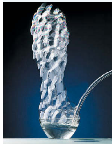
FIGURE 1.36 A mole of hydrogen gas would occupy the same volume as a mole of oxygen molecules, but because hydrogen weighs less than oxygen, it floats upwards in the air.
