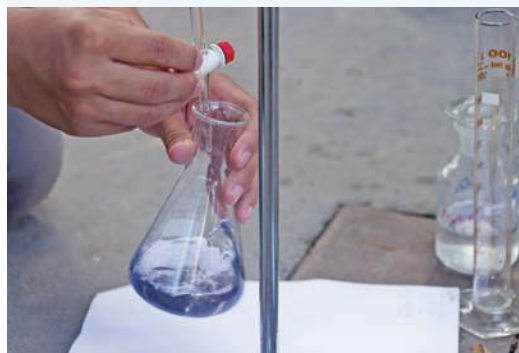
FIGURE 10.27 The presence of a starch-iodine complex indicates the end point of this redox titration.
