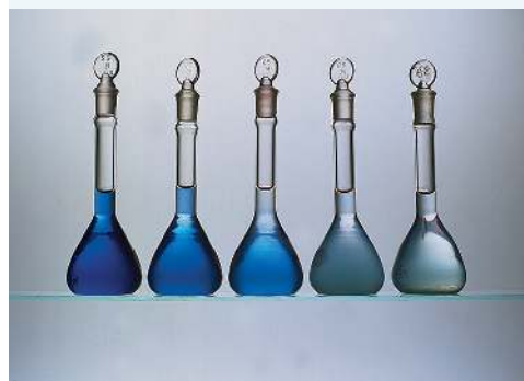
FIGURE 13.2 Solutions with decreasing concentration from left to right. The lightest coloured flask has \frac{1}{16} th of the concentration of the darkest flask.
