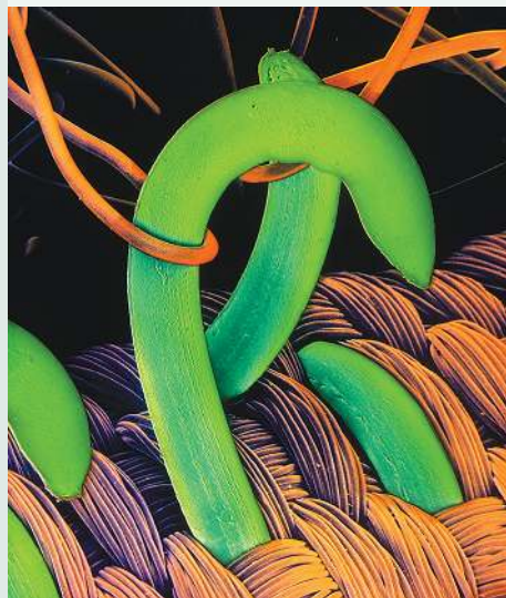
FIGURE 8.10 Electron micrograph of velcro, which is made of nylon. Velcro was inspired by burrs on plants that attach themselves to passing objects through thousands of tiny hooks.
