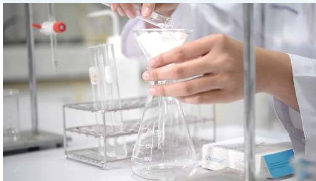
FIGURE 4.22 Filtration apparatus (funnel, filter paper and a conical flask) used to separate precipitate from solution
