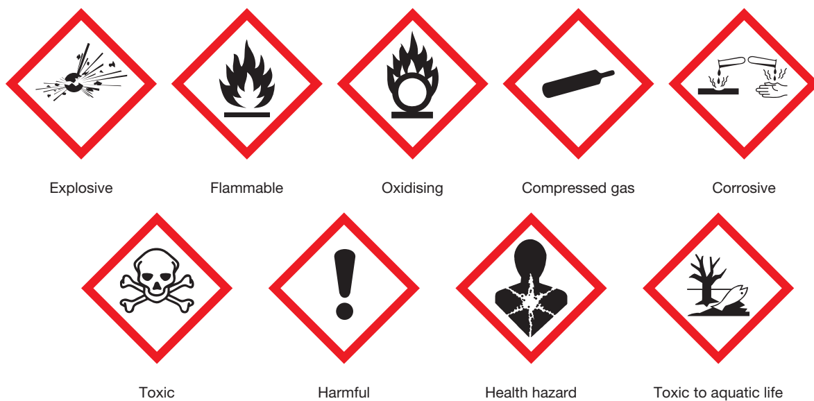
FIGURE 17.35 GHS pictograms can be found throughout risk assessments to visually show any possible hazards.
