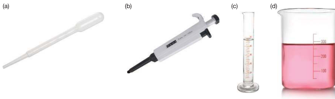
FIGURE 17.24 Equipment used to measure volumes: (a) micropipette, (b) pipette, (c) measuring cylinder and (d) beaker
