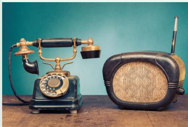
FIGURE 8.15 The casings and dials of early telephones, radios and many other appliances were frequently produced from Bakelite.
