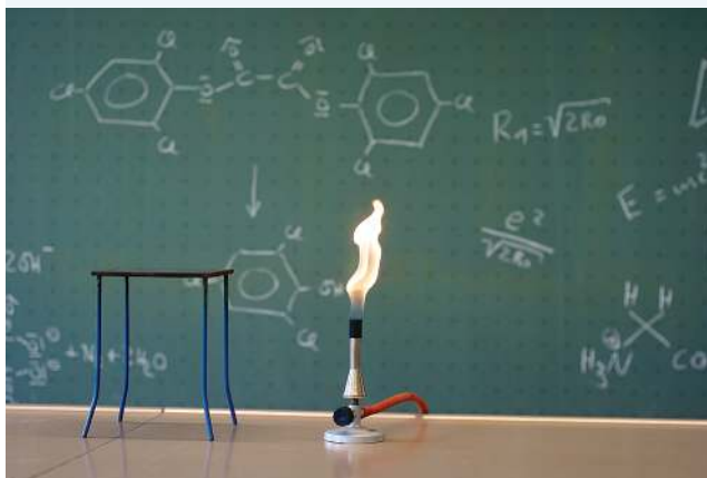
FIGURE 7.10 Methane burning with a limited supply of oxygen produces a yellow flame.
