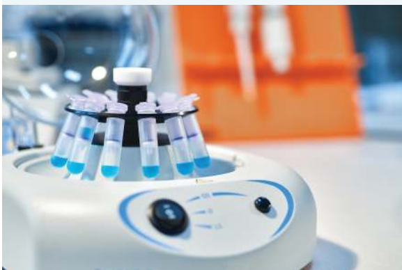
FIGURE 4.21 A centrifuge can be used to make a precipitate settle faster.
