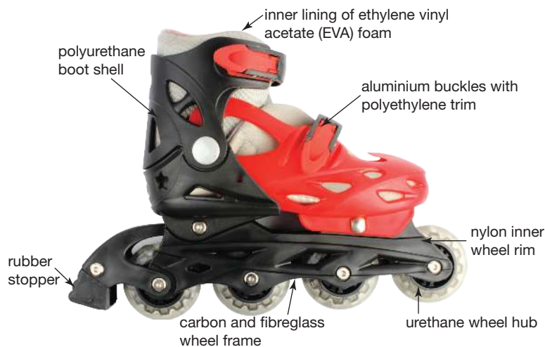
FIGURE 8.24 Many items, such as this in-line skate, are fabricated from a diverse range of plastic components. Each of these is chosen for its particular properties.
