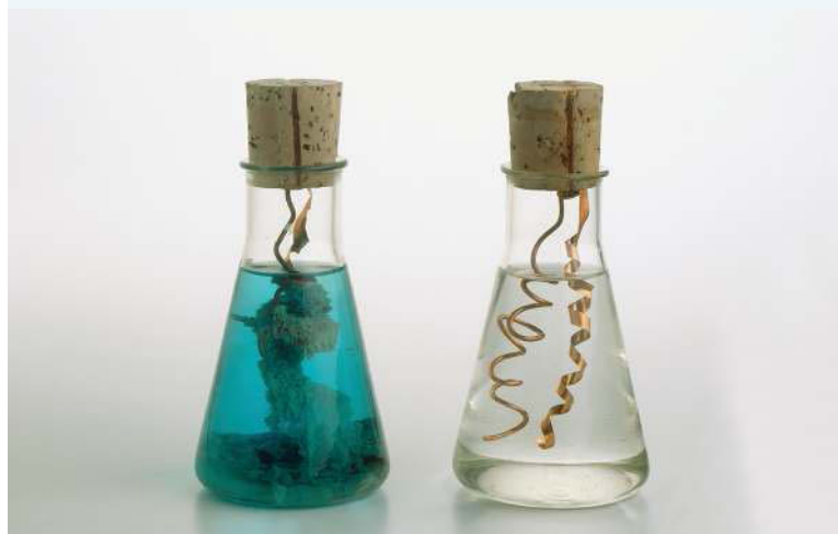
FIGURE 12.8 The flask on the right shows the initial set up. The flask on the left shows the silver forming on the copper strip. The solution has become blue due to the copper ions forming.
