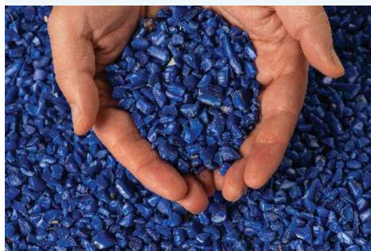
FIGURE 8.27 Recycled polyethene can be made into granules that are then melted and remoulded into new materials.
