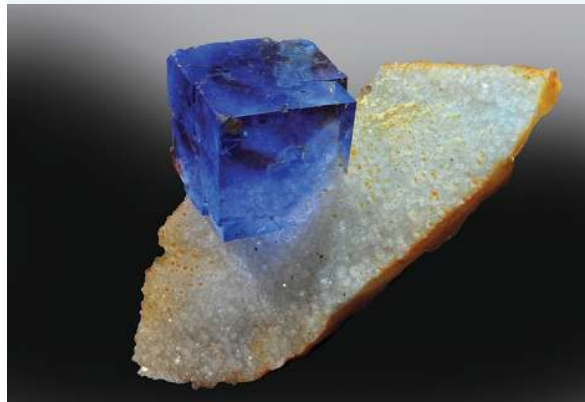
FIGURE 4.2 The main component of the mineral fluorite is the ionic compound calcium fluoride, CaF 2 . Its beautiful crystals are often cubic in shape and appear in a variety of colours.
