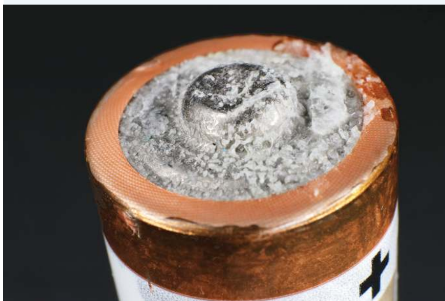
FIGURE 4.10 Old alkaline batteries often leak potassium hydroxide, which reacts with carbon dioxide in the air to form crystals of potassium carbonate. Both potassium hydroxide and potassium carbonate are ionic substances.
