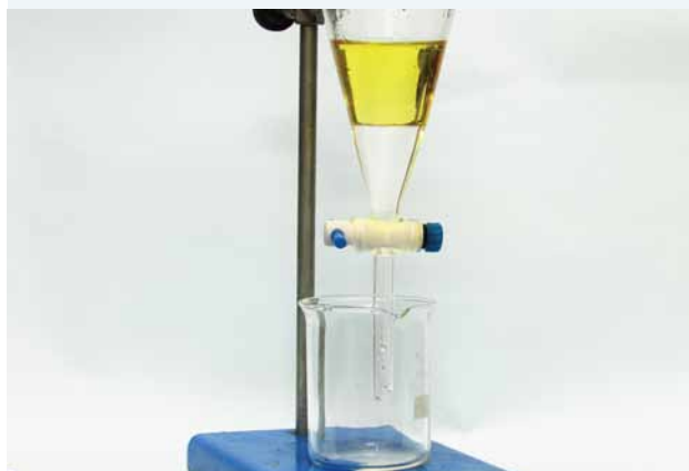
FIGURE 5.4 Oil and water do not mix. The non-polar oil forms a layer on top of the polar water.
