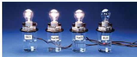
FIGURE 11.12 Strong electrolytes show high conductivity because they produce many ions in solution; water is classified as a non-conductor because it has very few ions.
