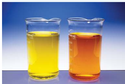
FIGURE 4.16 When chromium reacts with other chemicals, often Cr(III) (chromium in the +3 oxidation state; yellow beaker) changes to Cr(VI) (orange beaker). The colour change can indicate that a reaction has occurred.
