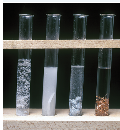
FIGURE 3.11 Reactivity of metals with hydrochloric acid; from left to right: calcium, magnesium, zinc, copper
