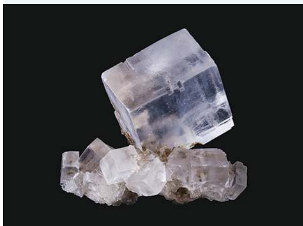
FIGURE 4.6 Each sodium ion is surrounded by six chloride ions, and each chloride ion is surrounded by six sodium ions. This gives the crystals of sodium chloride their characteristic cubic shape.
