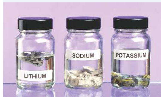
FIGURE 4.14 Lithium (Li), sodium (Na) and potassium (K) are highly reactive and are stored under oil. Lithium has a low density and floats on the oil.
