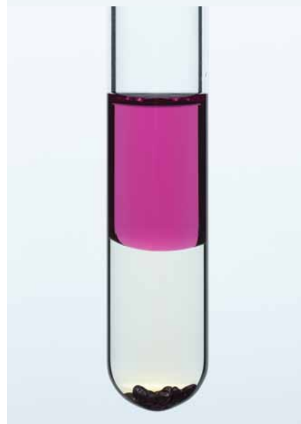
FIGURE 5.5 Non-polar I_2 is soluble in cyclohexane (top) but insoluble in water (bottom).
