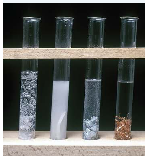
FIGURE 12.11 Reactivity of metals with hydrochloric acid. From left to right: calcium, magnesium, zinc, copper
