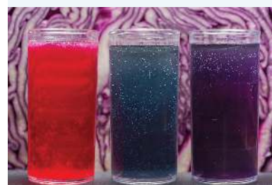
FIGURE 11.1 Red cabbage pH indicator solution: acidic lemon juice (red), alkali sodium bicarbonate (blue) and neutral water (purple)
