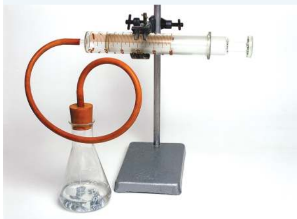
FIGURE 11.27 Measuring the volume of gas produced during a reaction between an acid and zinc
