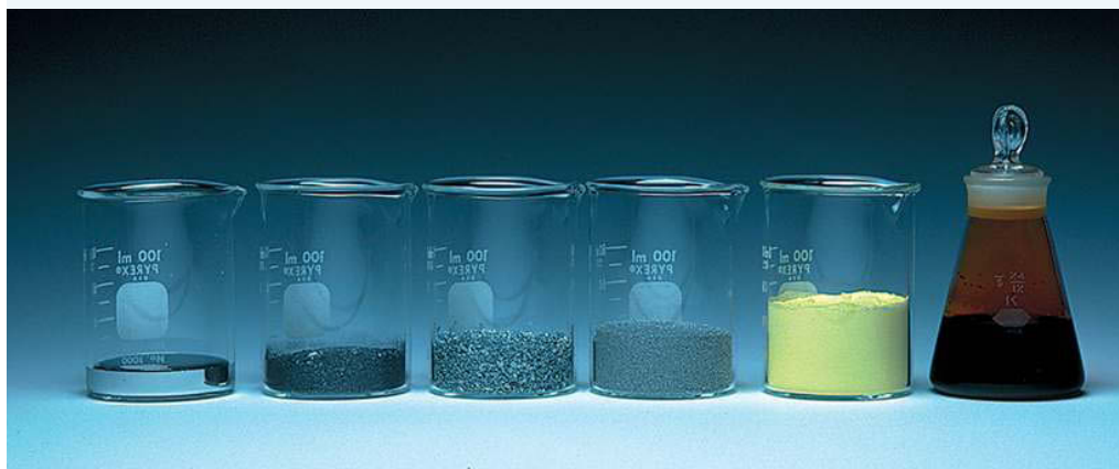
FIGURE 6.9 One mole each of mercury, zinc, silicon, aluminium, sulfur and bromine. The quantity of each of the substances shown contains 6.02 \times 10^{23} particles.
