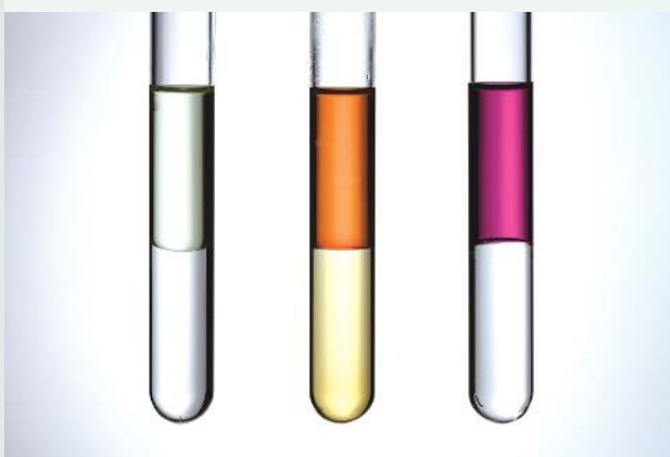
FIGURE 13.17 Halogens ( Cl_2 , Br_2 , I_2 ) dissolved in non-polar cyclohexane (top of each test tube), demonstrating immiscibility with water (bottom of each test tube)
