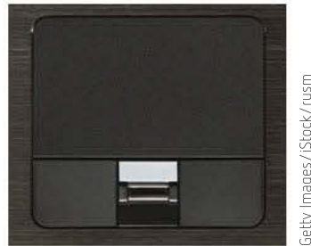
FIGURE 3.32 The fingerprint scanner positioned directly below the trackpad (in-built mouse replacement) on a laptop computer. The user only need run their fingerprint over the brown stripe in the gold section to capture their fingerprint scan.
