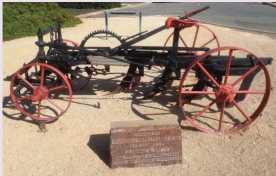
Figure 4.14: An early stump-jump plough invented by R.B. Smith of South Australia in 1876. This implement was especially useful in mallee country.
