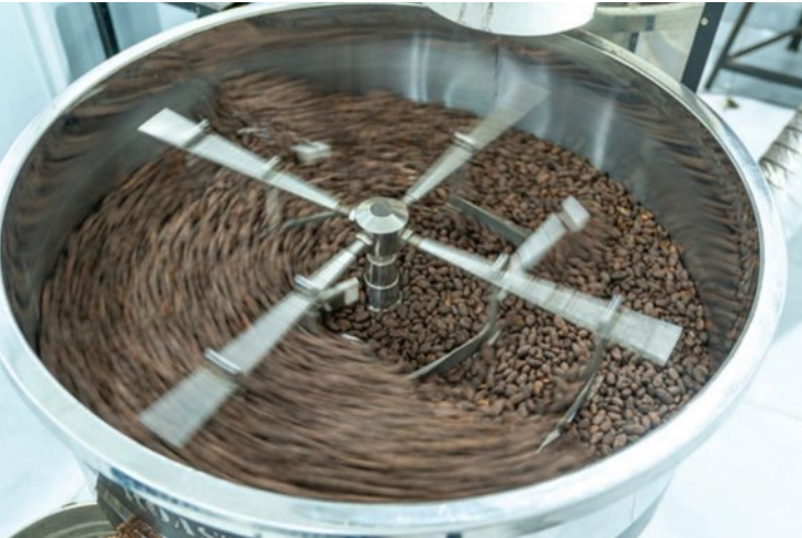
Figure 3.8: Roasting cacao beans is part of the chocolate manufacturing process. Over time, the development of technology has allowed for food processing techniques, such as roasting, to be more efficient. This has enabled food manufacturers to produce food commodities in large quantities, in a shorter timeframe.
