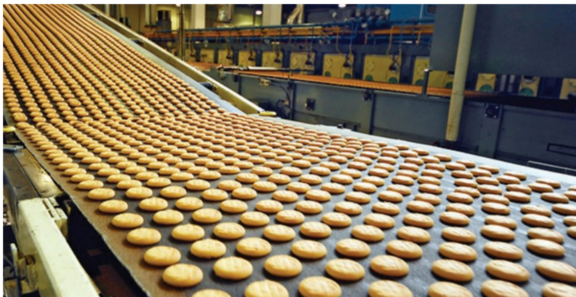
Figure 6.28: Specialised equipment and machinery enable biscuits to be produced at a rapid rate, all uniform in colour, shape and size.
