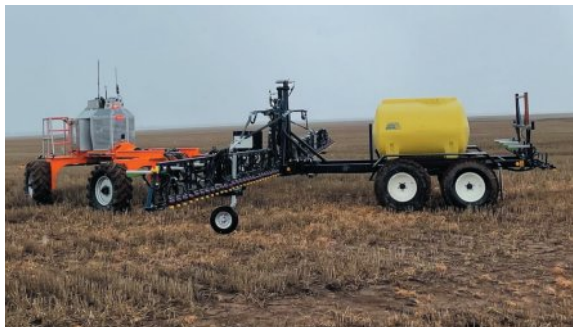
Agricultural robots can be fitted with a herbicide tank and spray arm to spray and eradicate individual weeds.
