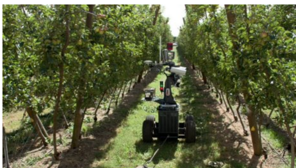
Robots are designed to sense flowers and fruit on trees, and are able to determine if fruit can be harvested.
