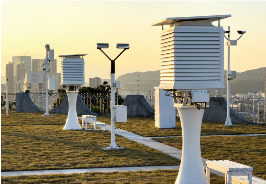
A modern weather station measures atmospheric conditions, such as temperature, atmospheric pressure, humidity, wind speed, wind direction and precipitation amounts, to provide information for weather forecasts and to study the weather and climate.
