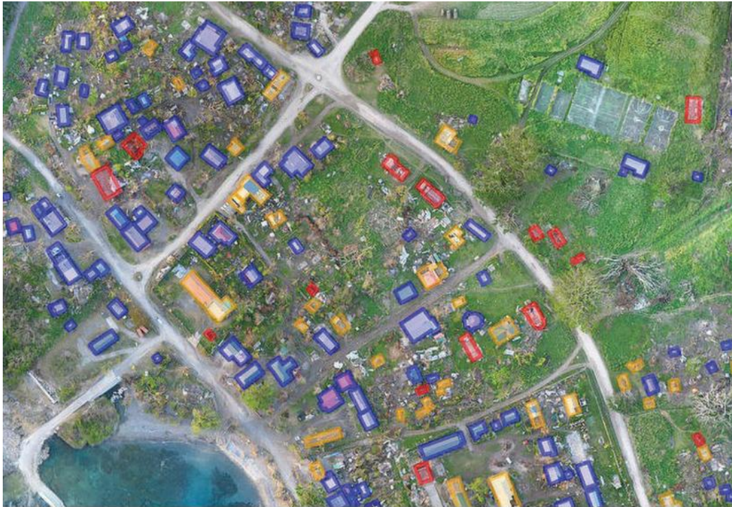
▲ Figure 2.28 Map of Cyclone Pam damage, Vanuatu, 2015. Red structures are heavily damaged, blue structures moderately damaged and yellow structures undamaged
