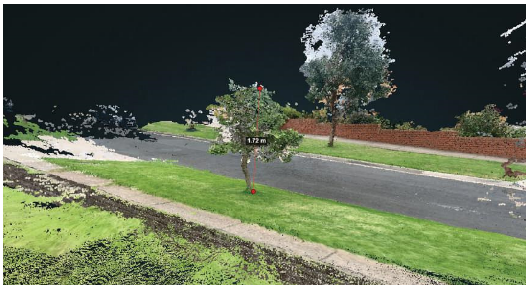
▲ Figure 5.15 Photogrammetry as a remote sensing tool: A geo-referenced point cloud is generated from a brief video pan; the resulting 3D file is accurate enough to take measurements from on the computer. This file can be converted to use with AR goggles (Image created using KickTheMap app)
