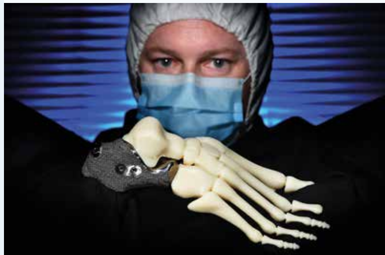
FIGURE 11.18 Anatomics biomedical technician Stuart Hall with a prototype heel of the revolutionary implant used to save Len's leg.
