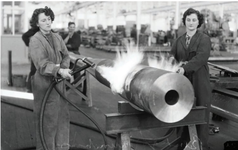
↑ Source 4.9 Two women working in an armaments factory in Bendigo in April 1943. They are superheating the barrel of an anti-aircraft gun in preparation for its final straightening.
