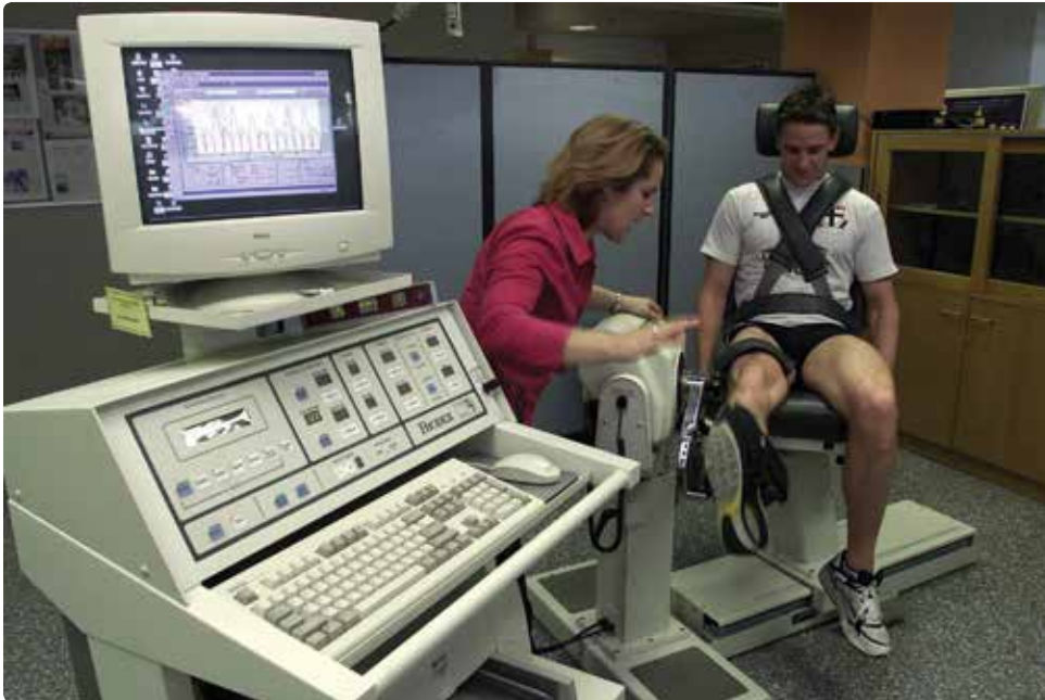
FIGURE 3.17 A Biodex machine allows the quadriceps muscle group to be both assessed and trained through its full range of motion.
