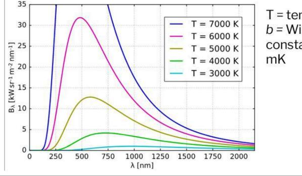
T = temperature (K) b = Wien's displacement constant = 2.897772 x 10<sup>-3</sup> mK
