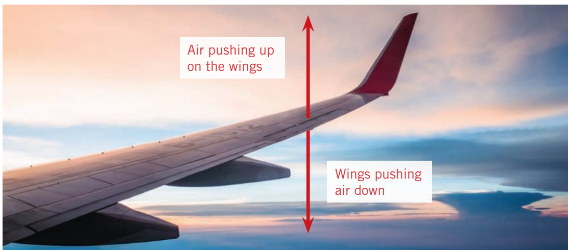
Figure 8B–6 The wing of an aircraft is designed to push air down; the air then pushes back up on the aircraft, providing the lift.
