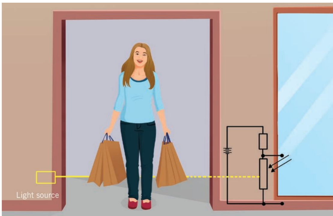
Figure 6A-17 A very common LDR use is to trigger a buzzer or alarm when a person entering a doorway breaks a beam of light. When the LDR is in shadow, its resistance increases, so the potential difference across it increases, which can trigger a switch which turns on a buzzer.
