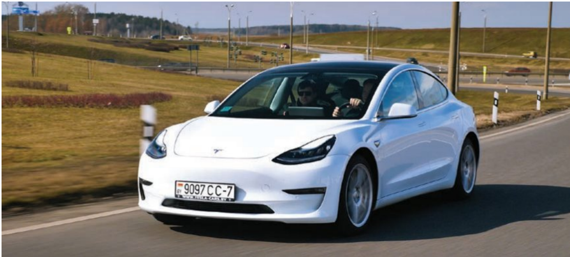
Figure 5B–7 The Tesla Model 3 has a battery pack under the floor and direct drive electric motors. The low centre of mass contributes to stability, especially when cornering.
