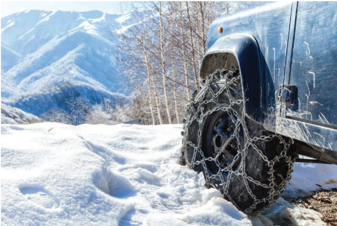
Figure 7A–3 The chains on a car’s tyre increase the friction between the wheels and the icy road so that forward motion of the car can be generated.
