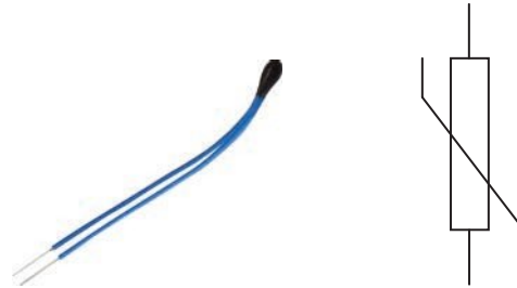
Figure 6A-18 Left: A bead-type thermistor; its resistance changes with temperature. Right: Thermistor symbol
