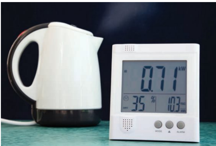
Figure 5E–3 A wireless energy monitor linked to the electricity meter can display a home’s present electric power use, 0.71 kW in this case, equivalent to 710 joules per second.
