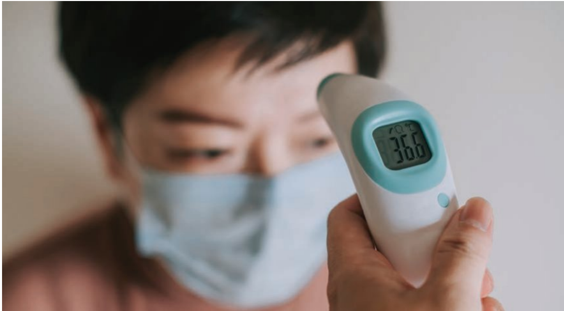
Figure 2B–3 Measuring forehead temperature by measuring the intensity of infra-red radiation emission and converting using Wien's law.
