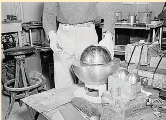
Figure 4A–12 Recreation of the Slotin experiment. Two half-spheres of beryllium (a neutron reflector) are placed around a spherical plutonium-239 core.
