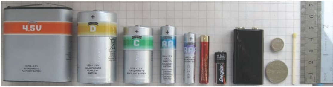
Figure 5B–6 Batteries supply different amounts of electrical energy. For household use a potential difference of 1.5 V up to 6 or 12 V is sufficient. The battery that drives an electric vehicle is between 300 and 500 V, with energy storage capacity of 150–400 kWh.
