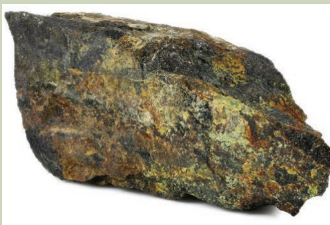
Figure 4C–1 Uranium ore, such as this sample from an Australian mine, normally contains the isotopes uranium-235 and uranium-238 in the ratio of 1:140.
