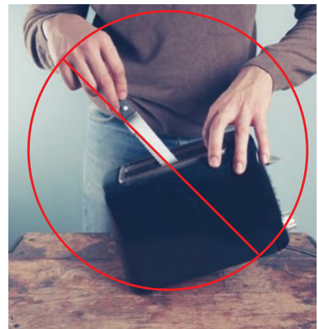
Figure 6C-5 Using a knife to free toast that is stuck can easily dislodge heater wires, which can then connect the active with the case of the toaster. Current enters the body where it comes in contact with the supply, and flows through the lowest resistance path to earth. Don't let that be through your body!
