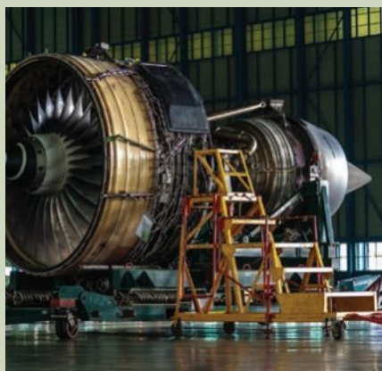
Figure 8B–1 A turbofan jet engine with the cover removed (left) and a diagram of a turbofan jet engine (right)
