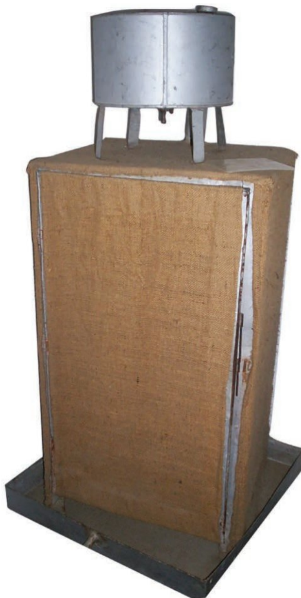
Figure 2A–10 A Coolgardie safe is a box that keeps its contents cool through evaporative cooling. Water in the tank on top is allowed to drip onto the hessian sackcloth covering the safe, from where it diffuses by capillary action through the cloth and evaporates, taking away heat and so cooling the safe.
