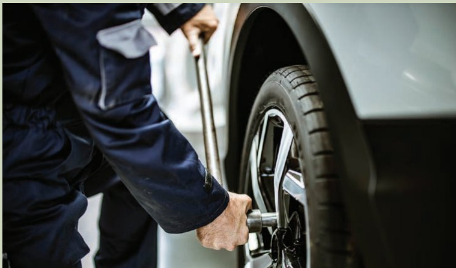
Figure 8C–1 Using the long lever on a socket wrench to loosen the wheel nuts on a car
