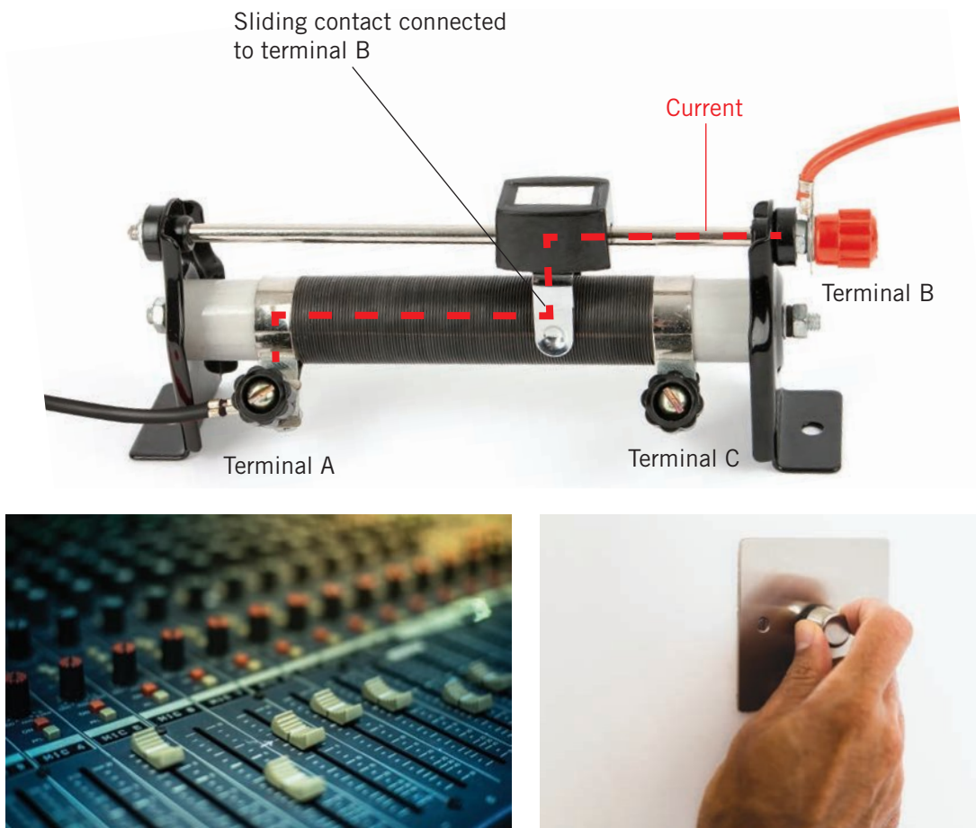
Figure 6A–9 Top: A physics laboratory potentiometer with terminal A connected to a power source and current flowing from there through the coils to the sliding contact and out through terminal B. This is the same connection as in Figure 6A–13 when it is used as a rheostat. Sliders controlling sound levels (bottom left), and a rotating knob dimmer switch (bottom right) use potentiometers to control the current of the circuit. The high-resistance wire may be straight, as in the slider type, or curved into an almost complete circle, like the rotating-knob type.
