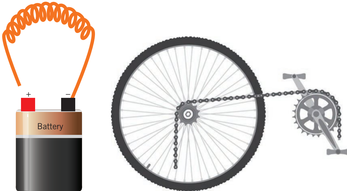
Figure 5A-11 An open circuit (left) is as though the bicycle chain broke and came apart (right), so the links (electrons) can no longer move around the circuit.
