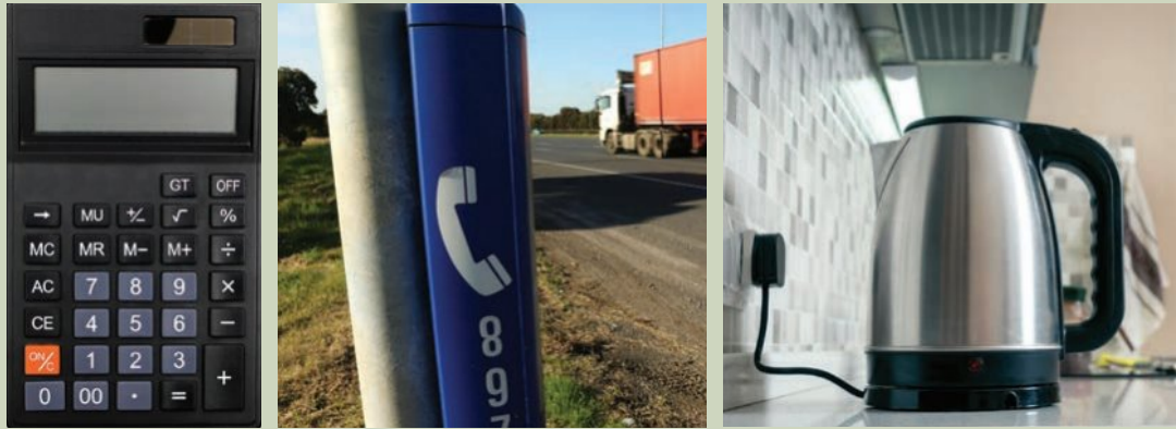
Figure 5E-2 Devices that use small amounts of energy per second ('power'), such as a calculator with a built-in solar panel (left) and an emergency roadside phone (centre), can often be supplied from solar panels. Appliances that use greater power, such as an electric kettle (right), need a connection to the mains electricity.
