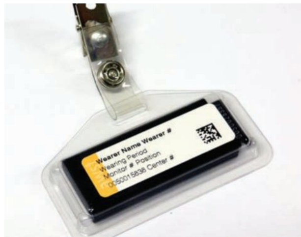
Figure 3E-10 An OSL monitor is used by radiation workers for monitoring personal levels of radioactivity. workers for monitoring personal levels of radioactivity. The source needs to be clearly labelled and identified, the amount of radioactive material specified, its half-life and activity known and/or determined, as well as the type(s) of radiation it is emitting.
