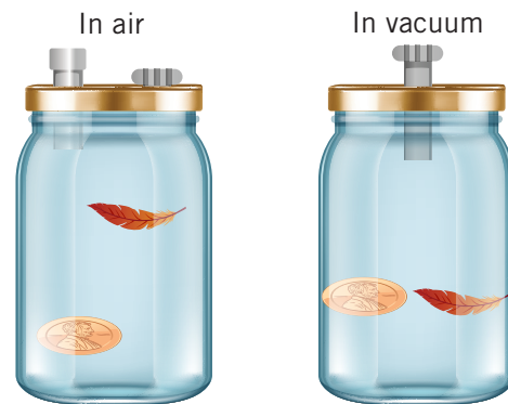
Figure 3A–15 Removing the effect of air resistance shows that a coin and feather both accelerate at a rate of 9.8 \text{ m s}^{-2} .
