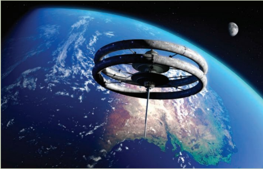
Figure 1B-2 In the future, spacecraft might use a spinning donut shape to produce artificial gravity.
