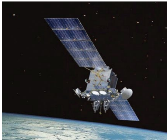
Figure 3C-6 A modern communications satellite that uses solar energy to power its batteries and run its electronic systems
