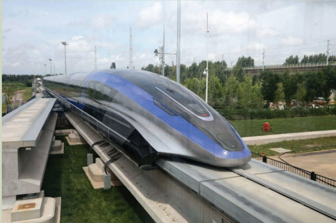
Figure 4B–1 China’s new experimental maglev bullet train, which can travel at 600 \text{ km h}^{-1} on a magnetic ‘cushion’
