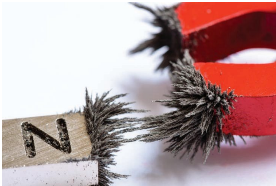
Figure 4B–5 The three-dimensional nature of magnetic field lines can be seen when iron filings are gathered between the north pole of a bar magnet and the south pole of a horseshoe magnet.
