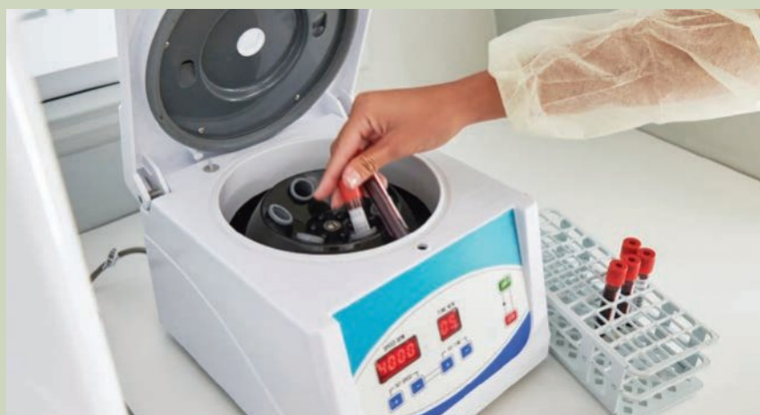
Figure 1B–1 The centrifuge above is being used to analyse blood tests. The specimen tubes are placed in holders that position the tubes at an angle to the axis of spin, or even at 90° to it, with the top closer to the axis and the bottom further away. During centrifugation, the denser red blood cells settle at the bottom of the tube, while the less dense plasma rises to the top.
