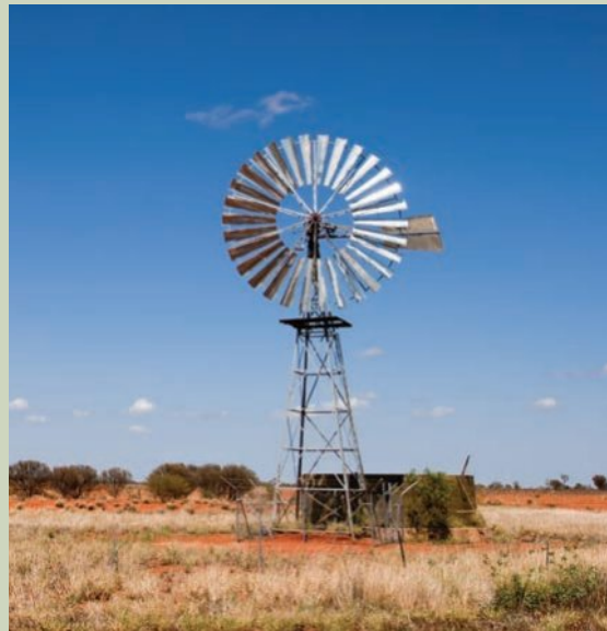
Figure 5D–1 In Australia, the outback windmill lifting bore water to the surface is a common sight. This one is purely mechanical, but there are also windmills that drive a generator instead of a pump to supply DC power to remote homes and stations.
