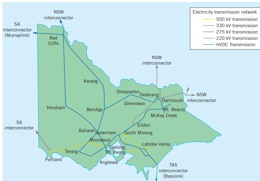
Figure 6C–6 A map of Victoria's electricity grid, showing transmission lines of different voltages, with interconnectors to South Australia, New South Wales and Tasmania. These connections between states help to balance power demand with availability. This is becoming even more important with the growth in renewable sources of energy and storage.
