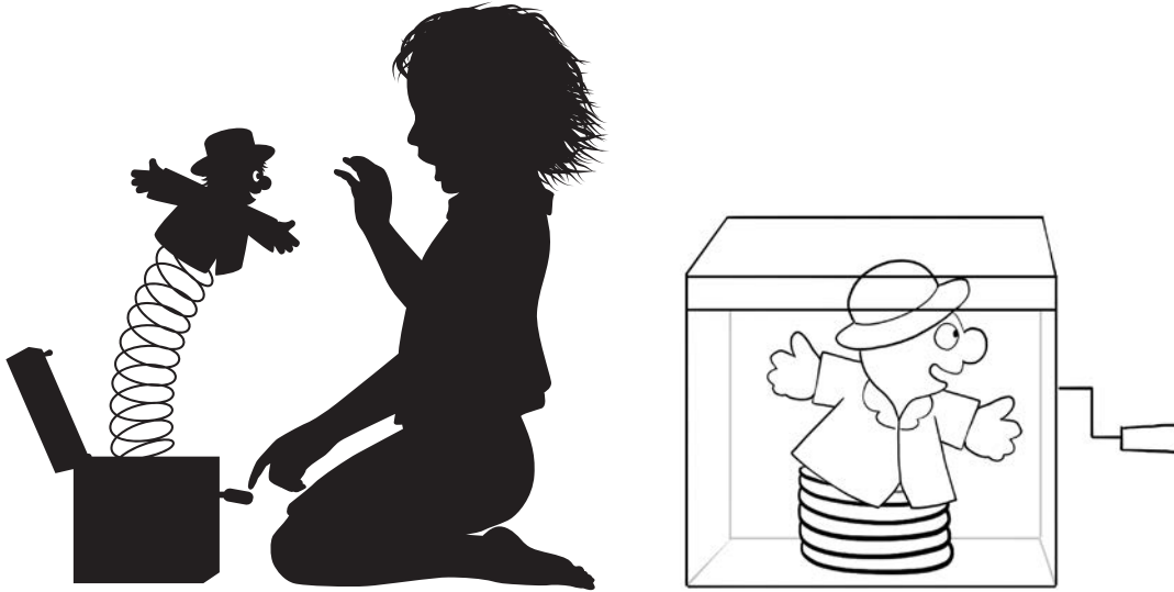
Figure 9D-2 A jack-in-the-box can illustrate an example of the conversion of mass and energy. When the box is closed, the spring is compressed (right). The compressed spring has elastic potential energy and this stored energy manifests itself as a tiny increase in mass.
