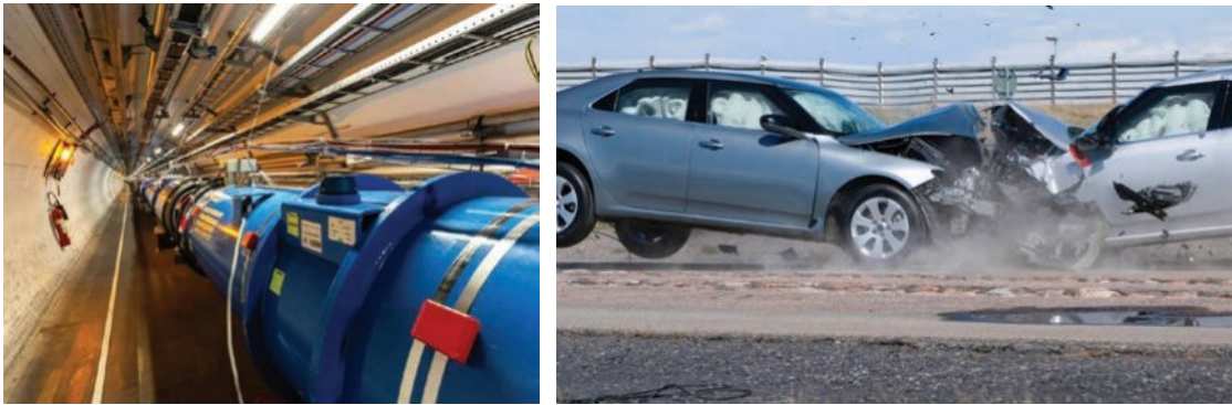
Figure 2A-4 Left: The 27 km long Large Hadron Collider, located on the Swiss–French border, collides beams of protons into each other at close to the speed of light in a highly evacuated vacuum chamber. These subatomic collisions are considered to be elastic, and the system is assumed to be a closed one. Right: A car crash is a common inelastic collision that you will study in Unit 3 Physics.
