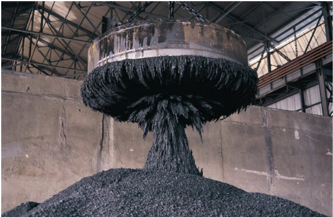
Figure 4B–16 500 kg of hot metal chips are transported into an industrial furnace by an electromagnet. The furnace then creates cast metal for wind turbines.
