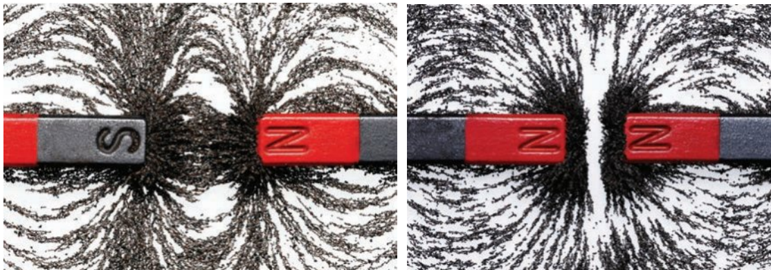
Figure 4B–6 Magnetic field lines shown by iron filings for attraction: north–south magnets (left) and repulsion: north–north magnets (right)
