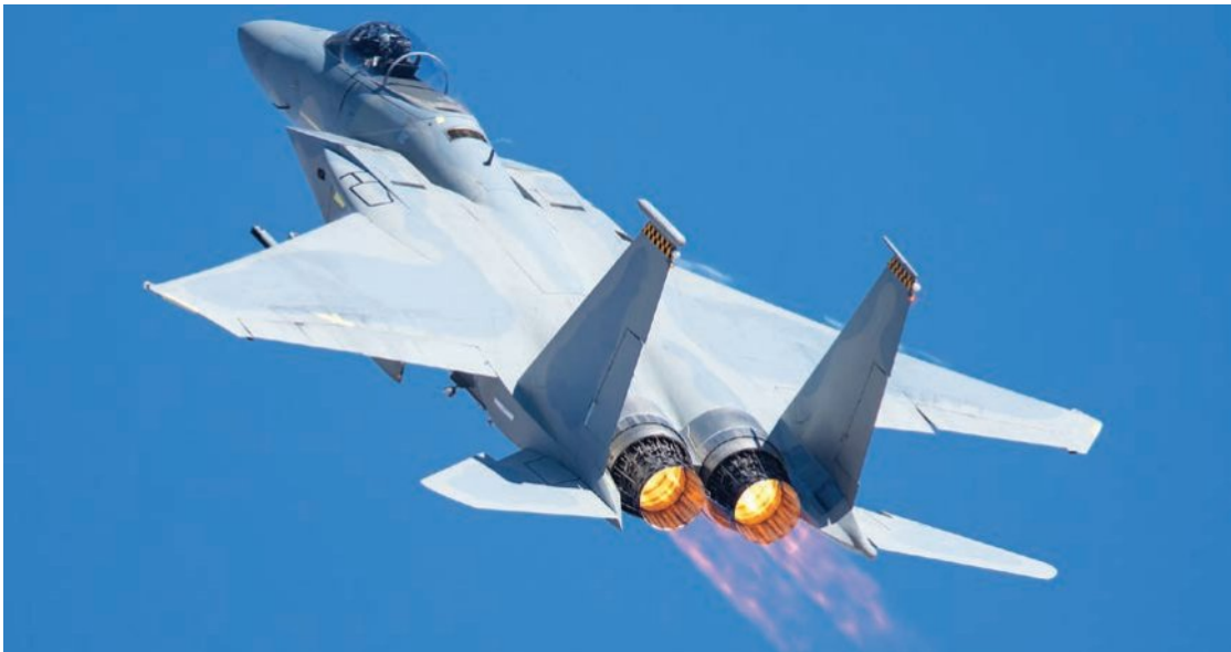
Figure 1A–5 The jets of a fighter jet push out extremely hot gas; the gas pushes back on the fighter jet and accelerates it forwards.
