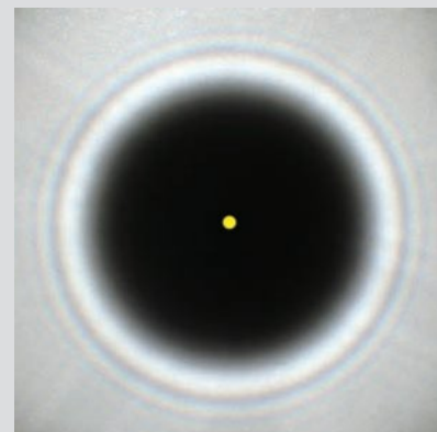
Figure 7A–21 The Poisson spot appearing at the centre of a shadow formed by a circular object
