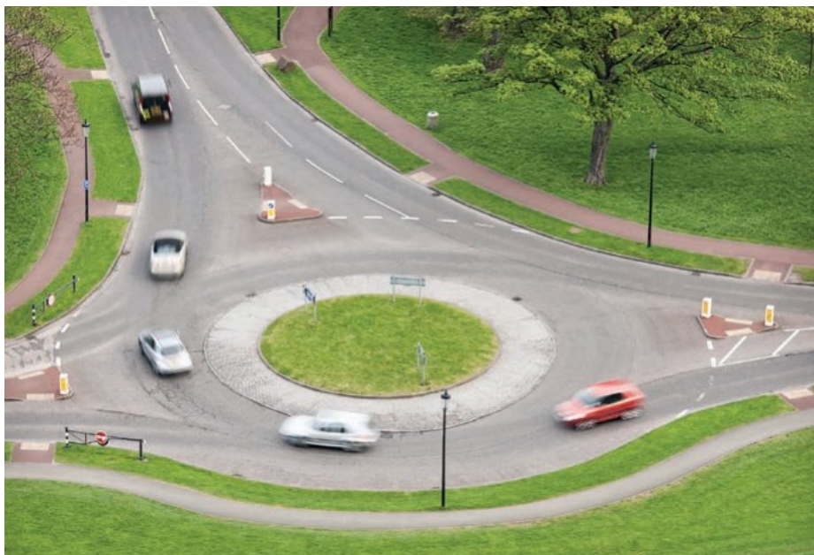
Figure 1B–4 When cars turn around a corner that is on level ground, a component of the friction between the tyres and the road provides the centripetal force.
