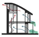
Figure 5 Natural convection creating air movement to cool a house
